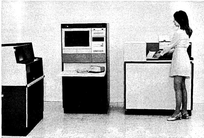
Configured as a communications terminal, the Mohawk Data SYSTEM 2400 can convert a tape that wasn't originally intended for communications, and then transmit it in a compressed, control-coded format.
