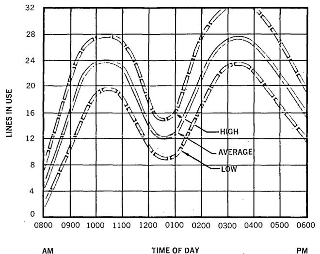
Fig. 6. Usage pattern by time of TRW in-house system.
