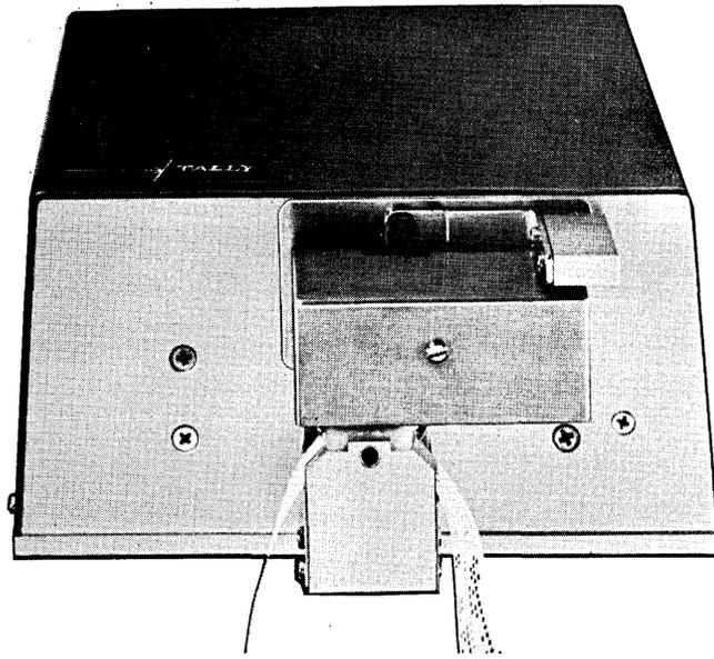
You don't have to upset your present paper tape data preparation routine to take advantage of a high speed data communications system. The low cost, easy to use, Tally data terminal shown above transmits paper tape data over the ordinary dial-up telephone network at 72 characters per second.
