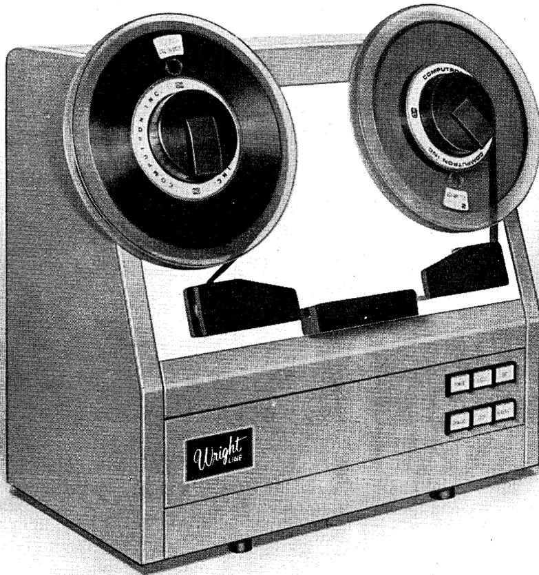
**NEW TAPE CLEANER** removes loose oxide, dust and other contaminants from magnetic tape. Contaminants are shaken loose by sixty cycle per second pulsing vacuum vibration and are carried away from the tape by a powerful vacuum. Exclusive Vac-U-Torq drive assures proper tape tension at all times and eliminates danger of spilling tape. Complete dual pass cleaning on 2400 ft. reel takes less than four minutes.
