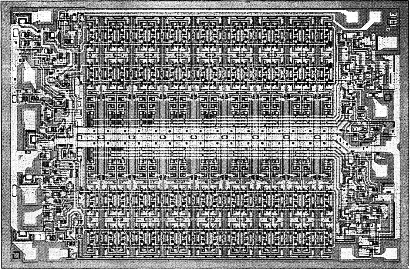
**Introducing the Intel Schottky Process Model 3101 Bipolar Scratch Pad Memory.** 64 bits—16 x 4/fully decoded /50 nanoseconds access time/OR-tie capability/simple memory expansion through chip select input/6 milliwatts per bit power dissipation/16 lead D.I.P.
