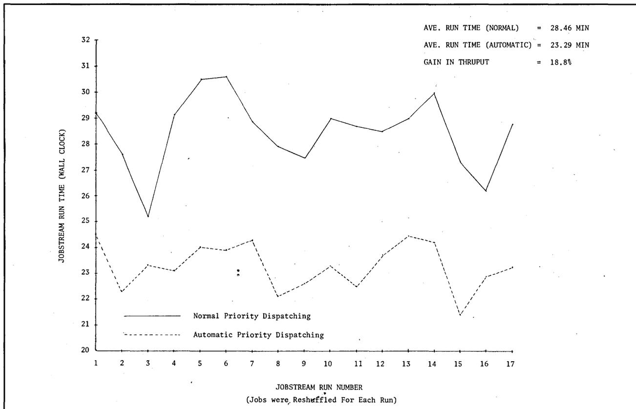
Fig. 1 Automatic Priority Dispatching (without time slice option).
