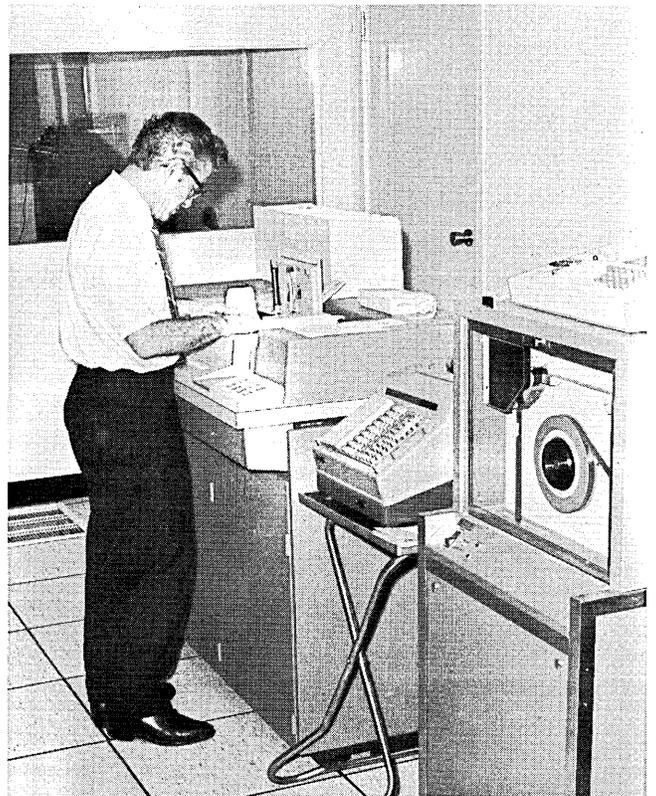
Inputs to the system are in the form of punched cards, Mohawk key-to-tape unit records, journal tapes which are recorded on NCR optical font adding machines for conversion (as above) to mag tape, and audio transmissions.
