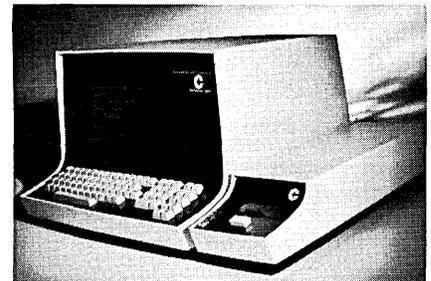
standard 64-character set and can include an extra 10 numerics. In addition to recording and editing displayed data from this keyboard, a "reproduce-local" mode may be used to scan the contents of the tape cassette at 60 cps (scrolling forward or backward), and a "reproduce-remote" mode is used for sending to a cpu or for file retrieval by the cpu.
