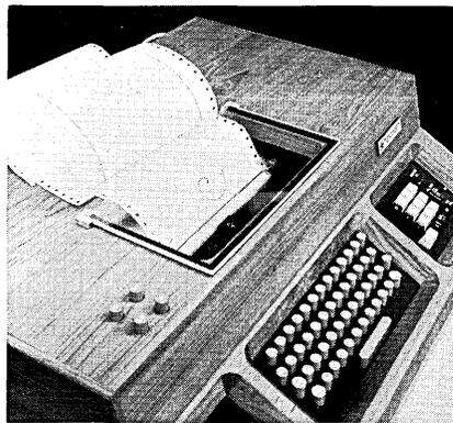
and knows some tricks that no one ever tried to teach a teleprinter. One of the most obvious differences—and actually one of the most minor—is that the standard tty keyboard has been augmented with a small numeric key set placed on the right side. The paper
