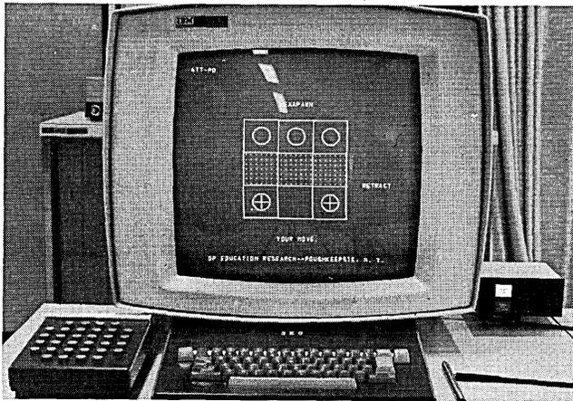
Fig. 5 Display of RETRACT after first half of move by player.
