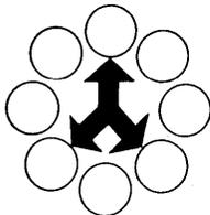
Actually, during that short time the computer works on many jobs. It does a fraction of a second's work on job A, then on job B, and so on until every active terminal has been serviced. It repeats that cycle over and over until all jobs are complete.
