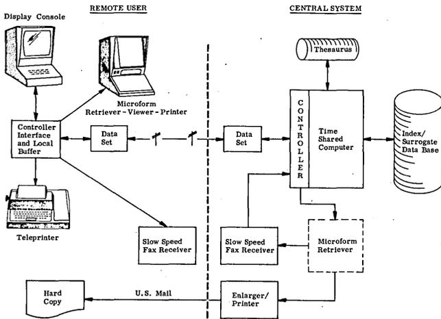
Fig. 2. Remote User/System Communication
