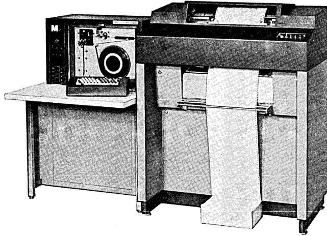
**LINE PRINT-OUT FROM 7-CHANNEL MAGNETIC TAPE UNIT**—1250 lpm:160 character line. Printer connects directly to a 729 . . . or MDS 2207 Mag Tape Unit. (MOHAWK 7160 OFF-LINE PRINTER.)
