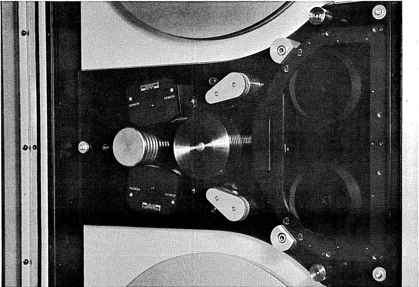
DUAL INERTIA DRIVE, INERTIA DISENGAGED
