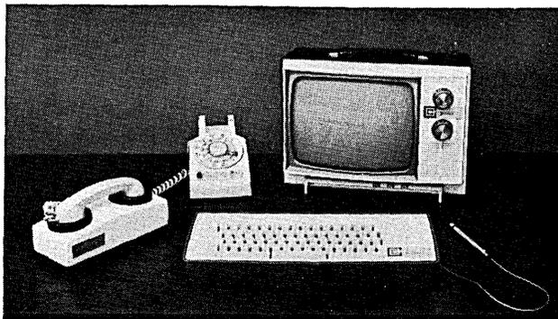
The CC-30 Display Console Using CRT Receiver.
