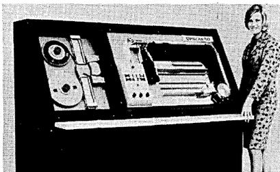
computer-printed, machine-printed, hand-marked, punched, or bar-coded forms, and can read data on 1" x 3" forms at a speed of 24,000 an hour. The OpScan 50 can read BCD or positional codes, such as pencil marks and punched codes, and has a basic tape speed of 24"/second. The integral tape deck adapts to 200, 556 and 800 characters an inch. A special blocking form allows five forms per tape record. OPTICAL SCANNING CORP., Newton, Pa. For information:
