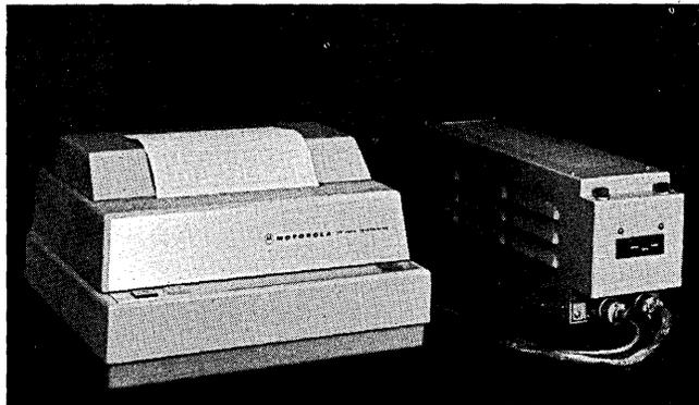
The Motorola TP4000 Teleprinter.
