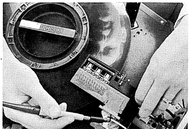
throughout the logic, arithmetic and several functional areas. This single circuit is combined on a total of only 16 wiring boards for memory and logic operations.
