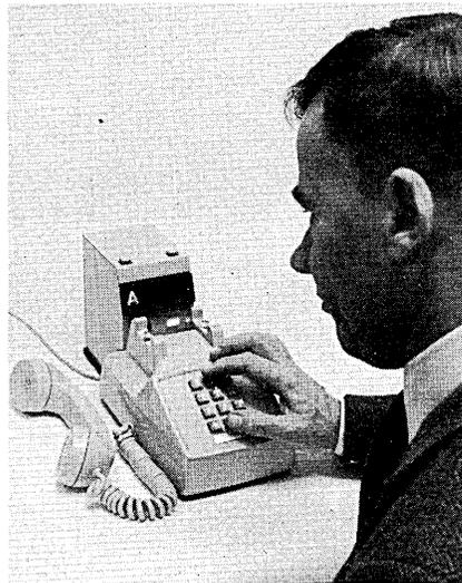
sentence signals. The 2 button, for example, is used to produce A, B, or C—depending on whether it is depressed one, two, or three times. The signals are stored until a character is fully coded, then released by pressing the zero. Practical limits of output are 8 to 16 words per minute. Further experimentation, including the use of simple printing attachments, is under way.
