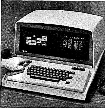
ters each; displays of 200 and 512 characters are also available as standard models. The character repertoire includes 26 alpha, 10 digits and six punctuation marks, plus a flashing cursor for character and line indication; data can be added, changed or deleted by the operator. The system uses an 8-bit code. TRANSISTOR ELECTRONICS CORP., Minneapolis, Minn. For information:
