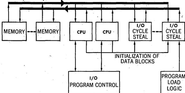
central processing units (CPU's) (1 to 3) to provide a multimission capability. The input/output (I/O) provisions are also modular to adapt the basic computer to a large variety of experiments and spacecraft. The memory modules are woven, plated wire, random accessed, and true non-destructive readout. Each module will provide 8,192 18-bit words of storage with a 2 microsecond cycle time.
