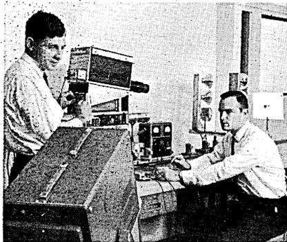
Jerrold J. Deener, detects and locates real or photographed objects in white light using standard hardware and optical techniques. Polarized aperture masks, a polarized grating, and a vidicon detector are used and the output of the vidicon is monitored by television and oscilloscope.
