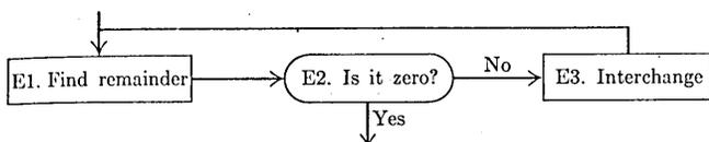
Fig. 1. Flow chart for Algorithm E.
