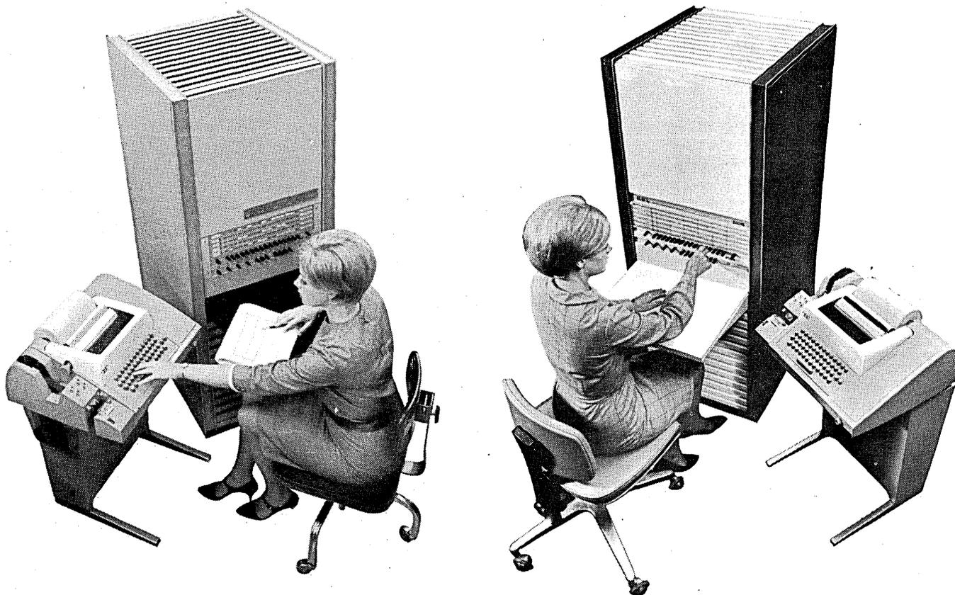
Over 50 SEL 810A, 16-bit computers have been supplied for data acquisition and control. Now meet the SEL 810B, with twice the speed of the A. Yet only about 20% more in price. Same great features: all integrated circuits, 2 levels of priority interrupt, memory expandable to 32K, I/O typewriter, high-speed hardware multiply and divide, and real-time I/O structure. And the software package of the 810B has been proven in the A.
