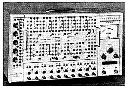
top model that is expandable up to 10 amplifiers and 15 coefficient potentiometers. The unit has ±100 V design, REP-OP mode control, and a null reference system.
