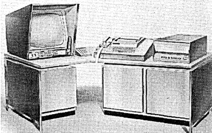
random access memory. Input devices include light pen, A/N keyboard and function keys. Output is on a rectangular 21" CRT screen.
