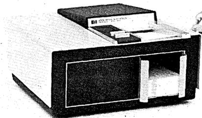
information. The unit, model 2760A, plugs into a standard telephone data set, and can be used in simple data communications applications. It operates in temperatures from 0° - 55°C and 95% humidity at 45°C. MTBF is 2000 hours at 25°C. A prototype of this model was displayed by the Datamec Corp. over a year ago, but did not perform to the company's satisfaction; now improved, it is being reintroduced.
