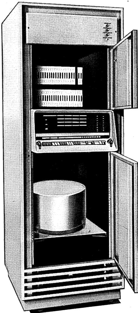
The versatile new PDP-8/S Digital Computer costs about \$10,000, complete with 4,096-word core memory. By investing \$9,950 more, any PDP-8/S (or PDP-8) user can make his computer think on a 32-times bigger scale. How? By plugging in a VRC 1104-8/S Drum Memory System . . . thus adding 131,072 additional words of data base or program storage . . . and enabling drum-stored programs to be called out as sub-routines, page by page or in up to 7-page groups at any point in your program.
