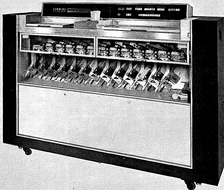
An Optical Document Processing System that can read any or all of the following codes or languages including a combination of any four of them on the same document in a single machine run transferring the information to magnetic or punched paper tape.
