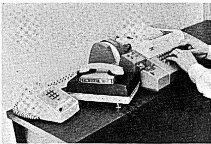
acoustic and a magnetic model for compatibility with most telephone equipment. Standard features offer half- or full-duplex operation, and a 72-character line (six lines/inch). Paper tape I/O with automatic start/stop is optional. COM-SHARE INC., Chicago, Ill. For information:
