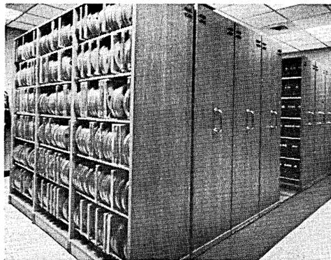
Loaded units of FULLSPACE glide left or right by hand to open one access aisle that does the job of five, six or more permanent space-wasting aisles always necessary with conventional fixed shelving. The elimination of permanent aisles saves floor space without sacrificing storage capacity. This installation permitted the storage of 30 per cent more computer tapes in 40 per cent less floor space and cut the cost per unit stored in half.
