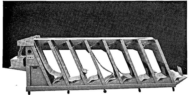
For high-speed decollating, this Moore Multi-Web Decollator does the job. Slits margins; removes carbons; separates opaques; refolds. In 4-web, 6-web, 8-web units. A real timesaver!
