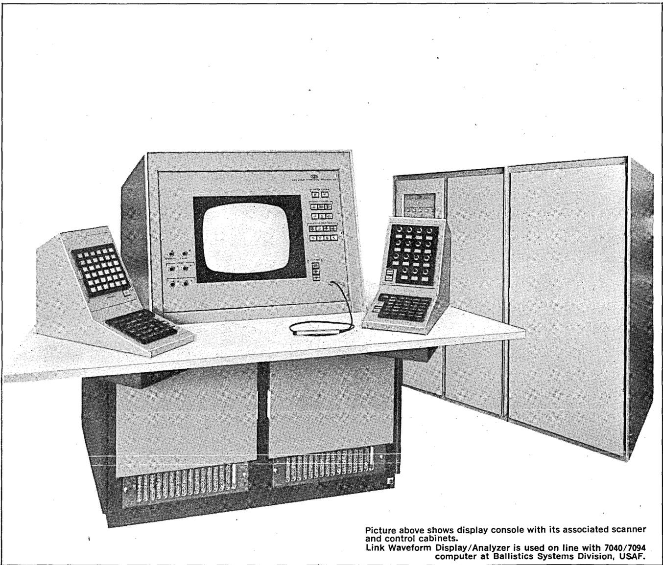
Picture above shows display console with its associated scanner and control cabinets.
