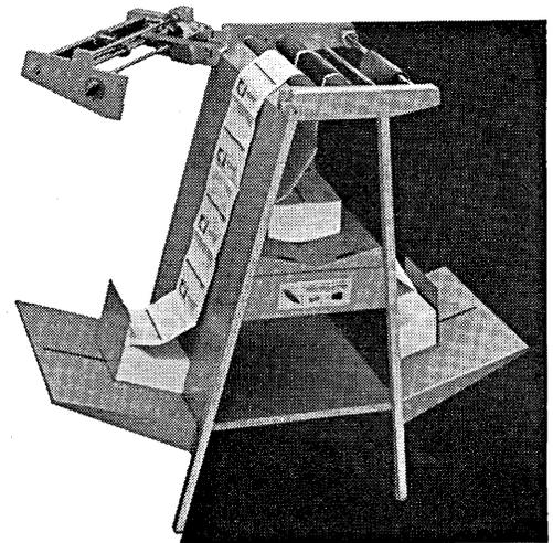
Where forms are to be decollated, carbon neatly rolled for clean, easy disposal, this Moore Decollator does the fastest job. Slitter attachment available to remove one or both margins.
