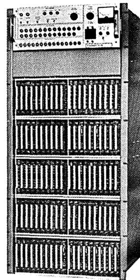
This typical 1-microsecond cycle time memory has a capacity of 16,384 words with 25 bits per word. Access time is 380 nanoseconds. The delay-per-bit in its memory stack is 12 picoseconds. For complete information about Fabri-Tek Memory Systems, write: Fabri-Tek Incorporated, Amery, Wisconsin; or call 715-268-7155; or TWX 510-376-1710.
