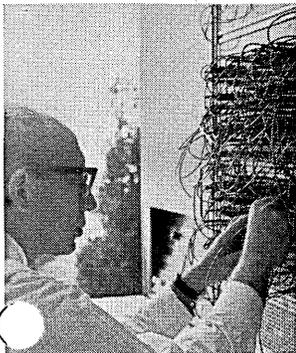
8900 DESIGN. The 8900 has excellent dynamic characteristics. The EAI 8800 Analog Computer has been designed with components directly behind the patch panel and maximum shielding to enable high accuracy 100-volt operation with component bandwidths of 125kc and higher. The 2mc parallel synchronous logic provides the extra time resolution which is essential with the higher frequency analog signals.
