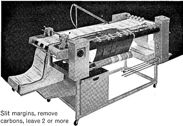
Slit margins, remove carbons, leave 2 or more parts held together for subsequent handling. Moore Power Deleaver removes carbons from continuous forms up to 8 parts.
