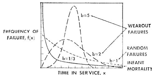
Varying one parameter ( $b$ ) in the Weibull distribution function allows the characterization of many types of reliability phenomena.
