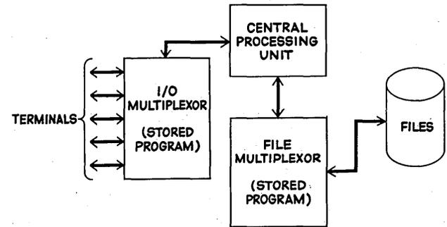
Fig. 4 Duplex System with Input/Output and File Multiplexors
