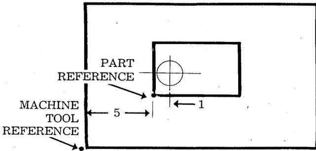
Thus, the X hole location is now six inches from the table reference. The next step is referencing to the spindle or absolute position, usually a function of the control.
