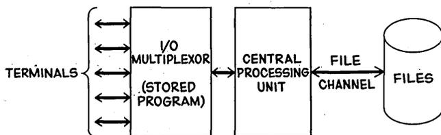
Fig. 3 Simplex System with Input/Output Multiplexor
