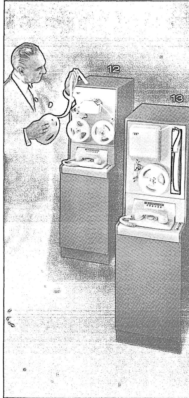
**HIGH-SPEED TAPE-TO-TAPE EQUIPMENT.** Used with DATA-PHONE and other communication services over voice circuits, this equipment is capable of 1,050 wpm tape-to-tape transmission. Shown above: (12) Sending Set. (13) Receiving Set.
