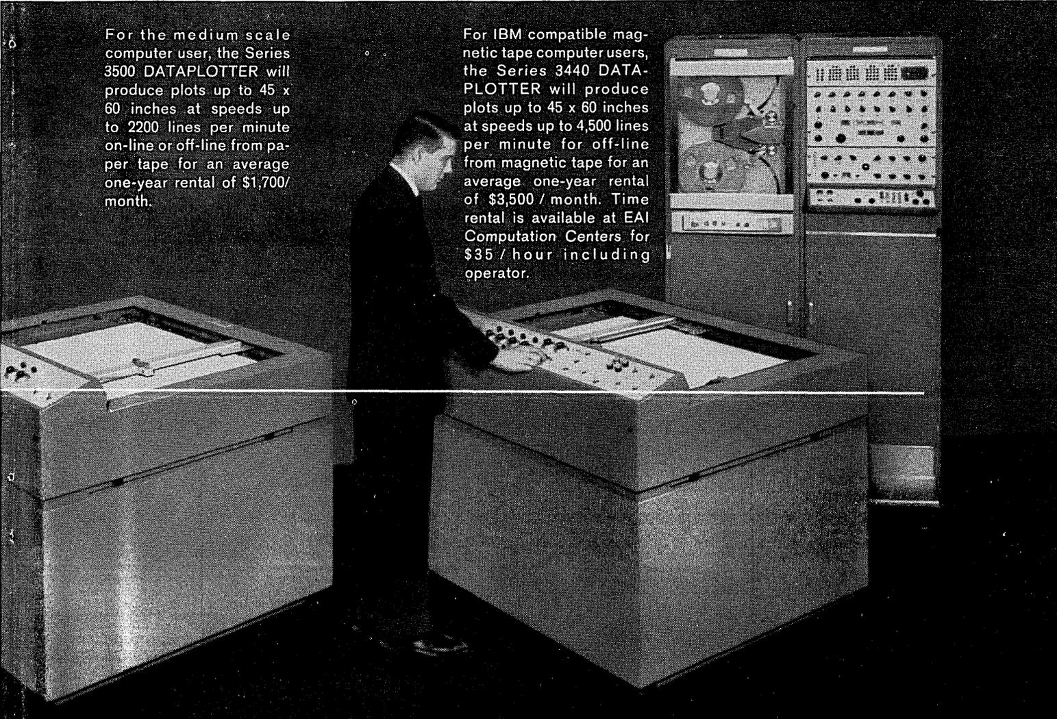
For the medium scale computer user, the Series 3500 DATAPLOTTER will produce plots up to 45 x 60 inches at speeds up to 2200 lines per minute on-line or off-line from paper tape for an average one-year rental of \$1,700/month.
