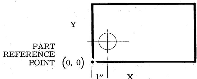
The planner must also specify once for the part, the relation of the part reference to the machine tool refer-
