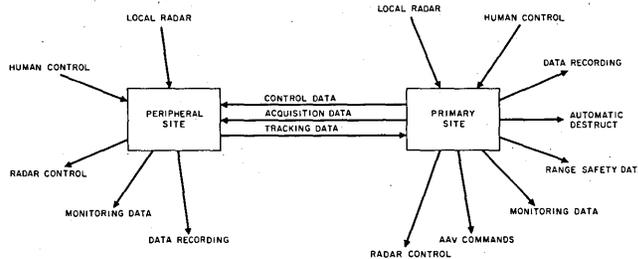
operator which could dictate data selection criteria, program mode change or sensor control. The manual input or control data could be generated locally or could originate at another site, usually one of the two primary sites. Peripheral sites output data to be used for acquisition, display and recording at local and/or remote locations.
