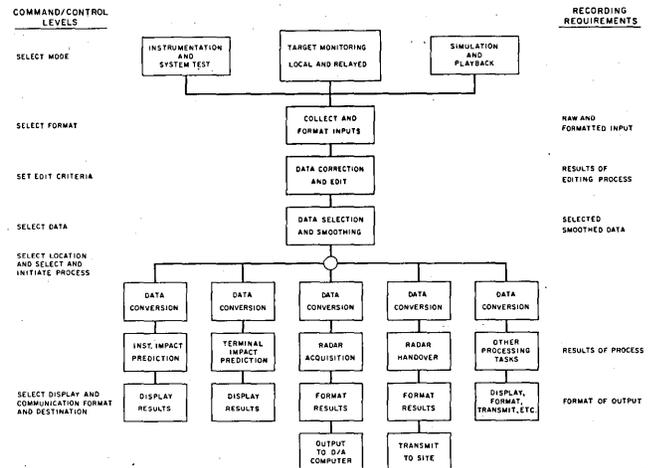
The flow of Fig. 5 shows the requirement of the RTDHS to process both instrumentation or system test data, and simulation or play back data. This requirement is difficult to implement in a system unless advance planning has taken the requirement into account. The distinction between actual data and non-real-time or test data tends to get obscured without adequate control.
