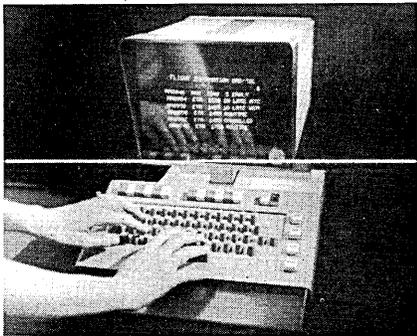
works with high concentrations of remote I/O devices, and the 200's are general purpose units. The CRT's can display from 128-768 characters, and the codes conform with the ASCII standard. THE TELEREGISTER CORP., 445 Fairfield Ave., Stamford, Conn. For information:
