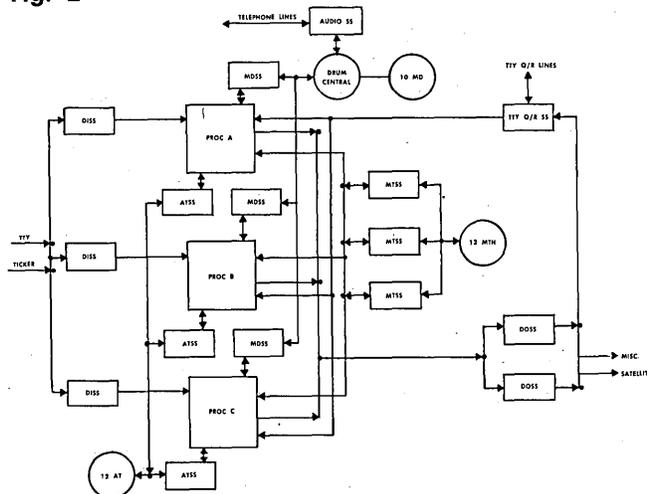
system (DISS) and flows to a processor (PROC). Programmatically, the processor has access to any magnetic storage drum (MD) via the drum control register (MDSS) and the drum central, to any magnetic tape handler (MTH) via a tape control register (MTSS), to any automatic typewriter (AT) via the AT control register (ATSS), and to output Teletype lines via an output control register (DOSS). Interrogations are handled via the Audio Subsystem and the Teletype Query-reply Subsystem (TTY Q/R SS).
