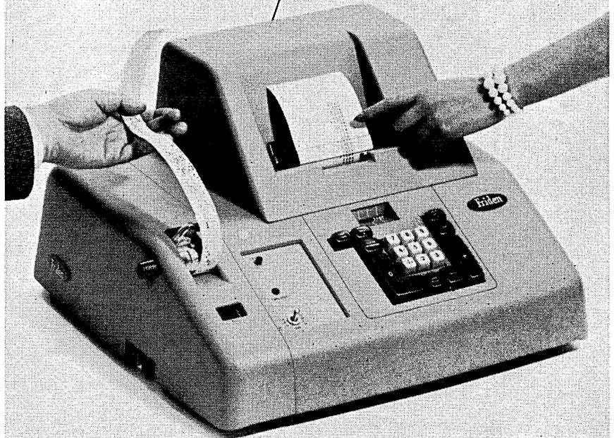
This is the Friden Add-Punch®, Model ACPT. Like any conventional adding machine, it produces a conventional paper tape establishing control totals.
