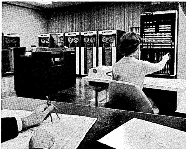
The 7044 is shown equipped with tape drives, printer and card read-punch. It may be enlarged with the addition of up to five disc files and the 1401. A design model of the operator's console is seen at the right and is similar to the 7040.
