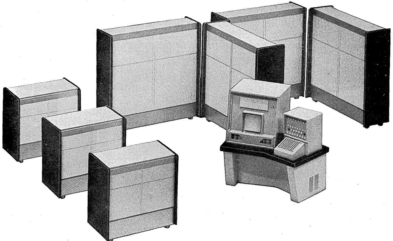
... provides a random access file of up to 495 million bits with access to information in less than 3/10 of a second.
