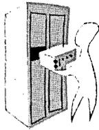
This new, high-speed DDP-19 (Digital Data Processor) is a single address, parallel, binary, 19-bit computer with a magnetic core storage of 4096 to 8192 words!
