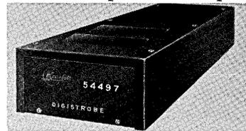
command, thus replacing as many as fifteen individual displays of existing types. Since this unit operates directly from the output register of a computer, counter or allied equipment, intervening circuitry is rarely required. GENERAL PRECISION INC., Kearfott Division, 1150 McBride Ave., Little Falls, N.J. For information:
