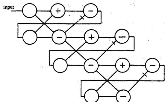
Figure 6. Examples of the parametron circuits
