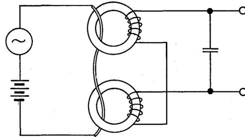
Figure 2. Parametron
