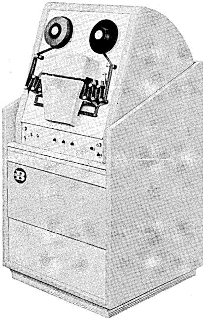
width tape, from five to eight level code. Plastic reels are available in two sizes, for tapes of 350 or 700 feet (40,000 or 80,000 characters). Features include automatic rewind and end-of-tape sensing, true straight-line loading and drift-free design. The photoreader is available as a component for mounting in any standard 19" cabinet. For information write ELECTRODATA DIVISION, Burroughs Corporation, 450 Sierra-Madre Villa, Pasadena, Calif. Or use card. *Circle 173 on Reader Service Card.*
