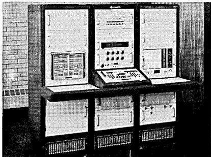
the patchbay assembly, a .01% reference voltage divider, a precision panel mounted vacuum tube voltmeter, and
