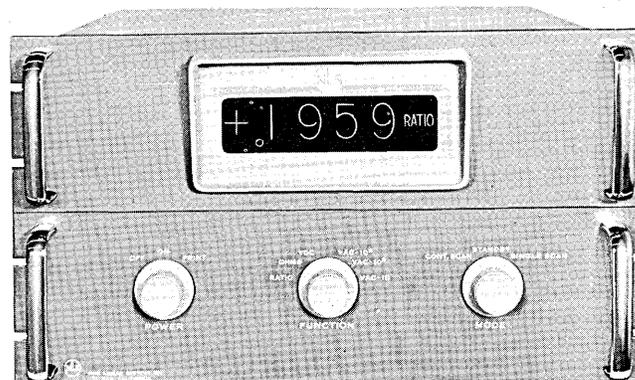
using precision stabilized wired-wound resistors and controlled by mercury relays. Series 20 has high input impedance, 10 megohms to 1000 megohms, operates card punches, electric typewriters and other printing devices. (Non-Linear Systems, Inc., Del Mar, California.)
