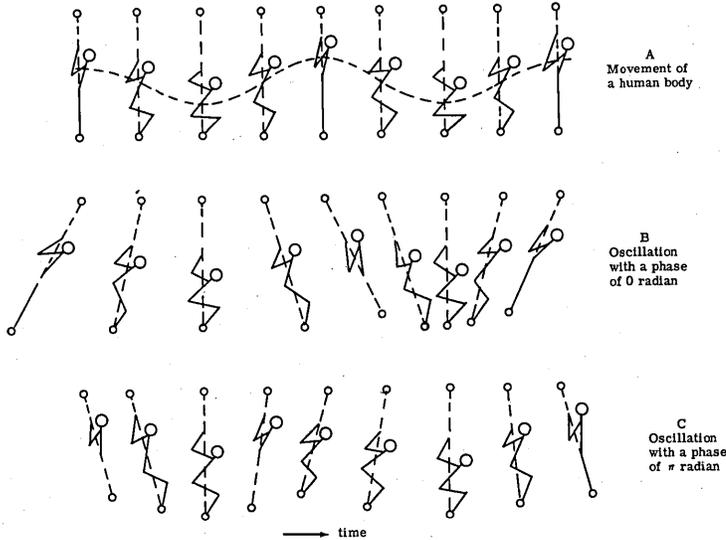
Figure 1. Parametron principle in a swing.
