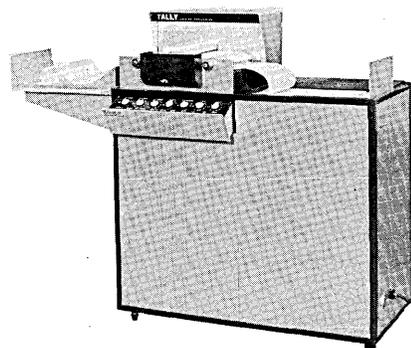
with random symbols. Results of computers can be plotted immediately. The plotted result is a series of mechanically generated printed impressions on paper or vellum. The act of plotting is a complex of mechanical
