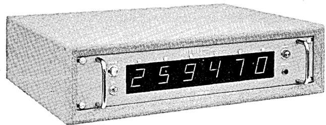
erates in response to a 1-2-2-4 binary code supplied by the manufacturer's counting instrument or some other source. The in-line indication does not change while the counter is actively scaling, but changes only at the end of a counting interval, at which time it displays the new total. Maximum display rate is 15 presentations per second. (Beckman/Berkeley Division, Beckman Instruments, Inc., 2200 Wright Avenue, Richmond 3, California.)
