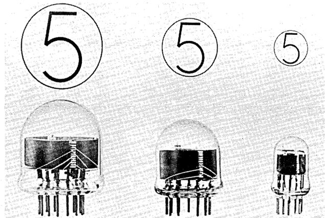
at a 50 KC rate. There are four basic types available: BD-200-S miniature, 6844-A standard, 7153 super, and BD-307 jumbo. (Electronic Tube Division, Burroughs Corporation, Plainfield, New Jersey.)
