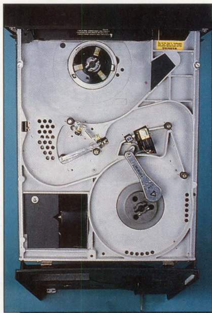
This top view shows the tape path. The drive automatically performs the loading.
