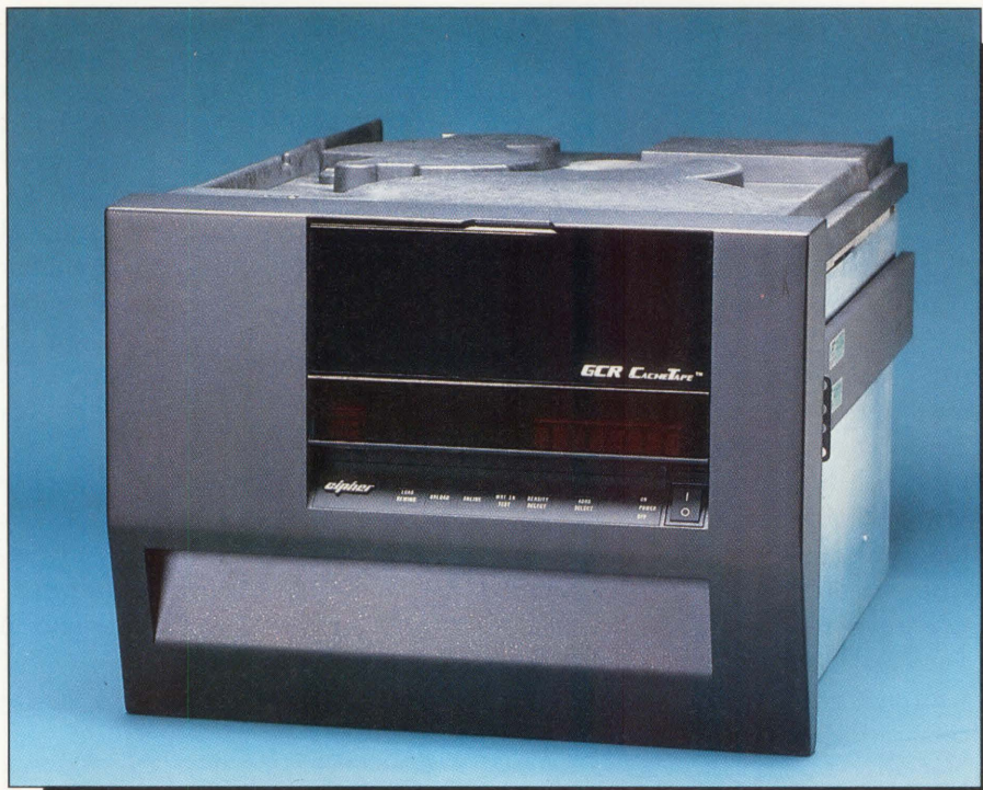
The Cipher M990 is 14 inches high, 17 inches wide and 22 inches deep.
