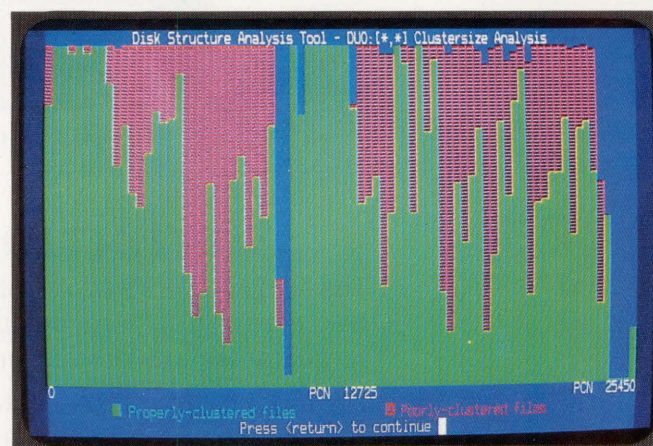
Screen 2: Cluster-size Analysis is another report provided by DSKBLD's Disk Structure Analysis Tool.
