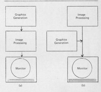
Figure 1-1: Multiple graphics and imaging functions – performed sequentially (a) or combined on monitor screen (b).
