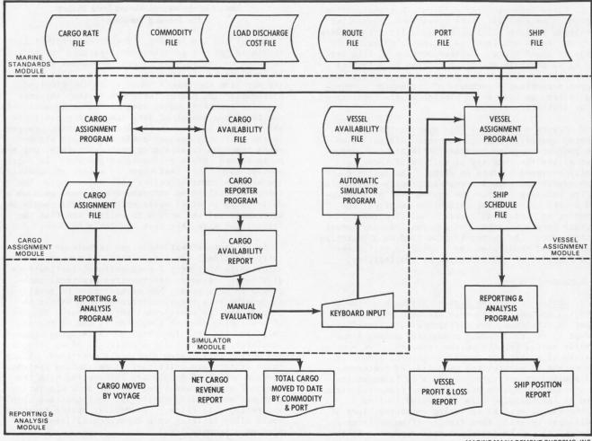
Figure 5: Marine Operations Simulator, Data Flow Diagram
