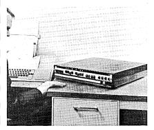
The minicomputer weighs 25 lbs., occupies  $3\frac{1}{2}$ " of rack space, and requires only 170 watts of power. I/O interfacing and all standard peripherals are available.
