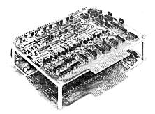
entire system is plugged into two standard (6  $3/8" \times 8"$  overall) stacked PC boards for integral equipment mounting and wiring. Two models are offered: the PDM-8/A is for decimal address; and, the PDM-8/B is for binary address. (For more information, circle #52 on the Reader Service Card.)
