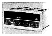
The PDC 808 has a 4,906 word 8-bit memory and 73 basic instructions. Memory is expandable to 16K words and processing is parallel with 24 microsecond ADD time. A flexible I/O section has DTL logic levels. Two priority interrupt lines and a third interrupt request line are standard. Many I/O options are available — including teletype, high speed tape reader and punch as well as magnetic tape. (For more information, designate #51 on the Reader Service Card.)
