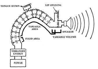
World's Fair in 1939. The Voder used two electrically-generated complex vibrations to create the sounds, a buzz representing the larynx tone (voiced sounds) and a hiss consisting of random noise (unvoiced sounds). Either of these sounds was applied to a group of bandpass filters which covered the range of speech frequencies. Each filter was separately controlled, and the outputs were combined, amplified and applied to a loudspeaker to form synthetic speech sounds.
