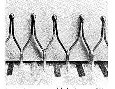
to spot a poor weld during quality control inspections. In the welding operation, the tips of a column of electrical terminals in the stacked core plane array are automatically and sequentially passed through the beam of electrons until the entire side of the array has been welded. The beam strikes each terminal approximately fifteen thousandths of an inch from its tip. All four sides of the array are welded in this way.
