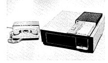
new device leaves the original document with the sender for permanent record-keeping. A number of readers can be connected to a central receiver. The reader is only 15" x 20" x 11" overall and weighs 40 pounds.
