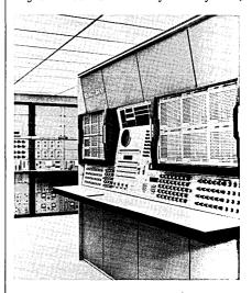
The standard model of the REAC-600 contains 300 solid state operational amplifiers of a new high speed type, giving it many times the problem-solving capacity of previous REAC models. End uses of the REAC-600 include design of space, automotive and other systems, automated railroad switching and many types of industrial and scientific research.
