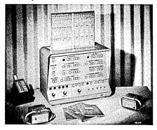
The system has the general capabilities of an internallystored programmed computer but has been design-limited for educational purposes. The BI-TRAN SIX has a coincident-current (15 microsecond cycle time) ferrite core memory with a capacity of 128 words of 6 bits each. A set of instructions are included which permit a wide latitude of problem solution at the basic level of programming.
