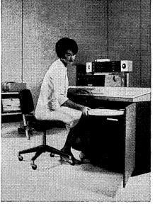
words of data on a single interchangeable disk cartridge. A basic disk model rents for \$895/month. You can transfer up to 35,000 words per minute on or off the file. Since the disks are interchangeable, a disk system is the ideal solution for an open-shop operation.
