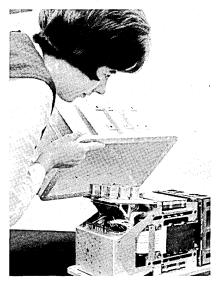
It measures just  $15 1/2 \times 9 3/8$ inches x 8 3/8 inches high, weighs under 46 pounds and consumes only 140 watts of power maximum. The 1824 has been successful in meeting the stringent high reliability, weight, power consumption, acceleration, vibration and temperature requirements imposed on present day aerospace computers. The completely thin-film memory consists of 4096 48-bit words of non-destructive readout (NDRO) and 512 24-bit words of destructive readout (DRO).
