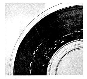
Complaint. Cinching during shipping, use or handling results when reel is wound under improper tension or exposed to temperature extremes.
