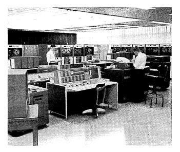
An IBM 7094 in M.I.T.'s Computation Center can be operated from the classroom via a time-shared console.
