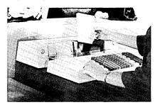
Data from a terminal is transmitted over communications lines to the computer through the IBM 1061 control unit and the IBM 1448 transmission control unit.
