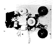
The printer may have 4, 8, 12, or 16 printing positions. Each position is capable of printing 0 through 9 in addition to 5 symbols, plus, minus, decimal, A and B (standard). The printer is of modular construction with a self-contained regulated power supply, timing circuitry, and a conversion matrix for the acceptance of 4 line codes.
