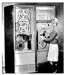
The device has a speed of 500 characters per second when operating in the magnetic tape mode. When converting data to paper tape, it has a speed of 250 characters per second. Five, six, seven, or eight-level paper tape codes can be accommodated, with or without parity. On the magnetic tape application, the converter operates with either the IBM 729 II/IV binary, or binary coded decimal low density format. Code translation, formating, and error-checking are performed automatically.
