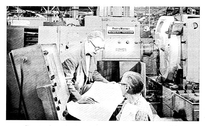
Figure 1 -- At the right is the helicopter gear box part, a large round slab of aluminum, with some of its depressions already machined. At the left is the operator's console. Not shown in this picture is the punched paper tape reader which controls the tool paths.
