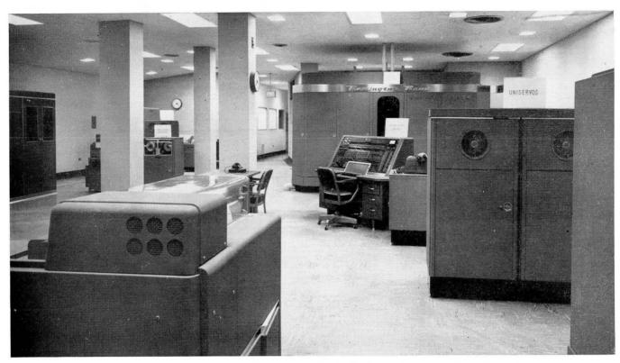
The new Computing Center at the Moore School of Electrical Engineering, University of Pennsylvania, Philadelphia, Pa., showing its powerful modern automatic digital computer, a Remington Rand Univac. The central machine is the supervisory control. (Figure 1)
