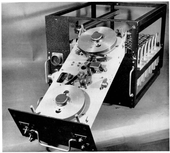
This is an airborne digital input recorder made by General Precision Laboratories, Pleasantville, N.Y. It will record on one-half inch wide magnetic tape a great quantity of data accurately. The digital form of the recorded data is compatible with International Business Machines Corp. computers Type 650, 704, or 705. In a typical application, the data from ten hours of recording of information in an airplane can be inserted into a computer in six minutes. (Figure 26)
