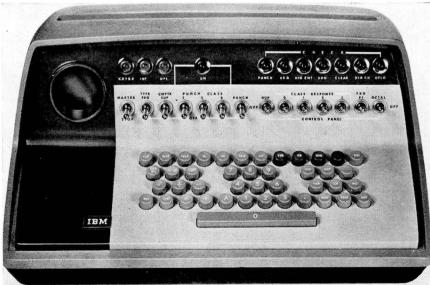
This is the input keyboard of the Type 610 Auto-Point Computer made by International Business Machines Corp. It enables a mathematician to solve a problem manually, and at the same time prepare a program tape so that all similar problems can be rerun automatically. Data can also be entered via this keyboard into tape for future use. (Figure 25)
