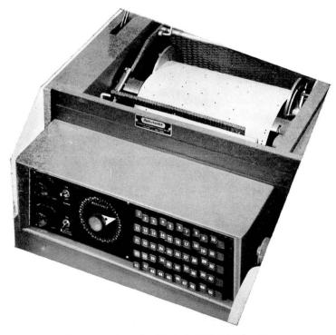
Above is a punched paper roll which automatically programs the keys of an electric typewriter, so that it will print any desired stored words or sentences. The machine is the Autotypist, made by the American Automatic Typewriter Co., Chicago. (Figure 10) Below is the wired plugboard of the Underwood Typewriter Co.'s Dataflo, which programs that machine. (Figure 11)
