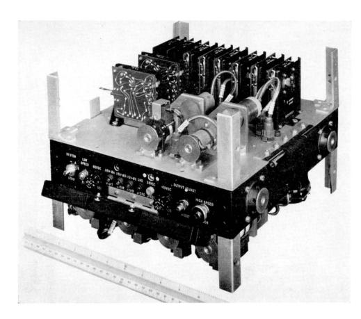
This is the upper chassis of a computer made by Westinghouse Electric Co., Air Arm Div., Baltimore, Md. It is a miniaturized analog computer less than 12 inches across, for air navigation purposes. The upper chassis shows six transistorized servo amplifiers, of the plug-in type and completely interchangeable. (Figure 18)
