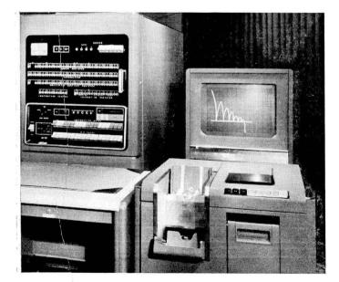
The visual display of the International Business Machines' Type 740 Output Recorder. Here, pictured on the face of a 21-inch cathode ray tube, are curves automatically traced showing the theoretical path of a bouncing ball as calculated by a big computer. (Figure 30)
