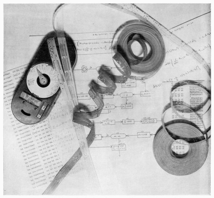
A mathematical formula is reduced to a flow pattern. The programming is worked out in a series of instructions. For example, the sixth instruction from the bottom is: 0be 2d46d2940a5 0b5 06d 0b5 00a 5
