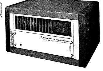
SPECIFICATIONS: Number of characters: 144; Number of bits/characters: 8\*, loaded or unloaded simultaneously; Loading or Unloading Speed: 14 µ. sec/character; Solid state components only. Signal Amplitudes: Input: ZERO-5 Vdc, ONE+5 Vdc, Output: Pulse: ZERO-5V, one +5v. Load Sync: +10v, Unload Sync. +10v. Power: 1 amp at 115v, 60 cps. \*Available in 4 bit model, specify 144-BQ4
