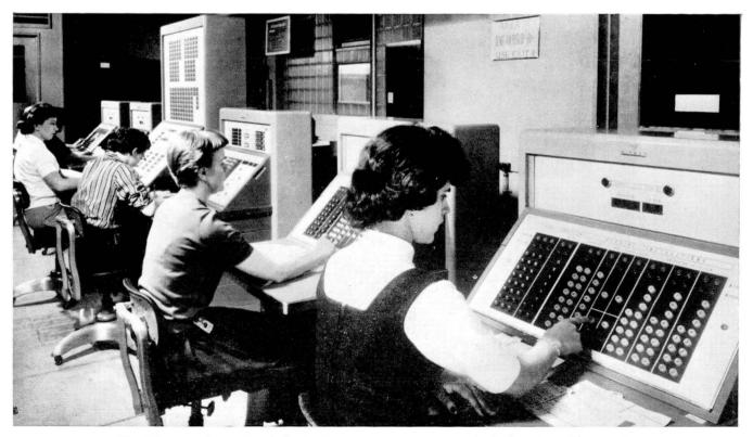
The "System Central" of the RCA Bizmac in Detroit, which functions like a telephone exchange. An operator at any one of these consoles can connect any of the 182 magnetic tape stations to the appropriate data processing machine by pressing a button; and she can tell from a glance at the control panel which machines are busy and which can take on a new job. (Figure 4)
