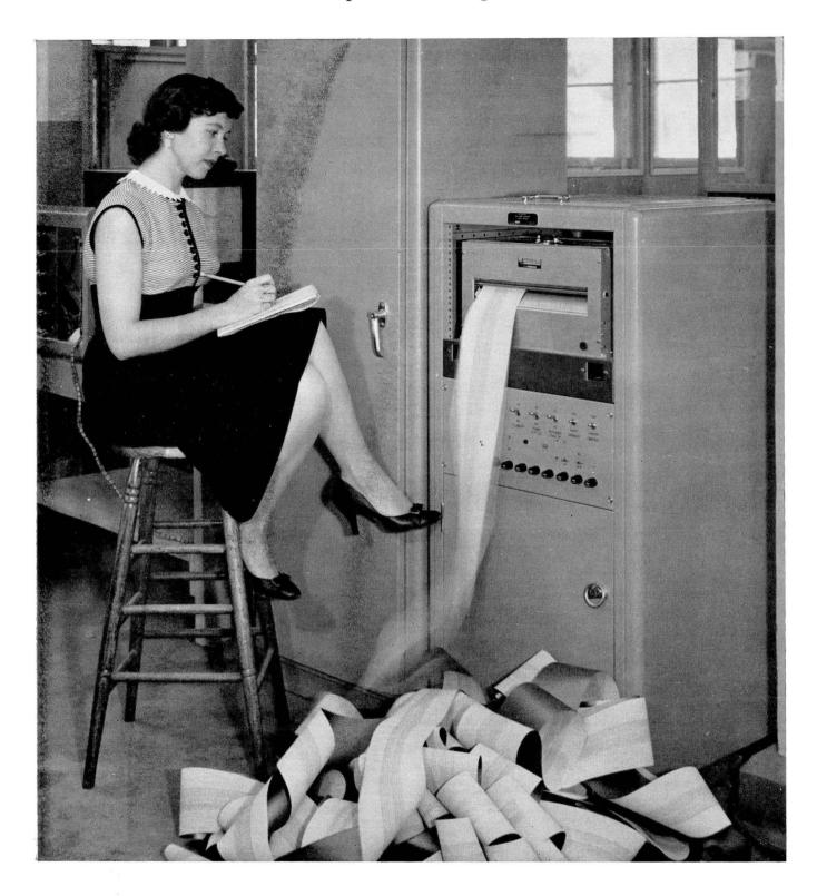
A digital printer, made by Radiation Inc., Melbourne, Fla., which produces 180 lines of printing per second, each line containing 12 numeric characters. The paper issuing from the machine is electrosensitive, marked by current passing through it. Each numeric digit consists of a selection out of an array of 30 points, 5 wide by 6 high. The speed of over 2000 characters per second is only about 500 times faster than a human being. (Figure 28) MATHEMATICIANS 1 TO 5 YEARS' EXPERIENCE INTERESTED IN
