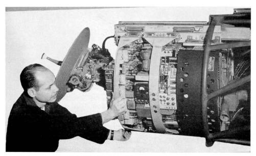
The inside of an airplane fire control computer installed in a U.S. Navy interceptor aircraft. The computer is an Aero 13 made by Westinghouse Electric Corp., Baltimore, Md. The fire control computer is mounted integrally with the radar at the rear of the assembly. (Figure 16)
