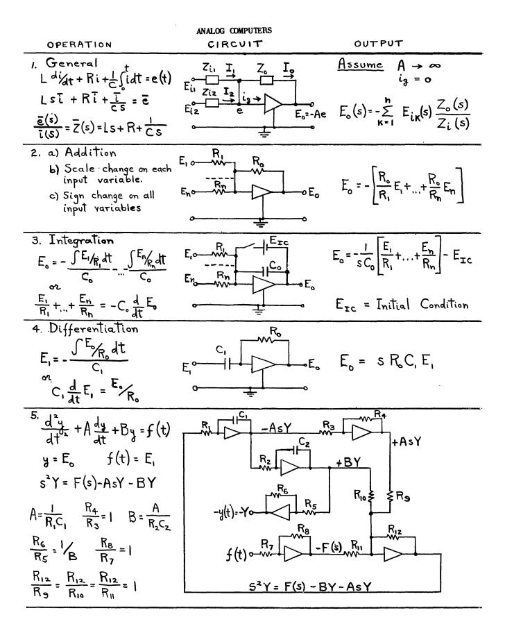
Figure 1 - Operational Amplifier Circuits
