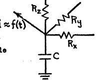
Figure 3 -- Analogous Electrical Circuits for Three-Dimensional Thermal Elements
