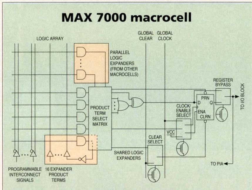
Macrocells within the MAX 7000 LAB provide both sequential and combinatorial logic capability, ensuring the most efficient implementation of a wide range of logic functions, according to Altera. Built into the MAX 7000 architecture are two types of logic expanders, shared and parallel (shaded areas); they provide additional product terms directly to any macrocell.
