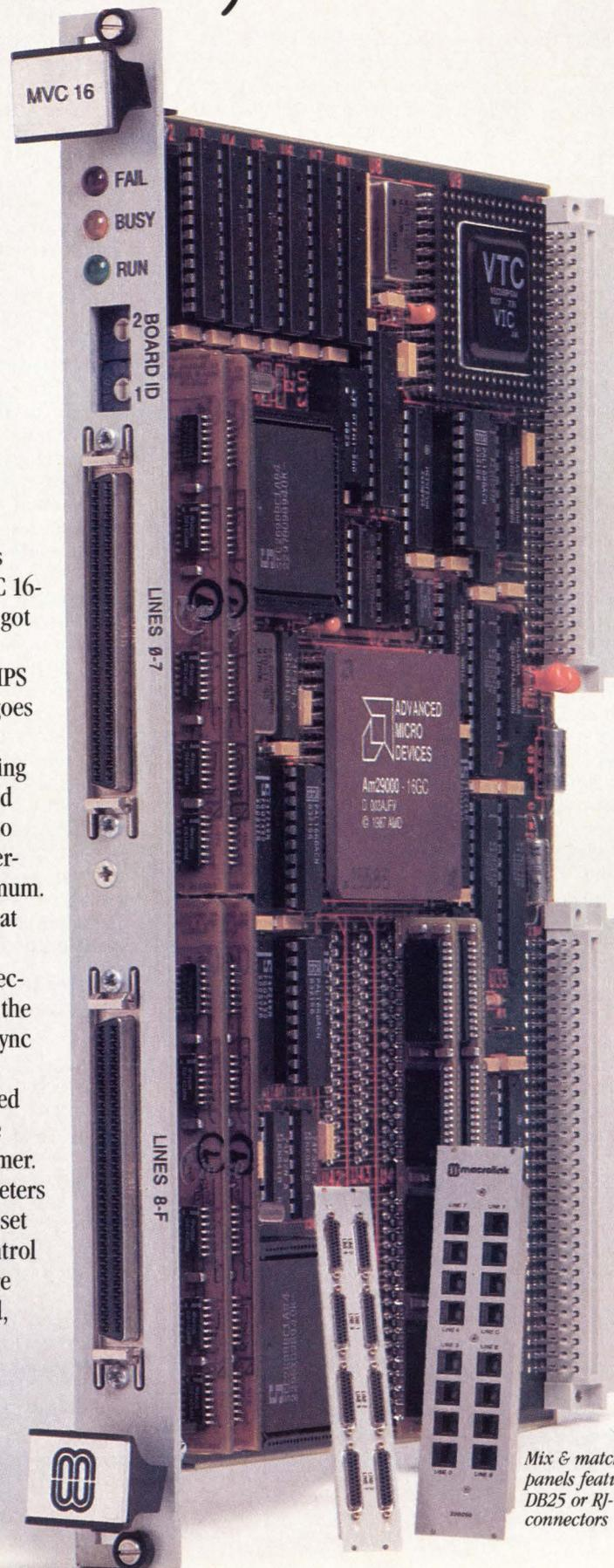
*Mix & match I/O panels feature DB25 or RJ-45 connectors*
