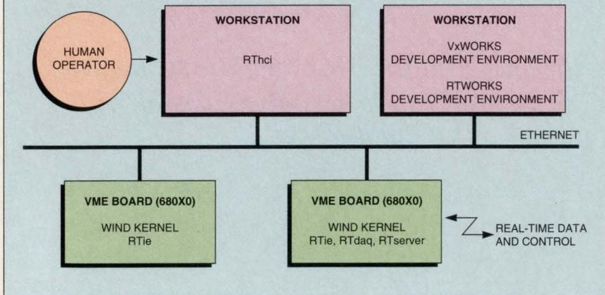
The combination of Wind River Systems' VxWorks with Talarian's RTtools lets designers build distributed real-time systems with a deterministic real-time kernel at dedicated nodes and distribute data anywhere it's needed on the network. Talarian modules will work with applications created with development tools already available under VxWorks.
