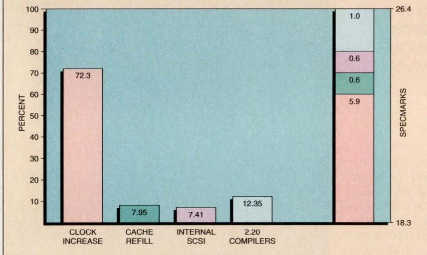
The 100 percent scale on this graph represents a 44 percent improvement of the 33-MHz MIPS RC3350 RISC CPU board over the 25-MHz RC3260—from 18.3 Specmarks to 26.4. That improvement represents more than a change in clock speed, which as shown here, accounted for 72.3 percent of the improvement. Other factors included a change in the cache design, addition of an on-board SCSI controller and improvements to the compiler.
