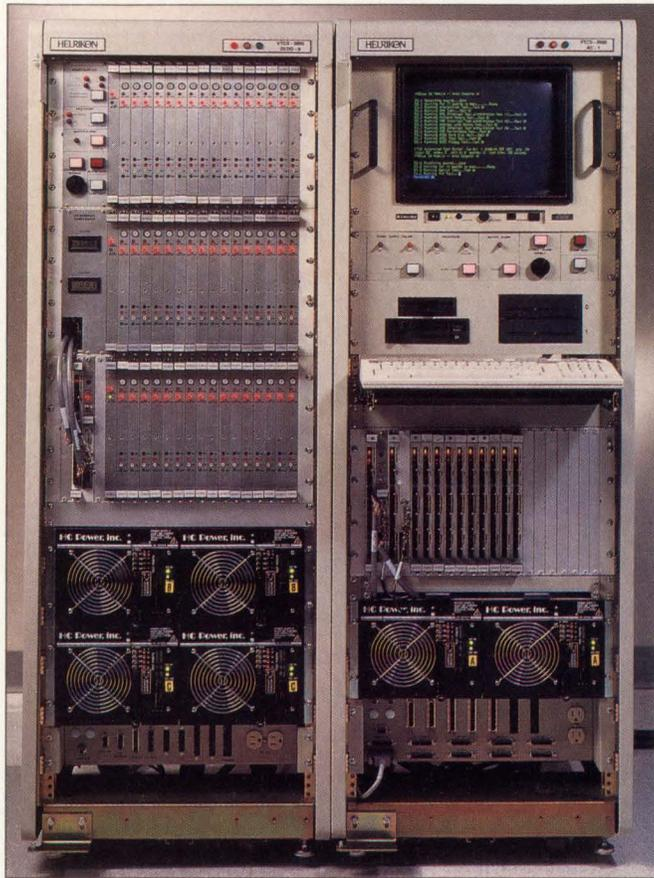
*New York City's new Vehicular Traffic Control System is composed of 11 digital I/O subsystems (left) and 18 area computers (right), designed and manufactured by Heurikon. Each area computer contains 10 to 12 Heurikon V30XE CPUs. Each DIOS contains 48 digital I/O cards, three controllers and one V30XE CPU.*
