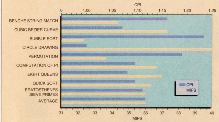
Different benchmarks run on the Sparlite processor at the same clock speed show relative invariance in terms of cycles per instruction (CPI). Fujitsu reports this same invariance over several different compilers, although the completion times for the benchmarks vary because of compiler differences.
