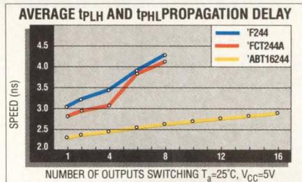
**TI's speed advantage:** In a one-to-one comparison, a TI 'ABT16244 16-bit Advanced BiCMOS driver proves to be much faster and more stable than Advanced Bipolar and standard CMOS octal drivers.
