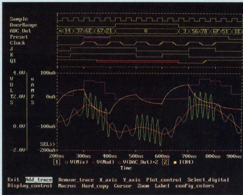
PSpice features mixed-mode simulation where analog and digital waveforms are displayed, aligned in time.
