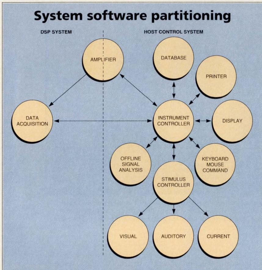
The software development team was divided into two groups—while one group worked on 56001 assembler code to handle real-time/data acquisition, the other developed control code in C for the OS/2-based graphical user interface. The partitioning of the two groups let them work at their own rates.
