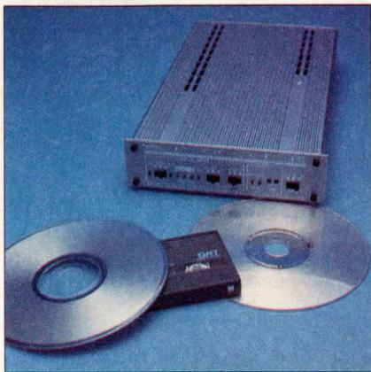
*When designers at Apogee needed to choose an audio D-A converter to use in their digital audio monitoring system, they decided that the sigma-delta converters, although cheaper, didn't have the performance they needed. Instead they chose the PCM63P, Burr-Brown's 20-bit audio DAC. They liked the way its dual-DAC per channel architecture prevents glitches.*
