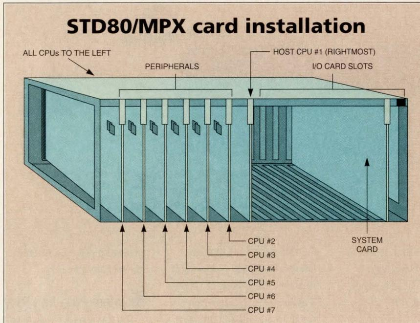
The new multiprocessing architecture proposed by the STD MG, the STD80/MPX, uses a simple arbitration scheme assigning CPU boards priority based on the slot in the backplane in which they reside. The CPU farthest to the right has the highest priority, with decreasing priority going to the left. The right-hand card slots are used for I/O.
