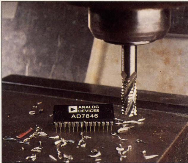
*In closed-loop servo control applications such as this drilling machine, D-A specifications such as monotonicity determine the degree of precision at which the tool can operate. Analog Device's AD7846 is 16-bit monotonic over a temperature range of -55 to +125°C. Its 100-mW power dissipation and small 28-pin package make it suitable for portable applications.*
