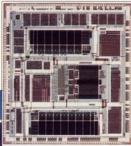
Cypress has integrated a multiprocessor subsystem on a multichip module (MCM) using its Sparc processors and CMU. Both processors and boards are interconnected using M bus. Shown is the Cypress Sparc core module for dual-processor multiprocessing, the CYM6002K. The heart of the system is the 605 CMU (insert), the solid-state implementation in silicon of the M bus multiprocessing protocol.
