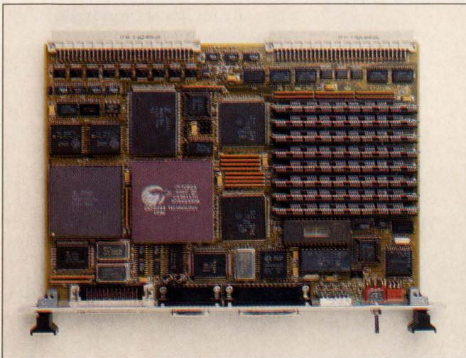
*The first SunOS Sparcstation-compatible VMEbus CPU to emerge outside of Sun is this 2SE high-performance single-board computer from Themis. The board, the first to be designed around the Sparc M bus, features SCSI and Ethernet ports as well as a selection of memory options.*
