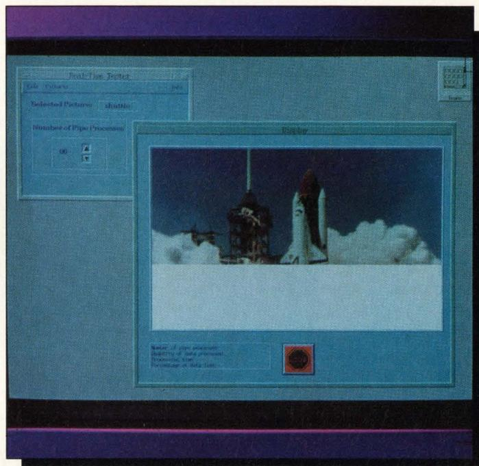
**Performance measurement tools for real-time systems can be used to test relative performance of systems and software. The Real-Time Tester from Modcomp lets you select a number of real-time processes in a pipeline and pass data through them. The data then forms an image at the end of the pipeline. Watching the image grow gives you a feel for the speed of the system.**
