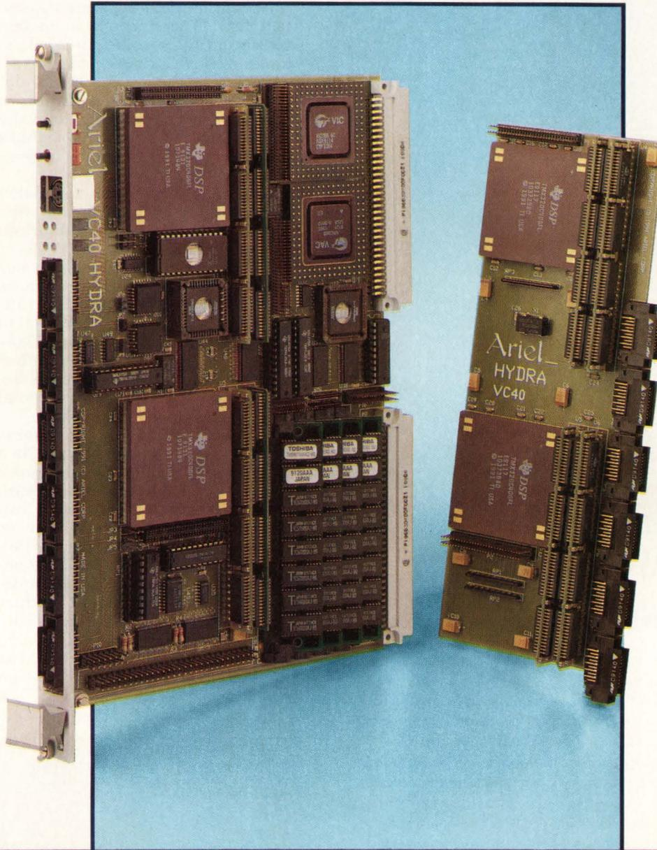
Only Ariel's Hydra combines four TI TMS320C40 DSPs to deliver twice the processing speed and four times the I/O bandwidth of any 6U VMEbus coprocessor card. It's the only choice for the most compute-intensive multiprocessor applications.
