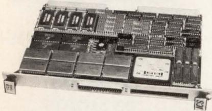
**8-Channel, 16-Bit Analog I/O Board
