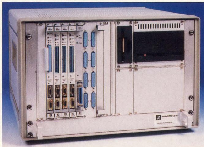
*A typical multi-processing system comprises a number of CPU boards and some I/O functions in a single crate. Systems can be as compact and self-contained as the one pictured here.*
