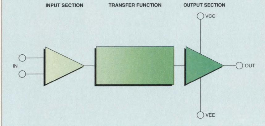
*Zeelan's ModelStation has a proprietary, automated root extraction capability which produces Laplace transform behavioral models of analog components or circuits. The system can produce a "black box" transfer function from input and output responses in a single-pass operation. According to Zeelan, the resulting behavioral model can simulate about 1,000 times faster than a comparable detailed circuit-level simulation and still provide almost as much accuracy.*
