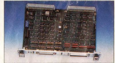
The DB-PCOMM high-speed 32-bit Parallel Communications Module.
