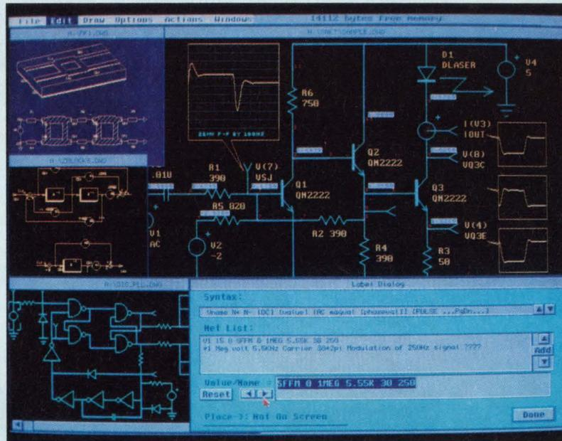
Intusoft's embedded schematic tools permit simultaneous display of schematics and waveforms at selected nodes of the circuit.
