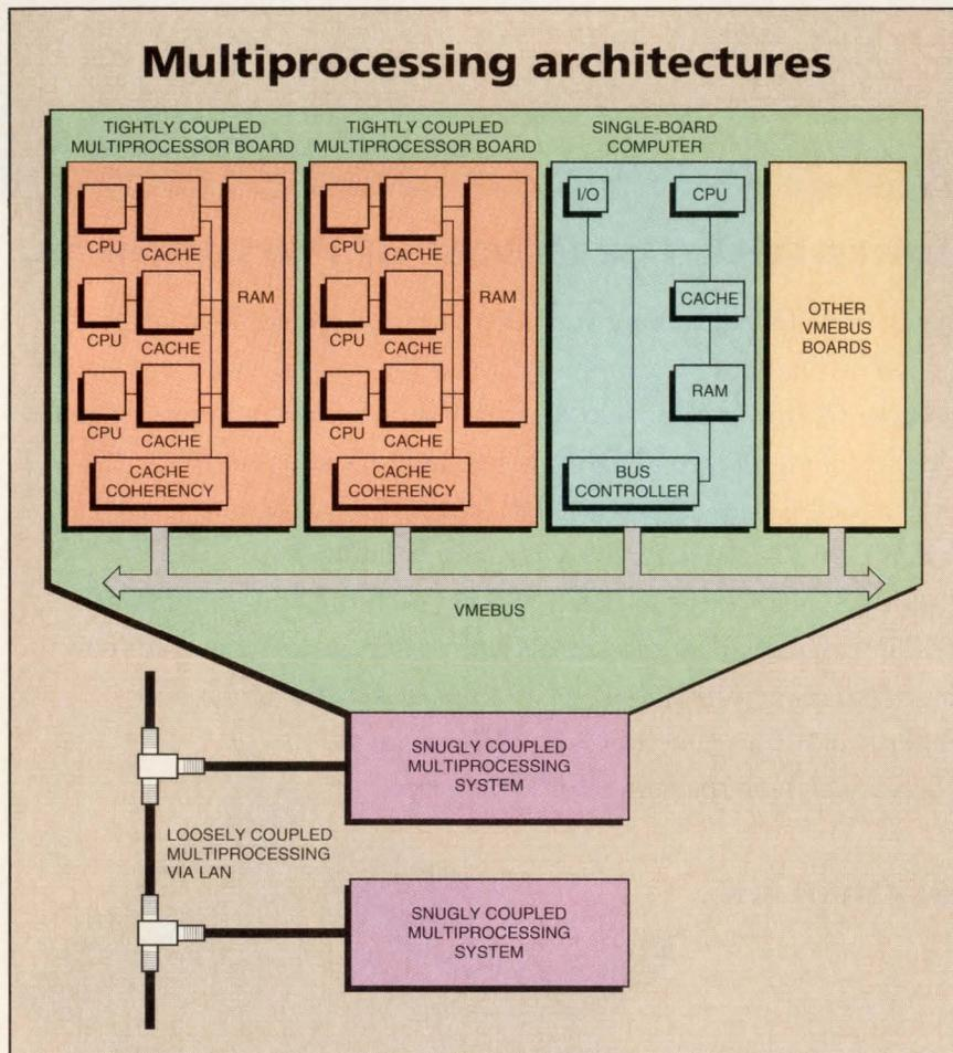
Lynx Real-Time Systems has its own definitions of the hierarchy of multiprocessing architectures—shared-memory approaches it calls tightly coupled, networked systems are loosely coupled, and systems linked by a backplane are "snugly coupled." As the diagram shows, all three categories can function in a single system.
