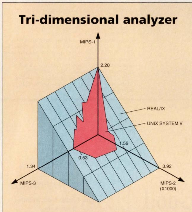
*The Tri-Dimensional Analyzer from Modcomp shows relative throughput for CPU (MIPS-1), interrupt handling (MIPS-2) and I/O throughput (MIPS-3) for a real-time system. This graph compares real-time performance of Unix System V (red plot) with the Real/IX version of Unix designed for real-time. Real/IX shows a much more symmetrical relationship among the three parameters.*
