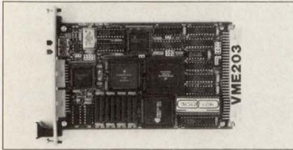
Micro-Link's VME203 SBC makes your design choice easy. Available in several configurations, VME203 prices start at less than \$1,025 in 100 piece quantities. Options include 68EC030 or 68030, FPU, 1 or 4 MB of DRAM with transparent refresh, burst mode Cache, up to 1 MB of EPROM, two RS-232 serial ports, and clock speeds of 16, 32 and 40 MHz. VME203 software support includes Microware OS-9®, CrossCode®, C/FreeForm™ and Microbug II.
