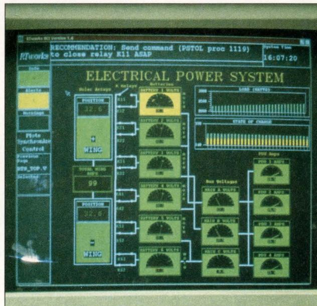
Talarian's RTworks includes a human-computer interface module, *RThci*, that lets you build point-and-click user interface screens to monitor and control real-time processes via other RTworks modules.
