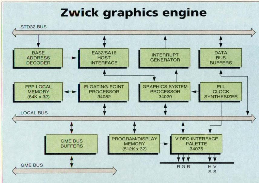
One of the first high-resolution graphics engines to emerge on STD32 provides flexibility by using a multiple-bus architecture. It uses its own local bus in addition to the STD32 host bus. It also provides a GME (Graphics Memory Expansion) bus which is essentially an extension or pin-out of the graphics processor. The GME also lets the board operate with other subsystems adhering to the GME specification.
