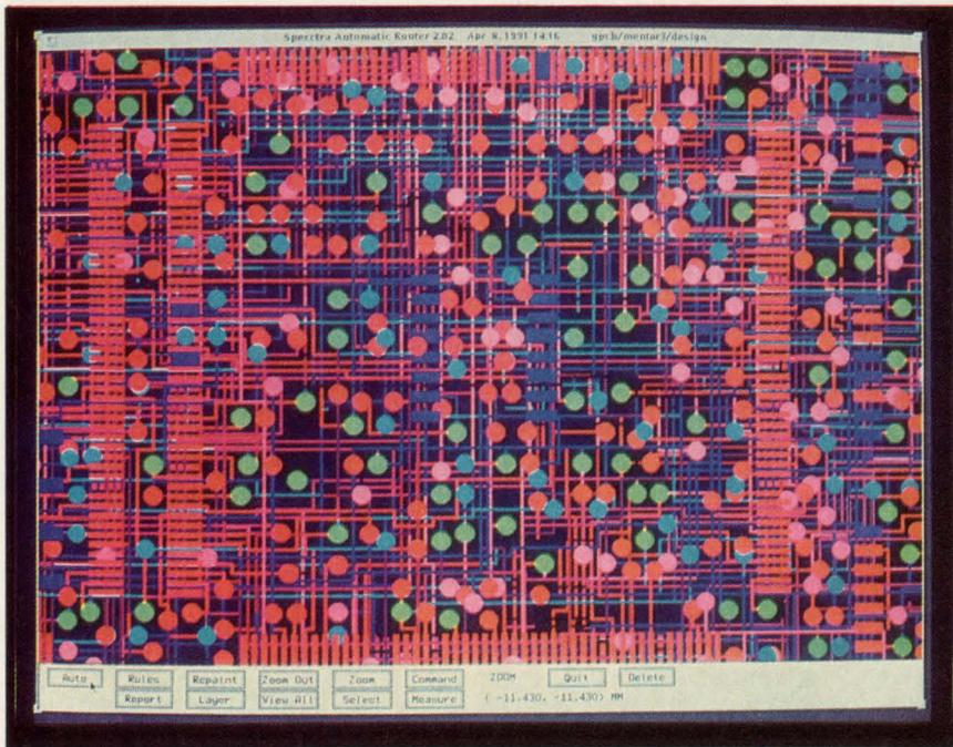
The Spectra autorouters incorporate complex design rules into the autorouting algorithms to account for SMD-specific manufacturing constraints. Soldering requirements, component densities and through-hole options are considered during routing.
