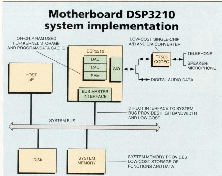
By sharing system DRAM resources, rather than using its own dedicated SRAM, the AT&T DSP3210 device lets designers build low-cost motherboards with DSP. To help minimize glue logic, the port features a bus interface compatible with Intel and Motorola processor families. The question is, who will use the device on a motherboard first?
