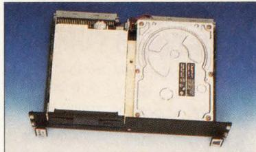
The DSM (Data Storage Module) for high-performance real-time systems.
