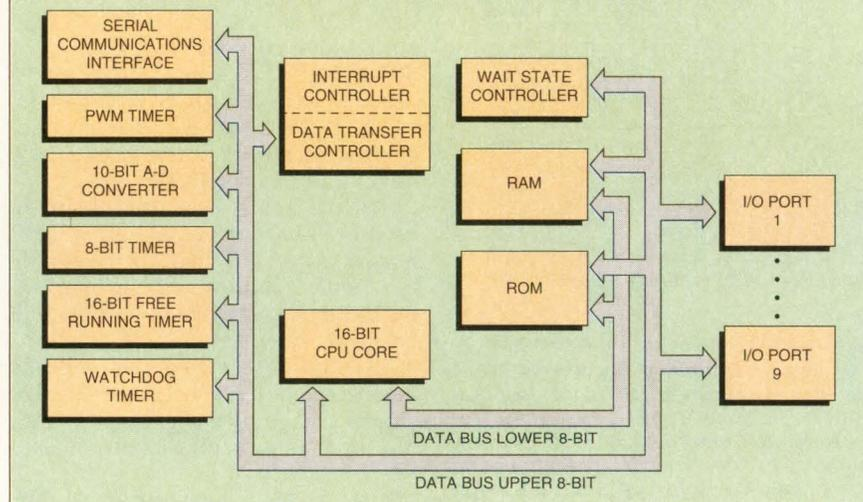
While the H8/500's CPU core and internal CPU-to-memory data bus are 16 bits wide, the chip's data transfer controller can be programmed to automatically move 8- or 16-bit values between any type of on-chip peripheral including timers, interrupt controllers, memory, and general-purpose I/O. Address bus not shown.
