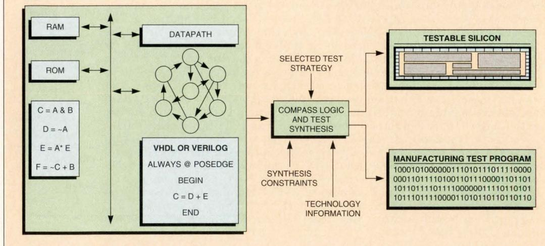
Compared to other tools, Compass Design Automation (San Jose, CA) claims that its ASIC Navigator toolset offers a broader test synthesis solution to VHDL users, one that enables an entire ASIC and its associated test circuitry to be synthesized. Compass users can synthesize not only random logic, but also RAMs, ROMs and datapath elements. In addition to manufacturing test, Compass offers BIST and boundary scan for field diagnostics.
