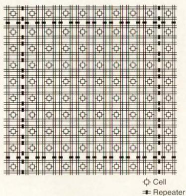
For design flexibility, Concurrent Logic developed a symmetrical array of identical cells for its CLi6000 FPGAs. Except for "repeaters," or connective units spaced every eight cells, the array is continuous and completely uninterrupted from one edge to the other. Repeaters are aligned in rows and columns, thereby partitioning the array into 8 x 8 blocks of cells.
