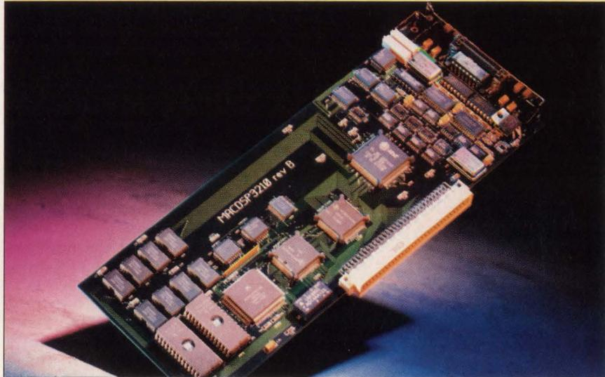
The MacDSP3210 board and AT&T development software let designers use a Macintosh host system to develop low-cost multimedia and digital signal processing systems and applications.
