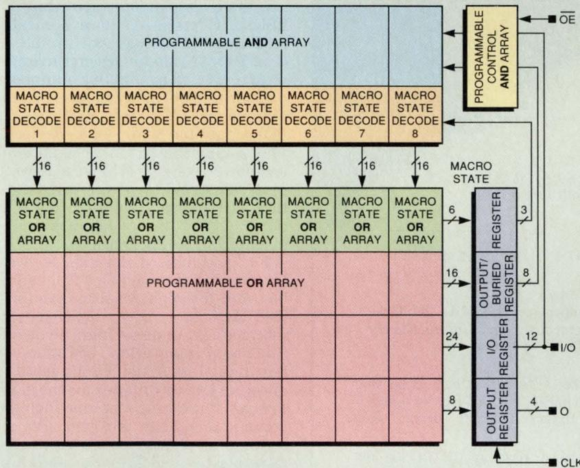
fixed feedback paths to a global bus determine which of eight PLA pages on the MAPL128 is enabled. Since only necessary logic terms are active, the MAPL128 draws just 140 mA max. from the supply. A worst-case system speed of 45 MHz, with feedback, is guaranteed across the MAPL product line.
