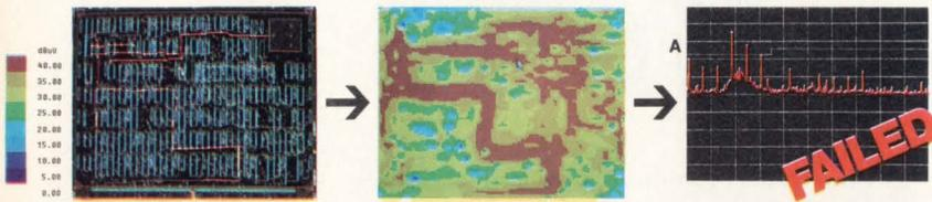
Hot traces identified early at the layout stage with PCP EMSIM indicate this board design will likely fail EMI radiated emission tests.
