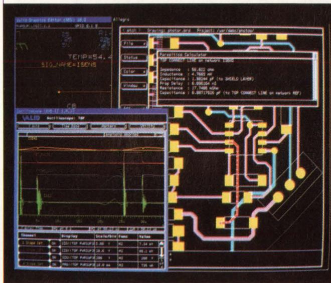
*Valid's Analog Systems Lab is an integrated environment for front-to-back design. The windowed display allows multiple simultaneous views of data. Here the circuit layout window (right) is overlaid with a parasitic calculator window. On the left an oscilloscope window is superimposed on the graphics editor.*
