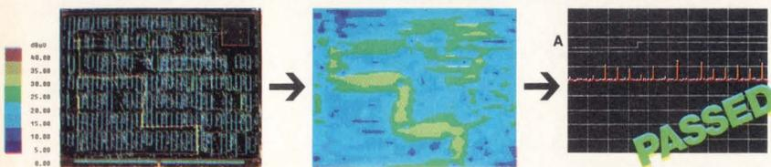
Optimizing component placement and routing with PCP EMSIM allows you to attack EMI before costly hardware prototyping.
