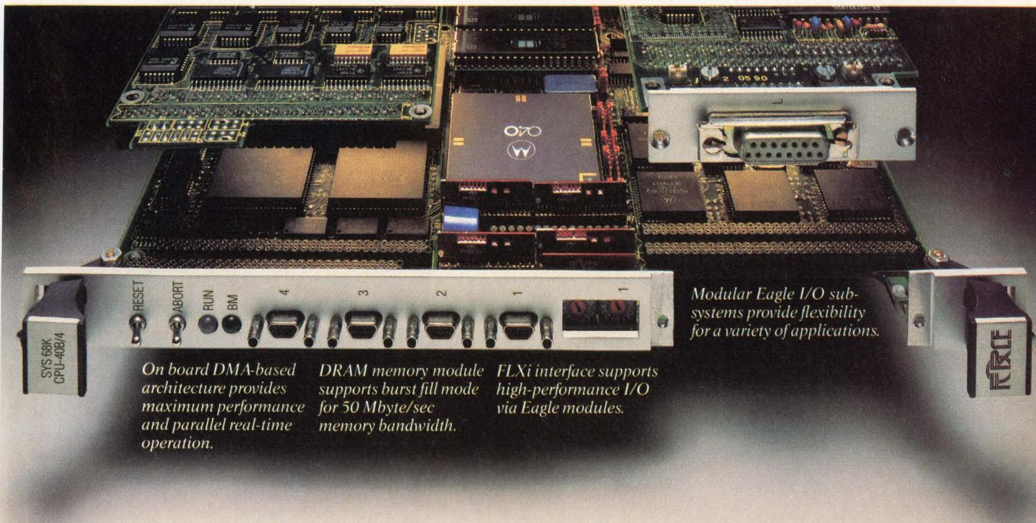
*Modular Eagle I/O subsystems provide flexibility for a variety of applications.*
