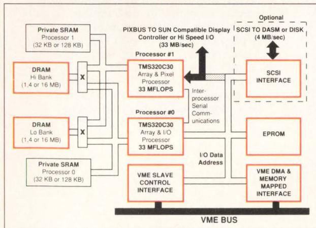
The MSP-6C30 is a 66 MFLOP, floating-point, VME array processor optimized for signal and image processing. High performance is assured through a unique, multi-banked, crossbar memory architecture, and high bandwidth is achieved with multiple, fast, industry standard I/O ports. Also available in a PC-AT version with optional VGA compatible display controller.
