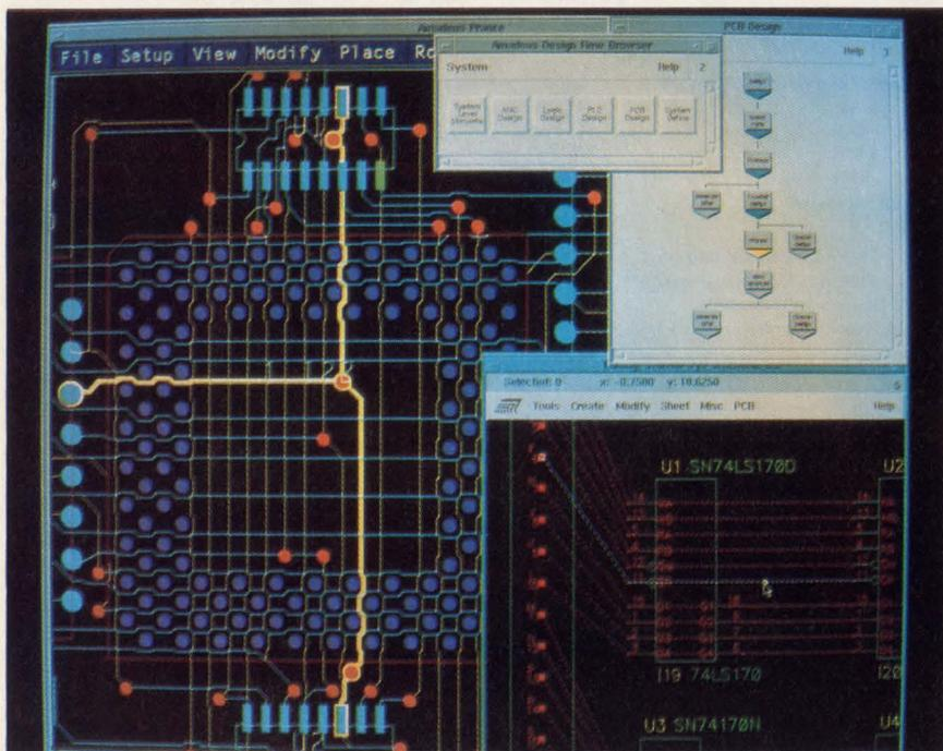
Framework technology is making possible tight integration of tools. In this view of Amadeus Prance from Cadence Design Systems, cross-probing of a signal in the schematics highlights the associated trace in the board layout. The windows in the upper right display design flow information.
