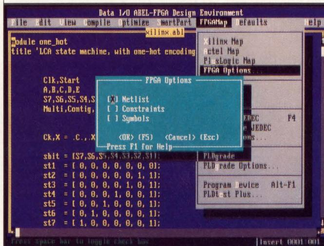
placement and routing of FPGA architectures. Optimization features include new criteria for netlist generation based on the details of specific FPGA architectures. In addition, menu features have been included to support FPGA design flow.
