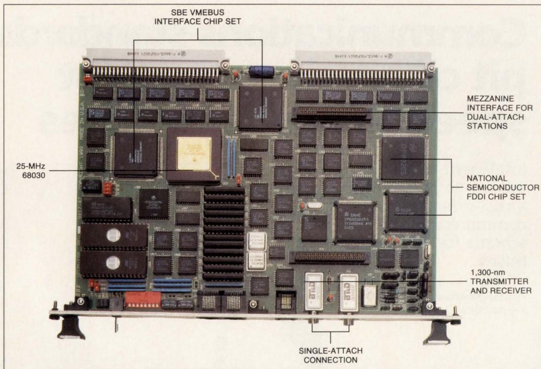
*Efficient communications using a standard such as FDDI requires some means of handling the considerable overhead of its protocols. High-performance controller cards (such as SBE's 68030-based VCOM-100) depend on local processors keep the protocol from slowing the system host. This configuration supports single-attach FDDI; dual-attach connections require a daughtercard.*
