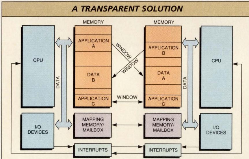
*Augment's proprietary high-speed communications capability is designed to be transparent to linked systems. It allows applications executing on either system to access data on a linked system as if they were local.*
