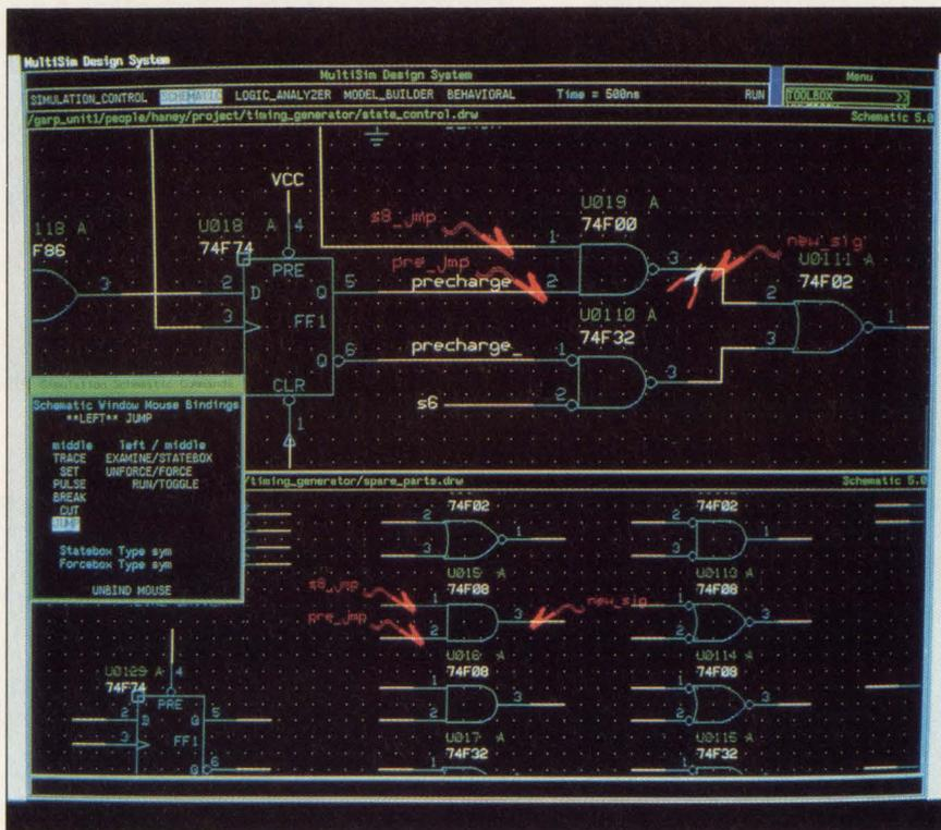
Teradyne's MultiSim interactive designer uses on-screen icons and mouse-driven controls to let designers modify schematics. In this software cut and jump operation, changes are made to selected circuits, with no need for recompilation and resimulation.
