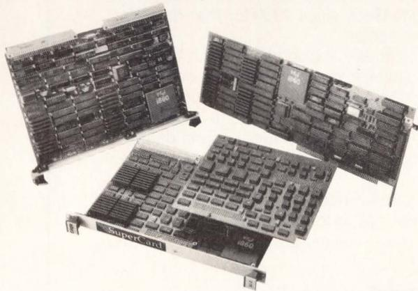
The second generation of i860-based SuperCards™ is here... vector processors with GigaFLOPS system capability, concurrent I/O via secondary buses, large math libraries, FORTRAN and C development software... and, best of all, the *best price* on the market. The SuperCard family is compatible with VMEbus, ATbus, EISAbus and TURBOchannel platforms for hosts like Sun, HP, Motorola, Compaq, and DEC... here's what you get:
