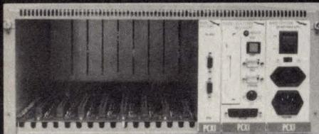
Shown here is a 386/33 EISA industrial computer, with a passive backplane providing six EISA bus master slots, one slot-specific slot and four AT slots.
