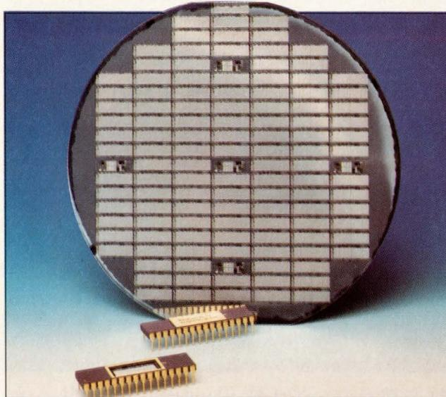
*Built with a proprietary dual-well 0.8-µm CMOS technology, a 128kx8-bit SRAM from Paradigm Technology offers access speeds down to 20 ns. The company uses a self-aligned process that's designed to eliminate empty space in the cell, enhancing density and speed.*
