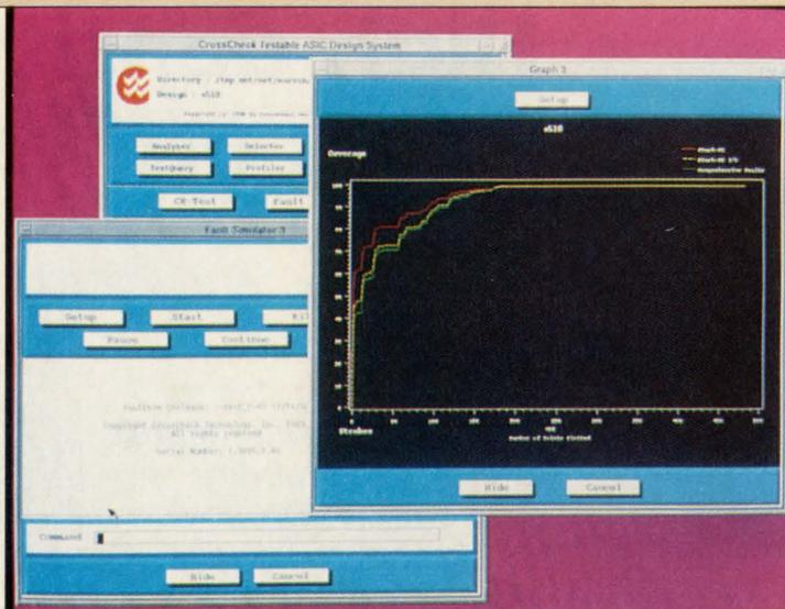
CrossCheck CX-Test 1.4 software adds controllability to the 100 percent observability provided by a matrix of test points embedded onto the base wafer. As shown in the chart, CrossCheck's observability achieves high fault coverage, typically better than 95 percent, with fewer vectors. Automatic test-pattern generation provides additional coverage (between 2 and 4 percent). The system test level ASIC design display shows a graph that identifies fault coverage vs. the number of vectors used.
