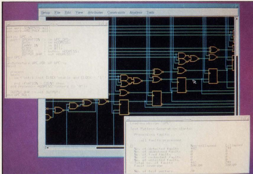
The Synopsys Test Compiler displays a synthesized VHDL module that has had scan registers inserted. The fault coverage report (lower window) shows fault coverage and a breakdown of faults. Test Compiler synthesizes scannable gate-level designs from register-transfer-level VHDL descriptions.
