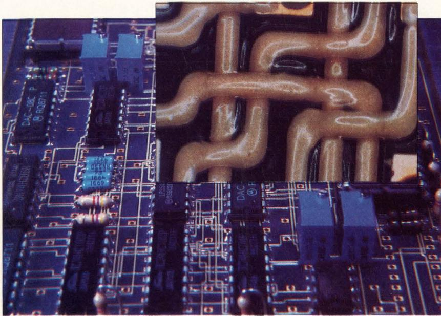
*Fast return of a prototype can shorten a printed circuit board's design cycle by weeks. The CircuitWriter system from Ariel Electronics can produce a prototype from a user's netlist and placement data in one day. Using a proprietary polymer thick-film technology, the system can create circuits equivalent to 6-layer, and even some 8-layer, copper circuit boards. Such densities are possible because the system allows trace crossovers and multiple traces between pads.*
