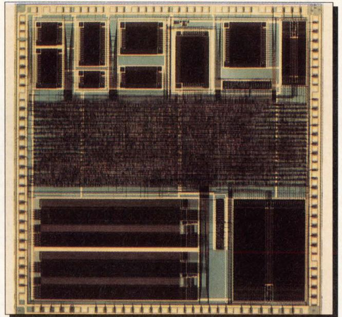
*Complex ASICs, such as this macrocell-laden telecommunication circuit built in AT&T Micro-electronic's 0.9- $\mu$ m CMOS Standard Cell Library, combine high density with testability. Fault coverage for the macrocells and BIST (built-in self-test) overhead is greater than 99 percent. Test time is less than 1 percent of that required without BIST.*
