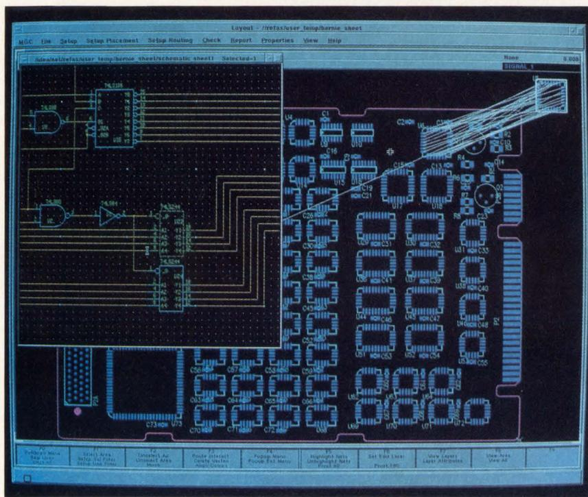
Though automatic placement tools are available, most designers prefer an interactive approach, which combines the power of the computer with a designer's expertise. In this split-screen view of Mentor Graphics' Board Station, a schematic and the associated printed circuit board layout let the user keep track of connectivity requirements to ensure better placement for routing.
