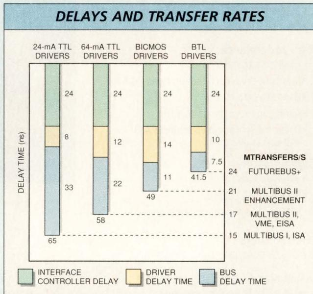
The maximum transfer rates for standard buses are limited by the delays of their backplanes, transmitter/receiver drivers, and message processors. The bus-dependent delays are illustrated along with their resulting transfer rates. A delay time of a state-of-the-art Message-Passing Coprocessor is assumed for all buses.
