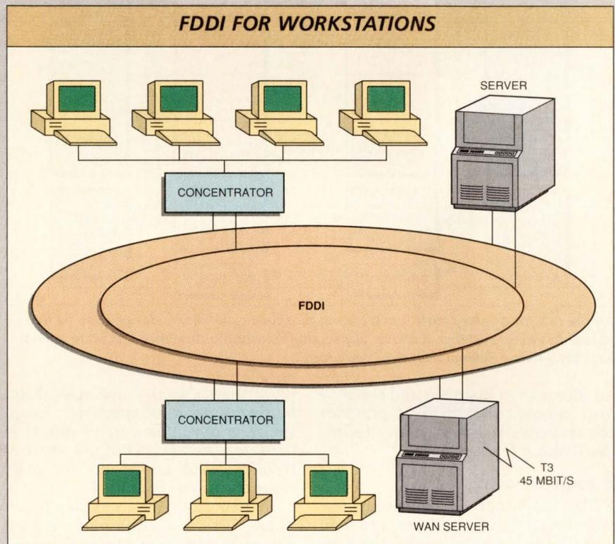
**The cost of implementing FDDI links can be brought in line with typical workstation budgets by opting for a single-attach link. Each workstation shown is linked to the network by a single fiberoptic cable. The network is implemented as two redundant fiberoptic cables, providing fault tolerant capabilities.**
