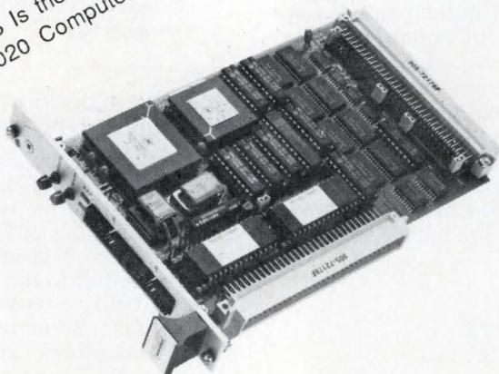
Yes, think small. And simple. And cost-effective. Single-high VMEbus computer modules offer no-nonsense solutions to your industrial control requirements while mounting in either single-high or double-high VME chassis.
