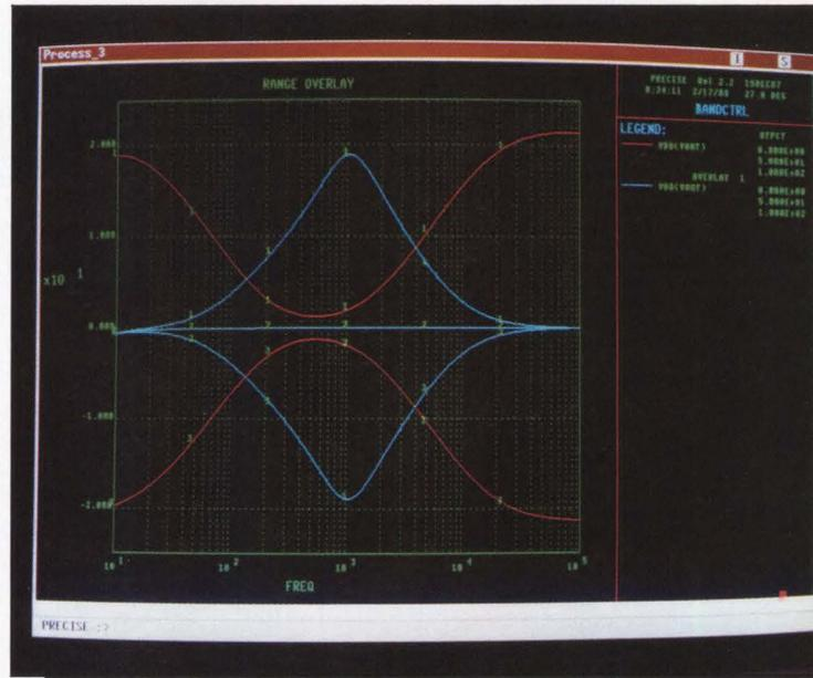
*Most analog simulators plot values in a single domain, such as time or frequency. Mixed domain analysis lets the designer view two or more domains in one plot. This Precise simulator plot of gain dB vs. frequency for a tone control circuit shows mixed-domain analysis, which varies frequency and varies the base, mid-range and treble potentiometers from boost to cut.*
