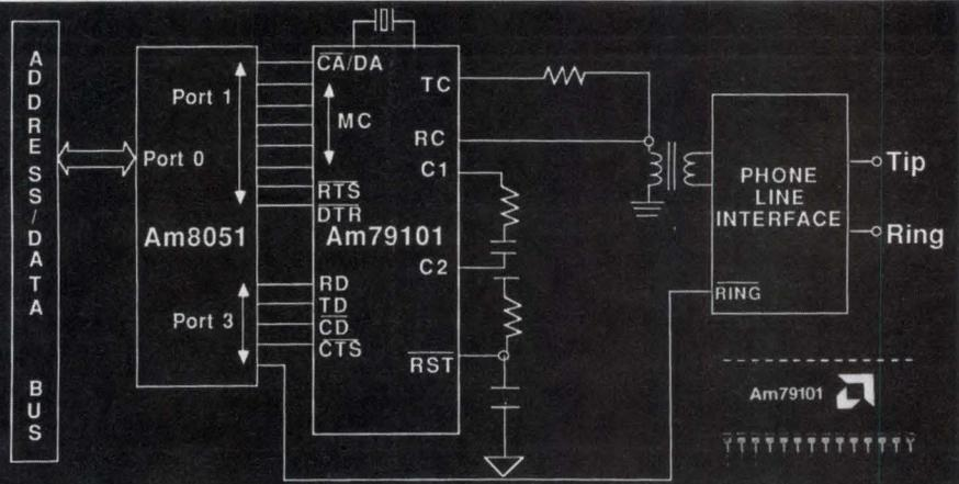
dem chip features digital signal processing architecture. The device is available in 28-pin plastic leaded chip carrier and 28-pin plastic and ceramic dual in-line packages.
