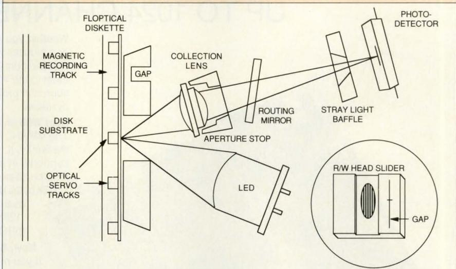
*In Insite's floptical servo system, an infrared LED shines through a hole in the read/write head to reflect an image of the servo tracks through an aspherical collection lens onto a quad-element photodetector.*
