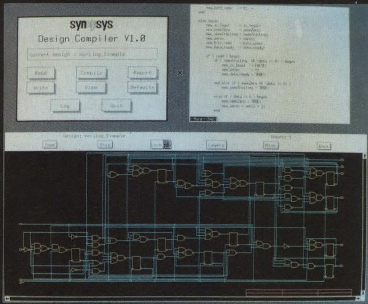
**The HDL Compiler from Synopsys provides logic synthesis from the Verilog hardware description language. An optimized, gate-level net list can be automatically generated from a register-transfer-level description in Verilog.**
