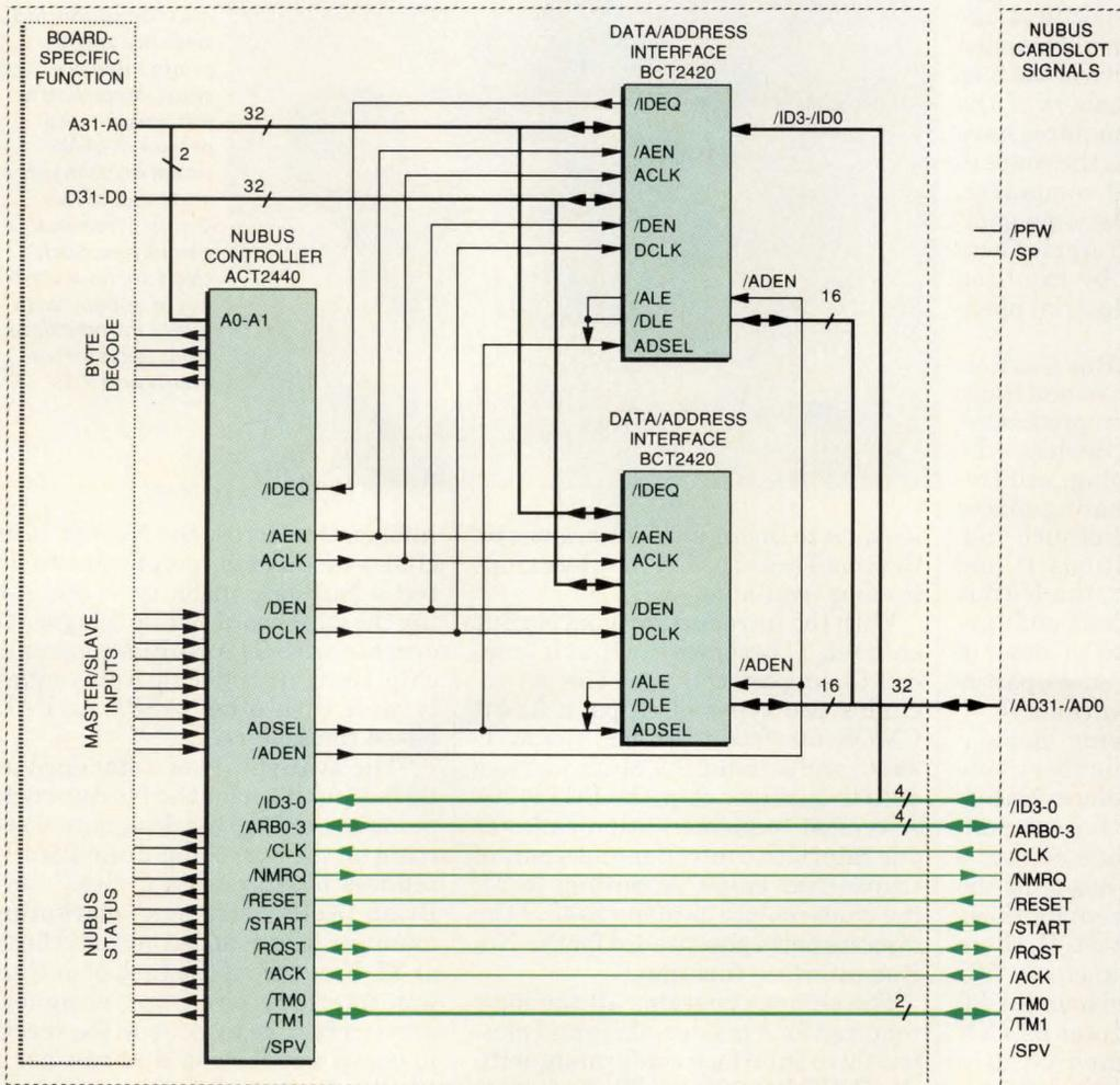
*In the Texas Instruments implementation of the NuBus interface, the controller chip directly interfaces with all the control signals on the NuBus backplane. Address and data lines are handled by the transceiver chips. Each transceiver has three 16-bit I/O ports and an on-chip comparator for backplane and slot identification.*
