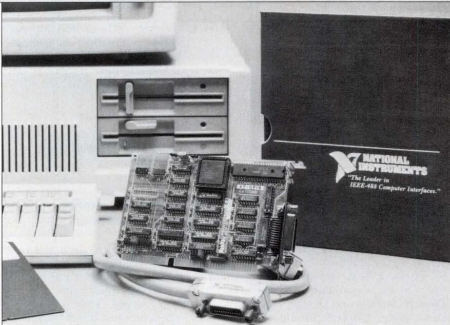
sible high-speed, burst-mode direct memory access (DMA) transfers, 1-Mbyte/s GPIB reads, 700-kbyte/s GPIB writes and 320-kbyte/s GPIB commands. The PC takes advantage of byte-to-word packing and unpacking circuitry in the ASIC to communicate with the IEEE-488 bus in full 16-bit mode, rather than 8-bit bytes, halving the data transfer overhead and PC I/O channel utilization time.
