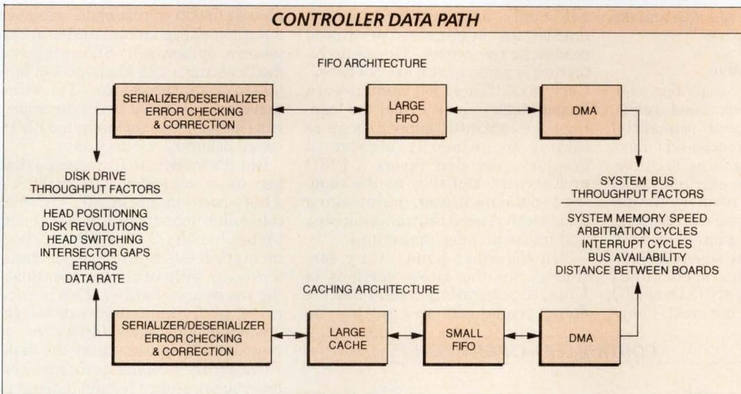
Each step in the data path between disk and system introduces latencies and overhead. The key to performance is the decoupling of the disk from the system to overlap operations. A high-performance controller, whether FIFO or RAM-based, will interface with the disk and bus at the peak rate they'll allow and will offer sustained performance equaling the disk drive rate.
