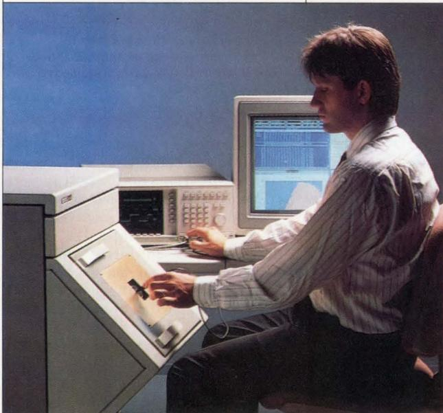
The first IC prototype tester to offer a true tester-per-pin architecture, the HP 82000 from Hewlett-Packard has been developed for designers with extensive characterization needs. Priced at around \$3,000 per pin, the system features a 200-MHz test rate and a  $\pm 250$ -ps system skew specification.
