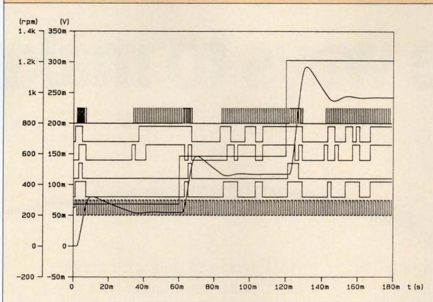
The Saber/Cadat mixed-mode simulator (a merger of Analog's Saber analog simulator and HHB Systems' Cadat digital simulator) provides the means for mixing analog and digital in the same simulation and for simulating mechanical as well as electronic functions. This printout displays both digital and analog waveforms for a motor speed controller, with an analog output waveform overlaying the digital control signals to show how the digital signals generate the analog signal.
