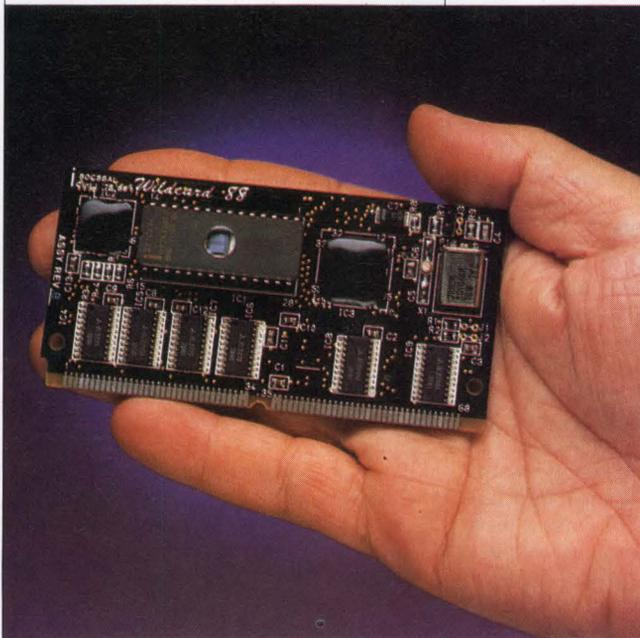
*At only 2 x 4 in., the Wildcard 88 holds all the core logic of an IBM PC XT mother board, letting OEMs incorporate DOS functionality into a wide range of intelligent systems. A CMOS 80C88 processor and an integrated peripheral controller chip are mounted directly on the board and encased in epoxy.*
