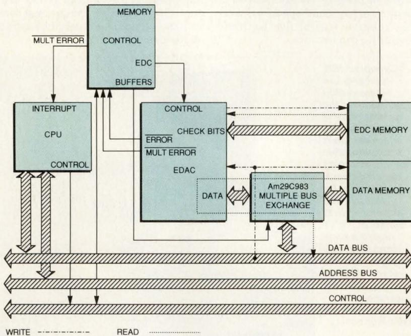
Advanced Micro Devices uses its 29C660 error detection and correction circuit (EDAC) in a flow-through configuration. In such an arrangement, the EDAC can correct any single-bit memory error before it reaches the CPU, but at the expense of slower memory access time.
