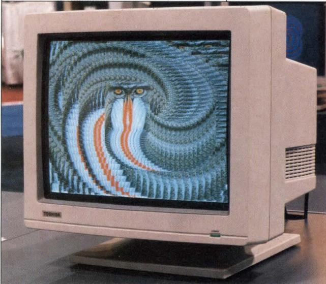
*Flat and square monitors such as Toshiba's 21-in. FS give the user a slightly larger viewing area and less corner distortion than do curved faceplate monitors. The 64-kHz, 1,280- x 1,024-pixel monitor is due out by year-end. A multiscanning version, ranging from a 1,024- x 768- to a 1,280- x 1,024-pixel resolution, will be available in early 1989.*
