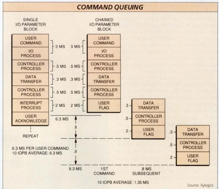
*By queuing commands on-board, an intelligent controller can minimize time-consuming host interrupts and let commands be manipulated to minimize overhead. Here, chained I/O parameter blocks (IOPBs) reduce the 10-IOPB average overhead from 6.3 to 1.35 ms.*
