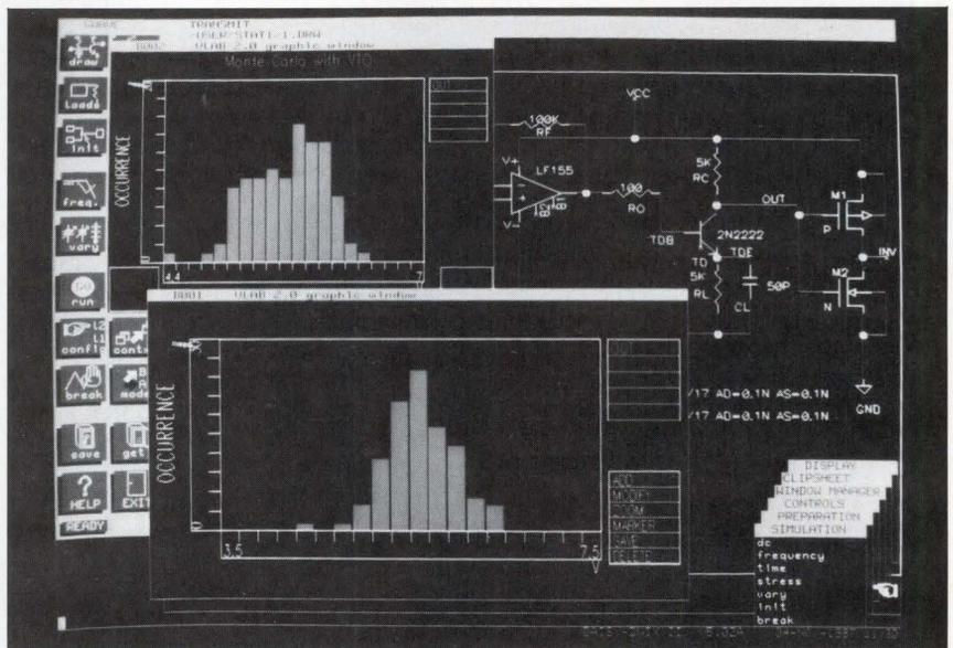
Monte Carlo analysis can be used to predict manufacturing yields by determining the possible spread of outputs based on various combinations of part values. Information is frequently displayed using bar charts, as shown in this display from the Virtual Lab analog design environment from Daisy Systems.
