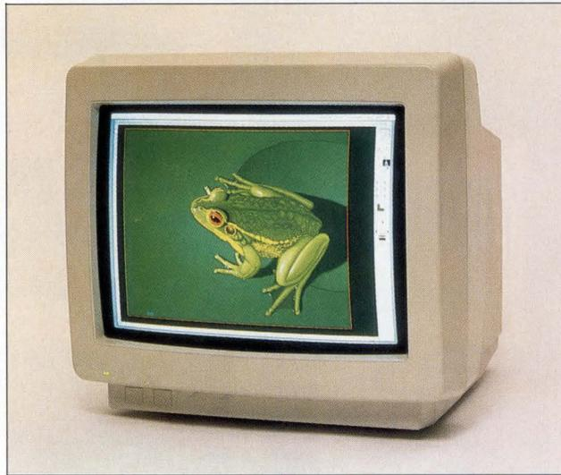
One of the latest members of Mitsubishi's Diamond Scan family, the 20 L is the first 20-in. (19-in. viewable) monitor capable of auto-tracking from 30 to 64 kHz. A microprocessor-based digital scan memory mode automatically fine tunes up to 20 discrete combinations of horizontal and vertical display settings.
