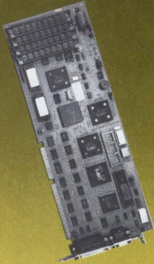
For industrial or any other demanding applications where you need a fast IBM®AT™ compatible computer. Use the TMI N286S/16-1 to get 16 MHz clock rate, and up to 4 megabytes of high speed on-board memory with effective zero wait state.
