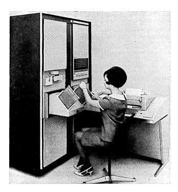
Operator compares unkown module with reference module at console of the digital logic module comparison test system.
