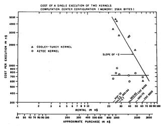
Fig. 4. Estimated cost of a single execution of the AZTEC and the Cooley-Tukey kernels on a typical computation center configuration. This system assumes about 2 million bits of storage, 8 tapes, about 500 million bits of disk storage, a line printer and a card reader. The machine costs indicated along the abscissa reflect the large base cost of this configuration.
