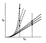
Fig. 8 The addition of a series resistance at the base causes the current from the previous circuit to distribute more evenly.
