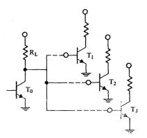
Fig. 4 Output of a logic circuit "fanned out" to three inputs.
