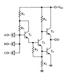
Fig. 11 DTL circuit with higher noise margin and current gain.
