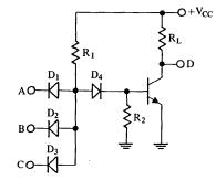
Fig. 10 Diode-transistor logic circuit.
