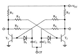
Fig. 29 Conventional center point triggered flip-flop.
