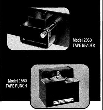
We're mostly mechanical but your control logic will think we're digital. How come? . . . Your logic can talk to us on "digital terms" because we don't use any timing cams or clutches like motor driven equipment. We use a simple ratchet drive, powered by solenoids, to move tape. Even our solenoids are like solid-state components—they require no lubrication and have virtually an infinite life.
