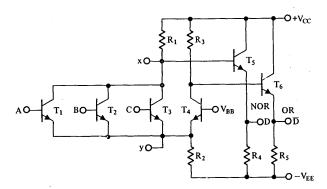
Fig. 19 Current mode logic circuit with level shifting.
