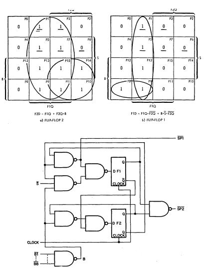
Fig. 7 (a, b & c) D Flip-flop logical mechanization.
