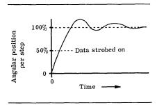
The data is strobed midway between steps, eliminating the variation in motor settling position as a factor in byte-to-byte jitter. However, in many applications as previously mentioned, it is satisfactory and less expensive to omit the use of the encoder at slower data rates and lower packing densities where the stepper has time to settle or where a mechanical damper is provided.
