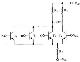
Fig. 18 Current mode logic circuit.
