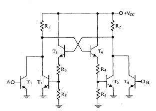
Fig. 28 Resistor coupled flip-flop with increased loop gain.
