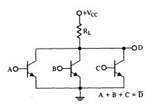
Fig. 1 Direct coupled parallel gate NOR circuit.
