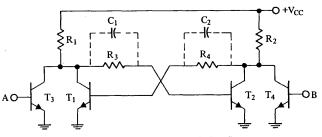
Fig. 27 Resistor coupled flip-flop.
