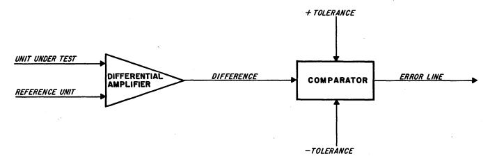
Fig. 2 Comparison circuits of the test system.
