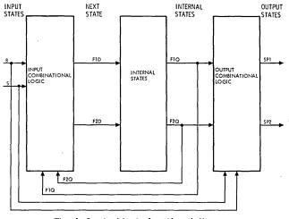
Fig. 4 Control logic functional diagram.
