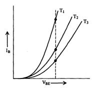
Fig. 5 Differences in the base-emitter characteristics of transistors in DCTL circuits cause an effect called "current hogging."
