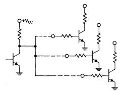
Fig. 7 Output of a logic circuit fanned out to 3 RTL inputs.
