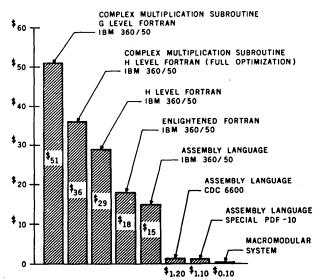
Fig. 6. Estimated cost per execution of a three-dimensional Fourier transform with a lattice size of  $64 \times 64 \times 64$ . This size problem requires about 2 million executions of the Cooley-Tukey kernel. Again the "down payment" required is suggested by the abscissa.
