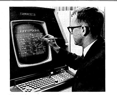
Using a light pen, an engineer designs an electronic circuit on the screen of a new UNIVAC graphic display subsystem which utilizes a digital deflection technique. From a number of component symbols shown in the upper part of the screen, the engineer can select those components he needs to construct the circuit on the grid provided by the system.
