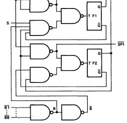
Fig. 9 (a, b & c) T Flip-flop logical mechanization.
