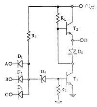
Fig. 14 Diode-Zener-diode-transistor logic circuit.
