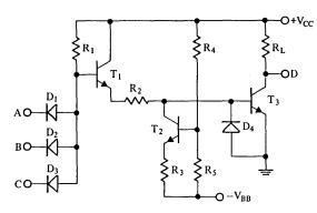
Fig. 13 Variable threshold logic circuit.
