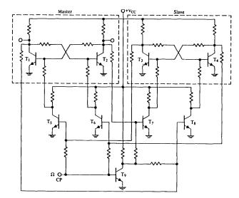
Fig. 30 Center point triggered master-slave flip-flop.
