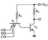
Fig. 16 Integrated form of TTL circuit.
