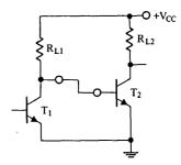
Fig. 3 DCTL stages in cascade.
