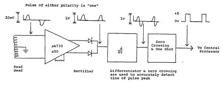
Fig. 2 NRZ Encoded Tape Playback System.
