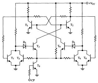
Fig. 31 Center point triggered charge control flip-flop.
