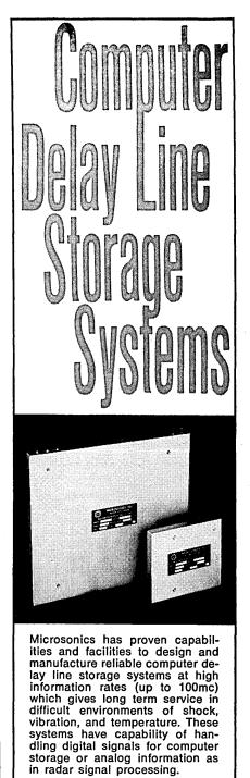
Ultrasonics computer storage lines, using fused quartz or zero T.C. glass, represent an ideal medium for high-speed computer storage up to 20mc rates.
