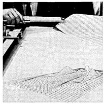
**CALCOMP THREE-D** (Perspective drawing software package) This program is a set of FORTRAN subroutines for use with any CalComp digital plotting system to produce perspective drawings of surfaces. It can also generate stereoscopic views of surfaces, and, with CalComp Model 835 microfilm plotter, can produce animated films. Easy to use, flexible and economical, THREE-D can be applied to such fields as marketing, engineering, toolmaking and designing.
