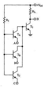
Fig. 15 Discrete form of TTL circuit.
