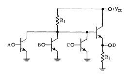
Fig. 20 Complementary transistor logic circuit.
