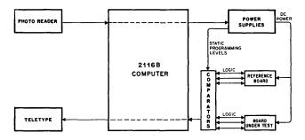
Fig. 1 Block diagram of the digital logic module test system.
