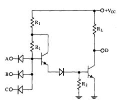
Fig. 12 DTL circuit with output stage.
