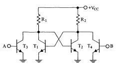
Fig. 26 Direct coupled flip-flop.
