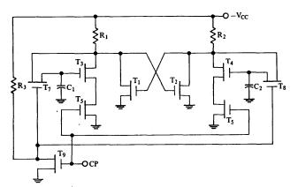
Fig. 32 Center point triggered flip-flop circuit employing field effect transistors.
