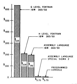
Fig. 5. Estimated cost per day of execution of the AZTEC kernel for each ten beds at 500 samples per second per bed. A time-shared system is assumed with no penalty for system overhead. The abscissa indicates crudely the "down payment" necessary to obtain the first execution.
