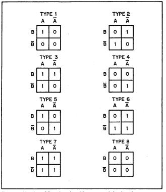
Fig. 1. Truth tables for the 16 types of logic elements.
