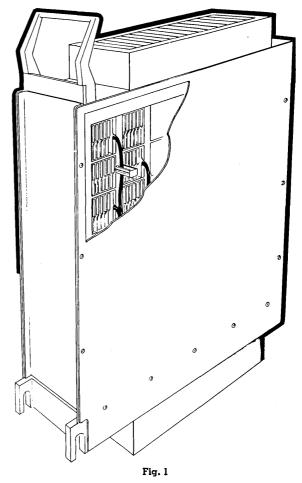
control panel can be provided that is fully accessible and maintains full EMI suppression during all computer operational modes. Cabinet penetration can be accomplished with EMI connectors located on a connector panel (Figure 2), through which all input/ouptut lines are routed. Power-line filters can be part of the connector-panel assembly or located elsewhere. Air intake and exhaust ports are shielded to allow adequate cooling while maintaining EMI integrity.
