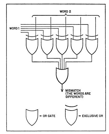
Fig. 3. The exclusive OR used in a comparator.
