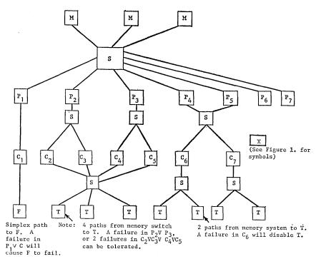
Fig. 6. Hardware structure of multiplexed computer.
