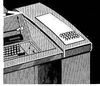
Cabinet at right of this Teletype Model 35 ASR set houses control panel and circuitry of Push Button Data Generator
