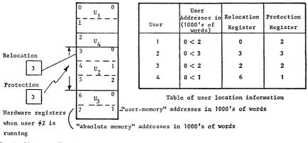
Fig. 7. Memory allocation using boundary or relocation and protection register.
