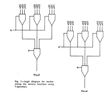
spectively. Since f(q, p) = f(p, q)the one of the simpler form is selected. With some experience in this technique, it will not be necessary to try all the possible solutions, since some Veitch diagram patterns suggest the factoring ways producing a minimal form.
