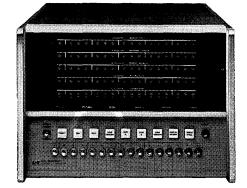
The 2115A Computer has 16-bit words, 2  $\mu sec$  cycle time, 4K memory. Price, including Teleprinter, \$16,500. Additional memory and options available.
