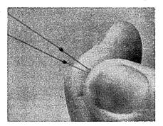
100 ohms. Applications of these diodes can be extended into the mega-Hertz range. Five separate units measuring only 0.075" diameter and 0.125" long, are offered ranging from working inverse voltage (WIV) ratings of 2000 volts to 6000 volts in 1000 volt steps. Peak surge current (8 msec.) varies from 9 amps to 3.5 amps. Computer Diode Corp., Fair Lawn, N.J.
