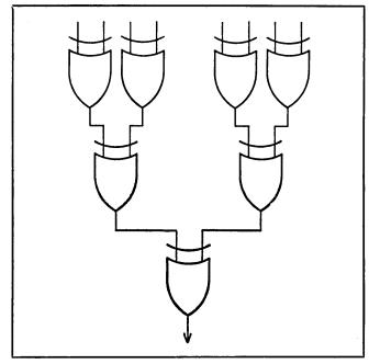
Fig. 2. The exclusion OR used to generate parity.
