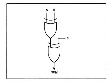
Fig. 5. The exclusive OR used to generate the sum in an adder.
