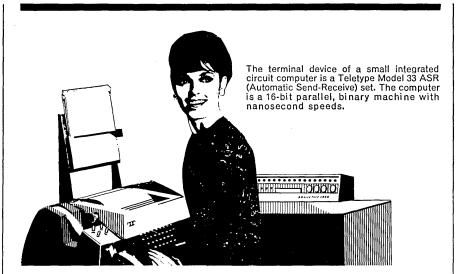
Users of a time shared computer system can contact the computer for service and inputs of all instructions, data, and plot programs through standard Teletype equipment. The computer processes the data and transmits via a Model 33 ASR set a complete plot program, including identification codes for that particular plotter and output signals for remote on-line plotting.
