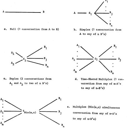
Fig. 5. Computer component switch or selection configurations.
