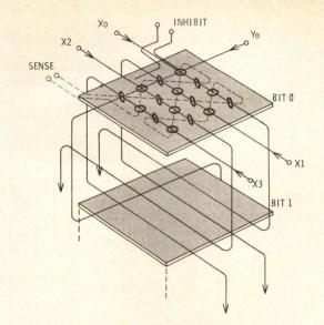
Fig. 9 Coincident-current stack wiring configuration.
