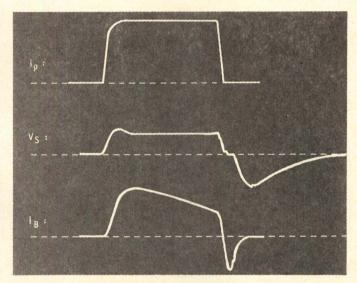
Fig. 16 Current-driven switch secondary response.
