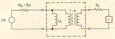
Fig. 5 Low-frequency equivalent circuit (flat-top period).
