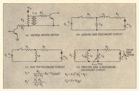
Fig. 13 Voltage-driven switch analysis.
