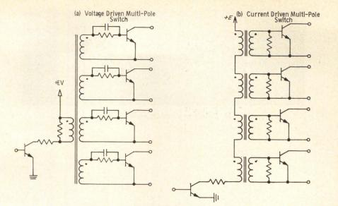
Fig. 20 Multi-pole switch configurations.
