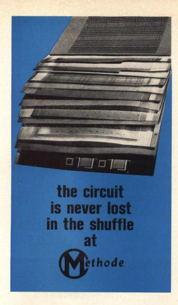
This 15-layer circuit board with multiple ground planes and signal circuits was especially designed for datamation applications.
