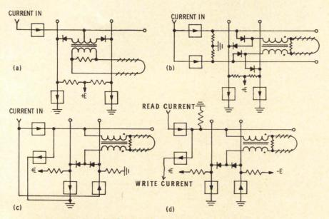
Fig. 25 Examples of transformer-diode matrices.
