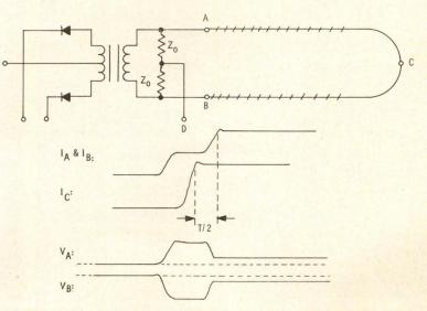
Fig. 22 Parallel line termination.
