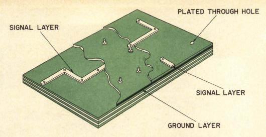
Fig. 1 Sectional view of multilayer PC board
