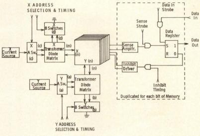
Fig. 10 Coincident-current memory system.
