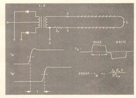
Fig. 21 Series line termination.
