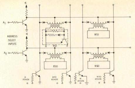
Fig. 18 Current-driven switch with turn-off drive.
