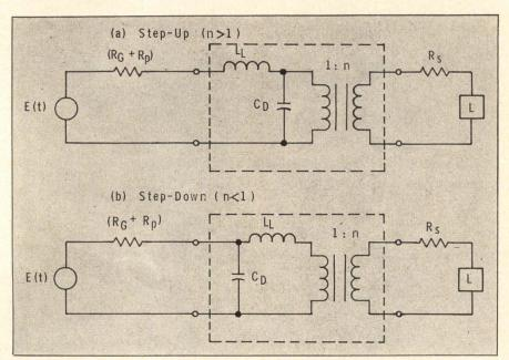
Fig. 4 High-frequency equivalent circuit (rise and fall periods).
