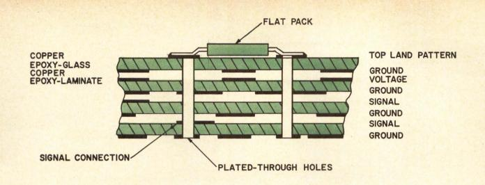
Fig. 2 Cross-sectional view of multilayer PC board
