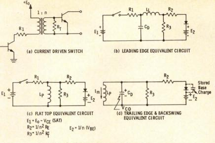
Fig. 15 Current-driven switch analysis.
