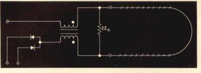
Fig. 23 Balun or common mode line coupling.
