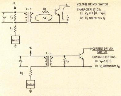
Fig. 12 Voltage- and current-driven switches.
