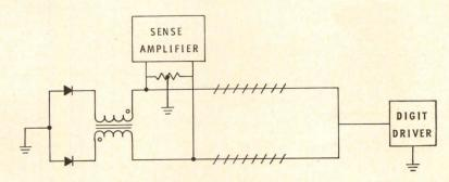
Fig. 28 Common sense-digit line with current splitting transformer.
