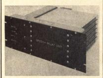
The DDI Analog Delay System imposes precise time delay of analog information using combined analog and digital techniques. System illustrated delays speech 60 msec. Longer delays are achieved by using additional digital delay lines. Applications include sonar data processing, speech and analog data transmission and autocorrelation.
