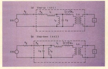
Fig. 2 Simplified equivalent circuits for step-up and step-down cases.
