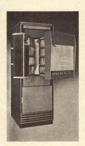
words - 1.8 usec core memory - 0 to 12 v. logic levels - standard rack mounting and front access to the entire computer.
