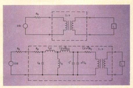
Fig. 1 Pulse transformer and general equivalent circuit.
