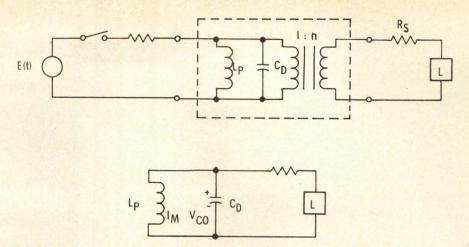
Fig. 6 Fall and backswing equivalent circuit (primary open-circuit).
