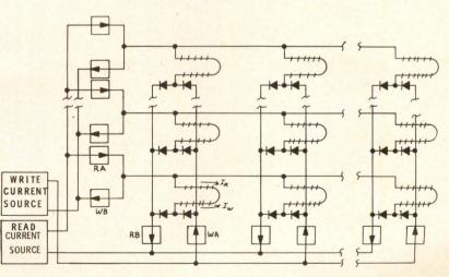
Fig. 11 Diode matrix with floating switches.
