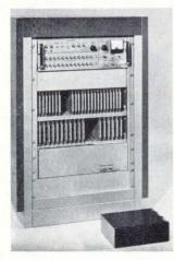
Two Fabri-Tek 4,096 x 12 memories. The larger one is the 1 usec. Series MF.Dwarfed is the 4 usec. Series MC compact memory. Of course, the big one has integral power supply, self-test, and many other features.
