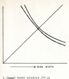
Fig. 2 Variations in electrical characteristics with change in bus bar width.
