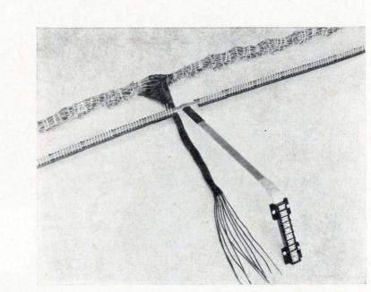
Fig. 1 Comparison of 10-layer bus assembly with equivalent wire harness.
