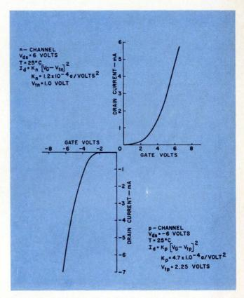
Fig. 2 Transfer characteristics of n-channel and p-channel MOS devices.
