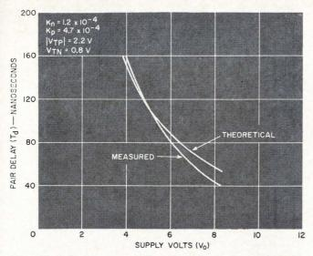
Fig. 12 Pair-delay as a function of supply voltage for circuit of Fig. 6.
