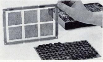
Memory stack consists of  $64 \times 64$  core arrays mounted on rugged, laminated frames. Wide temperature cores are used. Planes can be potted.
