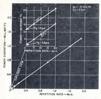
Fig. 8 Power dissipation as a function of repetition rate for the set-reset flip-flop of Fig. 6. (All data was taken using RCA's developmental semi-integrated MOS transistor circuits.)
