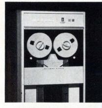
The **D 3030** writes and reads all three densities (800, 556 and 200 cpi) at 75 ips tape speed. Push-button selection of 60,000, 41,700 and 15,000 cps data transfer rates. Either 7-track or 9-track format. Vacuum column tape buffers, semi-automatic tape threading, front access to all electronics, and many other advanced features. Bi-directional start and stop times of 5 ms and 11/2 ms, respectively.
