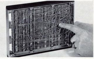
Wrapped wiring of circuit module terminations eliminates connectors, increases reliability, and yet retains easy replacement features.
