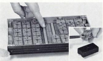
All heat-producing components mount directly to heat sinks. Inset shows how circuit modules each contain individual heat conductors.
