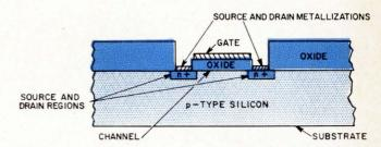
Fig. 1 Cross-section of n-channel MOS transistor.
