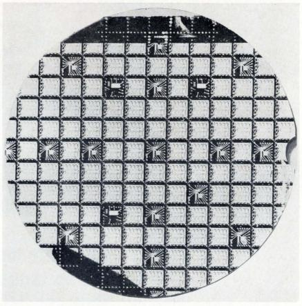
Monolithic memory chips are fabricated on silicon wafers, eight-thousandths-of-aninch thick. The spider-like designs interspersed throughout the wafer are test areas which enable IBM to test the chips for various electrical parameters while they are being fabricated.
