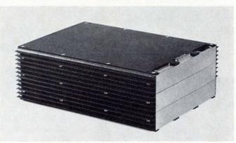
This typical Series MC memory is  $7.25'' \ge 9.375''$  and weighs approximately 8 pounds. Max. power dissipation is less than 48 watts. Operating temperature range is  $-55^{\circ}$  to  $71^{\circ}$ C.
