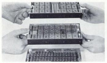
System is composed of stacked modules. Number of modules depends upon memory capacity. This typical system has 3 modules and a capacity of  $4,096 \ge 12$ .
