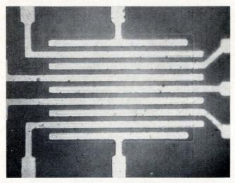
Fig. 17 Geometrical configuration of semiintegrated MOS unit (four transistors).
