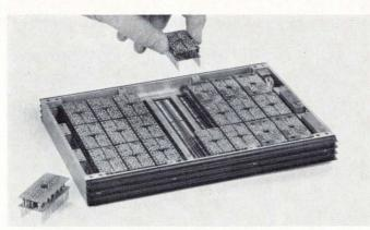
Economical circuit modules, mated directly through a parentboard assembly can be potted with light-closed cell foam if desired.
