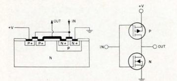
Fig. 16 MOS micropower integrated circuit using diffusion techniques.
