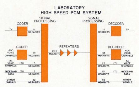
Block diagram illustrates Bell Telephone Laboratories' experimental high speed pulse code modulation system designed to transmit 224 million bits of information a second over coaxial cable. It can transmit simultaneously voice, television, and data. This diagram shows some of the combinations of these signals possible.
