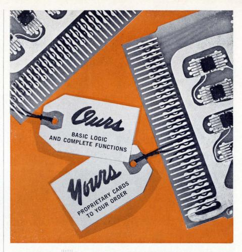
**EECOLOGIC** is a **product** of Engineered Electronics Company consisting of basic logic cards such as flip flops, NAND gates, drivers, and other logic, plus a line of logic function cards such as counters, shift registers, full adders, and decades.
