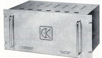
Model 4700 Magnetic Code Converter utilizes magnetic cores and micrologic circuitry to provide readouts of arbitrary binary functions. The unit accepts a 12-bit "argument" as an *input* and produces a parallel 12-bit "function" as an *output*. A single *read* command is required to initiate the entire code conversion operation. *Read* commands may occur as often as once *every three microseconds!* Outputs appear *less than 0.8* microseconds after the start of the *read* command.
