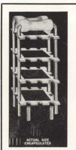
Fig. 24 Electra Mfg. Co. manufactures thin-film metal resistive microelements on ceramic substrates. As shown here, the ceramic wafers can be stacked and combined with capacitors and active elements. Resistive values from 10 to 100-thousand ohms are standard with a resistive tolerance of 2% and a temperature coefficient of 100 parts per million per degree C. The wafers are approximately 5/16" square and 0.010" thick.
