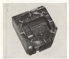
SPACE DATA AUTOMATION SYSTEMS are solid state systems designed to make possible receipt of technical data from unmanned spacecraft scientific experiments, and to act on command sequences sent to the spacecraft. The 3C/SDAS allows unmanned spacecraft to vary their command sequences by internally pre-programmed sequences of events, external signals sensed by experiments, or by radio commands. SDAS systems operate on less than 1 watt of power.
