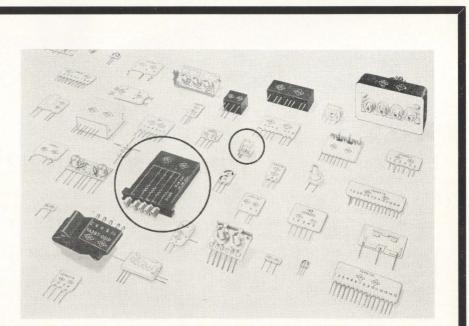
$13/32'' \times 13/32'' \times 5\%''$ ; and a high reliability arc-suppression circuit (the flat package shown circled in the photograph) which is potted in a case,  $11/2'' \times 21/8'' \times 1/4''$ . This R-C suppressor contains 4 resistors and 4 capacitors and was built for a minimum of 20,000 hours of continuous operation. Flip-flops and other digital circuits have been produced by Centralab using their PEC tech-
