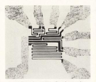
resistance change of over 0.57%. Shown here is a close-up of a NOR gate resistor network illustrating control over line width to less than a mil.
