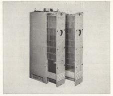
DELAY LINE TIME COMPRESSION (DELTIC) equipments are in tactical use aboard submarines, permitting extension of signal detection capabilities. DELTIC circuits digitize input signals and hold them in active storage, greatly compressing them in time for real-time signal correlation. 3C DELTIC equipment provides significant reduction in the complexity and size of signal processing equipment for application to sonar, radar, telemetry and audio spectrum analysis.
