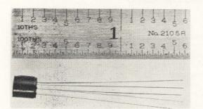
Fig. 5 Numerous diode, resistor, capacitor combinations are available in TO-18 or TO-5 packages from MicroSemiconductor. These integrated circuits are said to provide the optimum in microcircuit performance, reliability, and cost. The circuits operate over broad current and voltage ranges, frequencies in excess of 20 megacycles and over a temperature range of -55 to +150C. Typical circuits include input gates and flip-flop steering gates.
