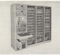
**REAL TIME COORDINATE CONVERSION COMPUTER** continually positions two eighty-five foot parabolic antennas used to track orbiting satellites and space probe vehicles from a West Coast site. The antennas, computer, and a microwave data link form the closed loop tracking system. Computer Control has also developed a Coordinate Conversion Computer now in use as part of an airborne telescope tracking system designed to photograph missiles during re-entry.
