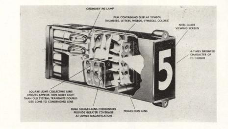
Conventionally, lenses are circular; the new lenses are basically square to permit greater usable lens area within the limited space. This increase in lens size utilizes two factors almost equally in quadrupling brightness. First, brightness is doubled because the larger lenses collect twice the amount of light from source. The second doubling of brightness takes place inversely through an approximate 50% reduction in magnification requirements.
