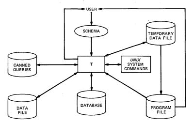
Fig. 2-Communication paths for the primitives module.
