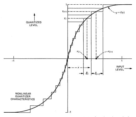
Fig. 2—Exemplary nonlinear quantizer; arbitrary f(x) and number of quantization levels.
