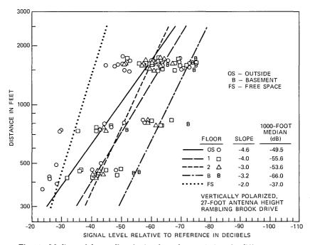
Fig. 14—Medians of the small-scale signal envelope variations for different measurement locations plotted versus distances between the locations and the van antenna. The locations are inside and outside a house on Rambling Brook Drive.
