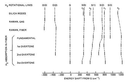
Fig. 4—Correlation diagram of Raman and fundamental and overtone absorption spectra of  $H_2$  in silica. Frequencies are measured with respect to the Q-branch frequency. The gas-phase  $H_2$  rotational structure<sup>10</sup> and silica tetrahedral vibrations<sup>9</sup> are shown.
