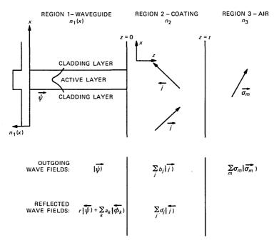
Fig. 1-Two-dimensional model used in calculation.
