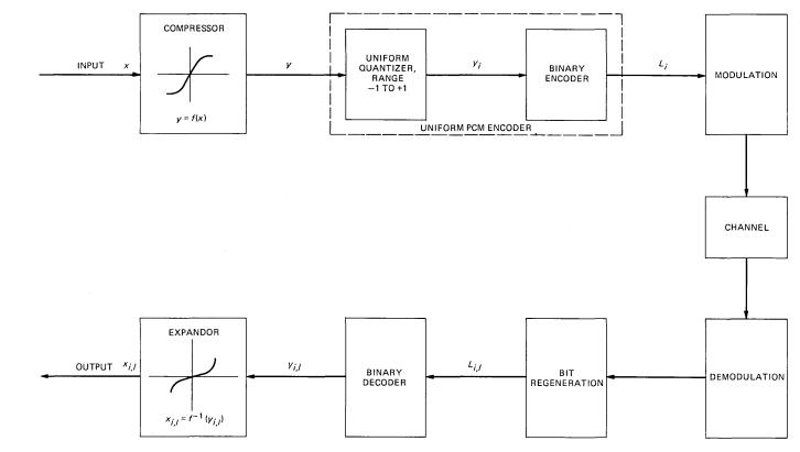
Fig. 1—The basic companded PCM system.
