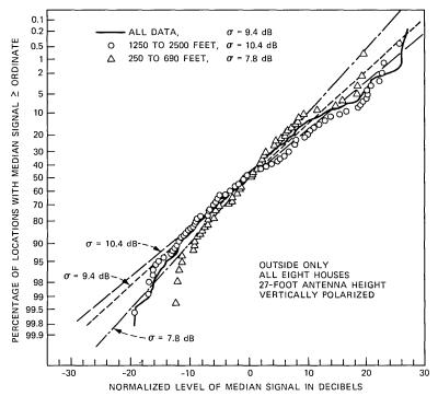
Fig. 27—Cumulative distributions of the medians of the small-scale signal envelope variations for outside locations after the trend values for the solid regression line in Fig. 22 are subtracted out.
