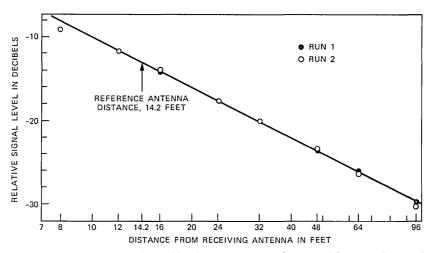
Fig. 5—Relative received signal level as a function of distance, *d*, between the signal source on top of a building and the receiving antenna mounted on the 27-foot van mast shown in Fig. 2. The measurements were made in an open area free of obstructions.
