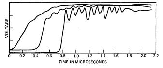
Fig. 4-Typical shock waves on transmission line of Fallside et al.
