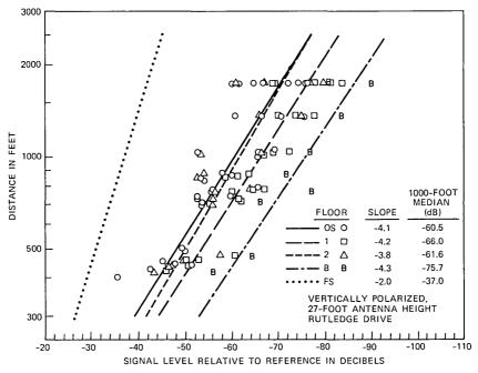
Fig. 21—Signal envelope medians and regression lines for the house on Rutledge Drive similar to those in Fig. 14.
