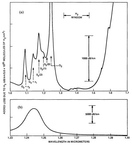
Fig. 1—First-overtone loss spectrum at room temperature of  $H_2$  in silica fiber: (a) Entire spectrum of the first overtone, measured in a 10m single-mode fiber;  $\nu_1$  and  $\nu_3$  are silica vibrations;<sup>9</sup> (b) Expanded view of the most intense band, the Q branch, measured on 2.3m of multimode fiber.
