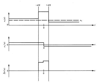
Fig. 3-Details of index step for an asymmetric waveguide.
