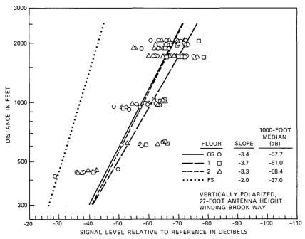
Fig. 15—Signal envelope medians and regression lines for the house on Winding Brook Way similar to those in Fig. 14.
