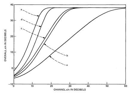
Fig. 14—Effect of diversity on Rayleigh fading channels. Theoretical cuves of overall s/n against channel s/n for -17 dB input power, NCFSK modulation, bit scrambling: (a) no diversity; (b) ISCD (M = 2); (c) IMRCD (M = 2); (d) ISCD (M = 4); and (e) IMRCD (M = 4).
