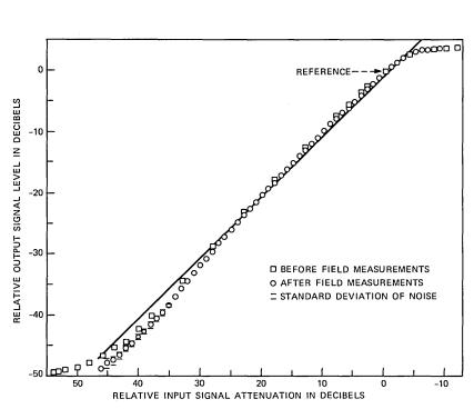
Fig. 4—Input-to-output characteristic of the modified receiver. The data from after the field measurements include the analog-to-digital conversion in the digital-storage oscilloscope. The data from before the field measurements were measured with an analog voltmeter at the output of the linear detector.
