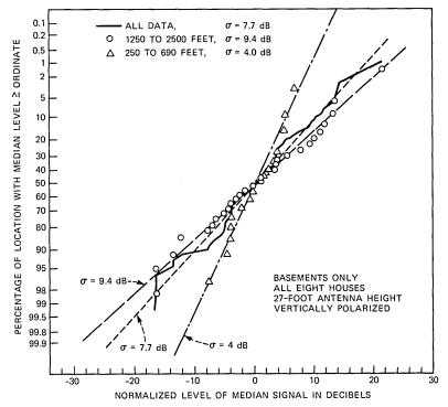
Fig. 29-Cumulative distributions for basement locations similar to those in Fig. 27. The regression trend removed was the solid line in Fig. 25.
