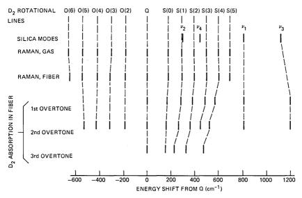
Fig. 5—Correlation diagram of Raman and overtone absorption spectra of  $D_2$  in silica. Frequencies are measured with respect to the Q branch. The gas-phase  $D_2$  rotational structure<sup>10</sup> and silica tetrahedral vibrations<sup>9</sup> are shown.
