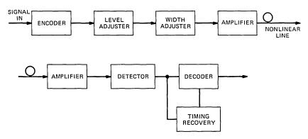
Fig. 9—Pulse code modulation transmission system employing solitons.
