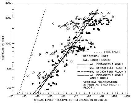
Fig. 23—Signal envelope medians and regression lines for the data from the first floors for all eight houses similar to those in Fig. 22. In addition, the regression line is included for all the first- and second-floor data combined.
