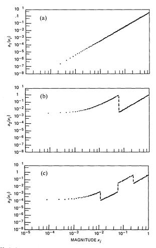
Fig. 4—Variation of  $a_l(x_i)$  as a function of  $x_i$  for 8-bit  $\mu$ -law PCM,  $\mu = 255$ . The subfigures a through h apply for a single bit error in the msb (l = 1), the next msb  $(l = 2), \dots$ , lsb (l = 8), respectively.
