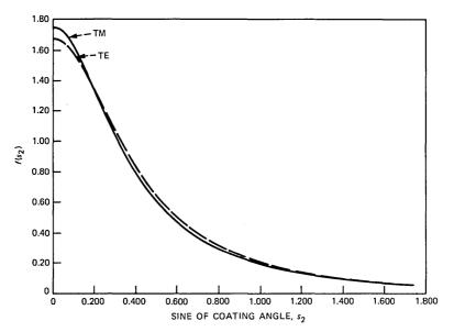
Fig. 2—The k-space wave functions of TE and TM modes. Solid curve is TE mode and dashed curve is TM mode.
