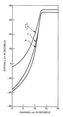
Fig. 8—Gaussian channel. Speech simulation curves of overall s/n against channel s/n for CPSK modulation (a) -17 dB input power, MDC; (b) -17 dB input power, FBC; (c) -40 dB input power, MDC; and (d) -40 dB input power, FBC.
