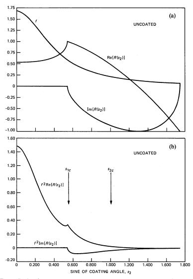
Fig. 5—Real and imaginary parts of (a)  $R(s_2)$  for h = 0, and (b)  $R(s_2)|f|^2$  for h = 0.  $f(s_2)$  is shown for comparison.
