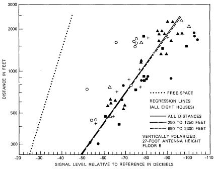
Fig. 25—Signal envelope medians and regression lines for the data from the basements for the six houses that have basements. The figure is similar to Fig. 22.
