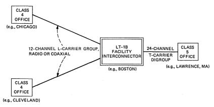
Fig. 10-LT-1 facility connector end-office trunking.
