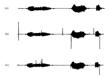
Fig. 11— $\mu$ -law PCM speech waveforms for mobile radio channels, nondiversity CPSK, vehicular speed 30 mph, -40 dB input power level, 25-dB channel s/n, and no bit scrambling: (a) original speech; (b) recovered speech with FBC (point A in Fig. 10); and (c) recovered speech with MDC (point B in Fig. 10).
