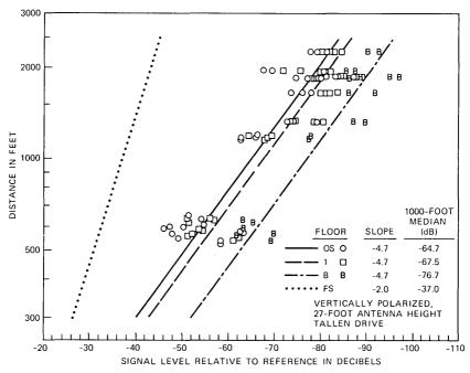
Fig. 20—Signal envelope medians and regression lines for the house on Tallen Drive similar to those in Fig. 14.
