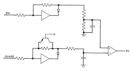
Fig. 5-Signal receiver.
