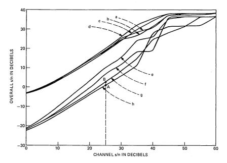
Fig. 10—Mobile radio channel. Speech simulation curves of overall s/n against channel s/n for nondiversity CPSK modulation with a vehicular speed of 30 mph. Curve labels are as in Fig. 9.
