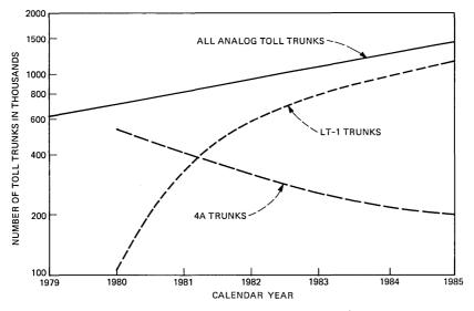
Fig. 1—Long-haul, toll network, analog trunk estimate.
