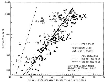
Fig. 22—Medians of the small-scale signal envelope variations for different measurement locations plotted versus distances between the locations and the van antenna. The locations are outside of the eight houses. Signal levels are with respect to 0 dB at the signal reference. Regression lines are drawn for all the outside data from all eight houses for all distances and for two subsets of the outside data.
