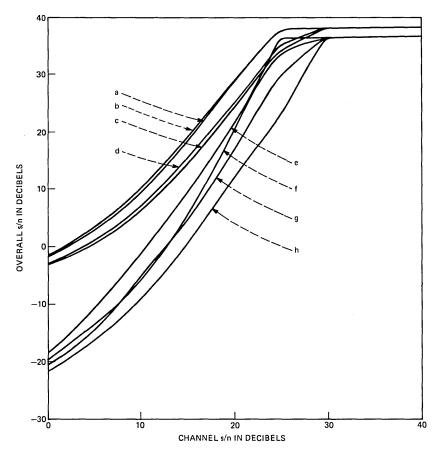
Fig. 13—Mobile radio channel. Speech simulation curves of overall s/n against channel s/n for CPSK modulation. The vehicular speed is 30 mph, with 2-branch diversity and bit scrambling employed: (a) -17 dB input power, IMRCD, MDC; (b) -17 dB input power, IMRCD, FBC; (c) -17 dB input power, ISCD, MDC; (d) -17 dB input power, ISCD, FBC; (e) -40 dB input power, IMRCD, MDC; (f) -40 dB input power, ISCD, FBC; (g) -40 dB input power, ISCD, MDC; and (h) -40 dB input power, ISCD, FBC.
