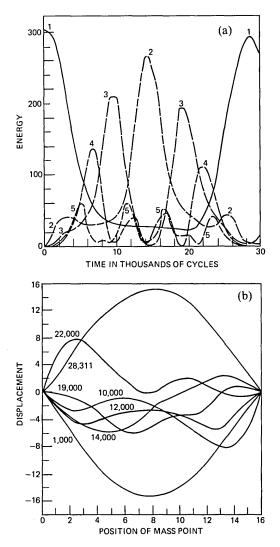
Fig. 1—(a) Energy in each of the first five modes. Initial form of string was single sine wave. Higher modes never exceed 20 units in energy. (b) Actual shape of string at various times.
