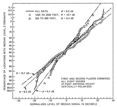
Fig. 28—Cumulative distributions for first- and second-floor locations combined similar to those in Fig. 27. The regression trend removed was the dashed and dotted line in Figs. 23 and 24.
