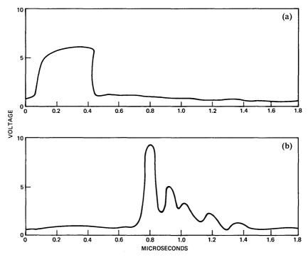
Fig. 6—Decomposition of a pulse into a finite train of solitons.
