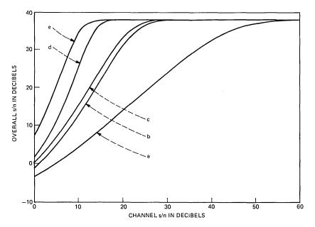
Fig. 15—Effect of diversity on Rayleigh fading channels. Same conditions as in Fig. 14, except that CPSK modulation is used.
