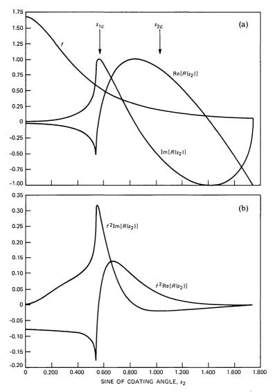
Fig. 6—Real and imaginary parts of (a)  $R(s_2)$  for h = 1/4, and (b)  $R(s_2)|f|^2$  for h = 1/4.  $f(s_2)$  is shown for comparison.
