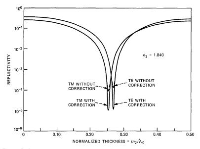
Fig. 8—Reflectivity as a function of normalized thickness for a coating index of 1.840.
