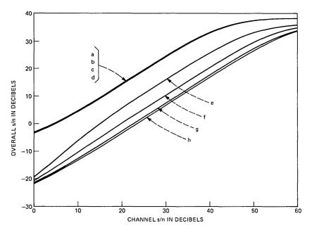
Fig. 9—Rayleigh fading channel. Theoretical curves of overall s/n against channel s/n for nondiversity CPSK modulation: (a) -17 dB input power, bit scrambling, MDC; (b) -17 dB input power, bit scrambling, FBC; (c) -17 dB input power, no bit scrambling, MDC; (d) -17 dB input power, no bit scrambling, FBC; (e) -40 dB input power, bit scrambling, FBC; (g) -40 dB input power, bit scrambling, FBC; (g) -40 dB input power, no bit scrambling, FBC.
