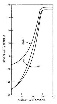
Fig. 6—Gaussian channel. Theoretical curves of overall s/n against channel s/n for NCFSK modulation (a) -17 dB input power, MDC; (b) -17 dB input power, FBC; (c) -40 dB input power, MDC; and (d) -40 dB input power, FBC.
