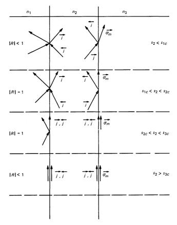
Fig. 4—The k-vectors for states involved in the calculation of  $R(s_2)$  for all values of  $s_2$ .
