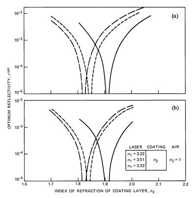
Fig. 7—Optimum reflectivity as a function of index of refraction of coating for (a) TE and (b) TM modes for laser structure shown in inset.
