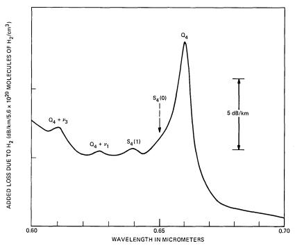
Fig. 3—Third-overtone spectrum of  $\mathrm{H}_2$  at room temperature measured on 450m of multimode fiber.
