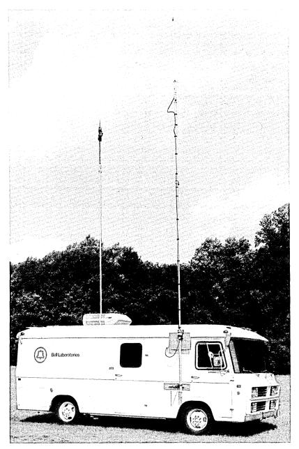
Fig. 2—The instrumentation van with the receiving antenna mast and the reference signal mast erected. The center of the four-element collinear receiving antenna is 27 feet above ground at the top of the mast mounted on the right side of the van near the front. The signal source is at the top of its reference mast mounted on the left side near the rear. The center of the signal-source dipole is also 27 feet above ground.
