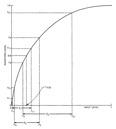
Fig. 5—The nonlinear quantizer characteristic showing how the effect of a transmission error in the second msb (l = 2) affects the amplitude of the recovered sample.
