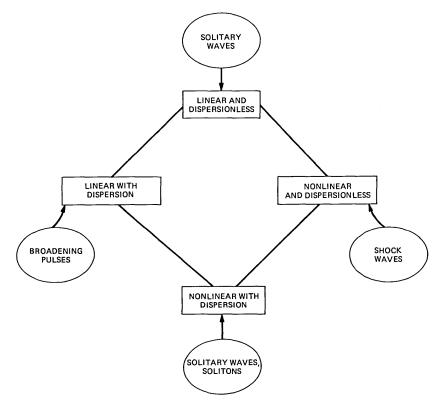
Fig. 5-Four types of wave-propagating media and the types of waves to be expected.
