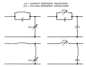
Fig. 8-Nonlinear transmission lines where solitons can propagate.
