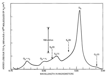
Fig. 2—Second-overtone spectrum of  $\mathrm{H}_2$  at room temperature measured on 13m of multimode fiber.
