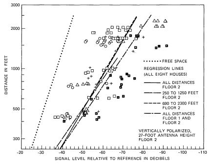
Fig. 24—Signal envelope medians and regression lines for the data from the second floors for the five houses that have second floors. The figure is similar to Fig. 22. In addition, the regression line is included from Fig. 23 for all the first- and second-floor data combined.
