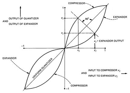
Fig. 3-Compressor and expandor characteristics.
