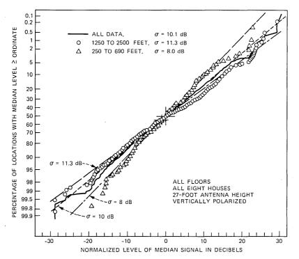
Fig. 30—Cumulative distributions for all floors and outside combined similar to those in Fig. 27. The regression trend removed was the solid line in Fig. 26.
