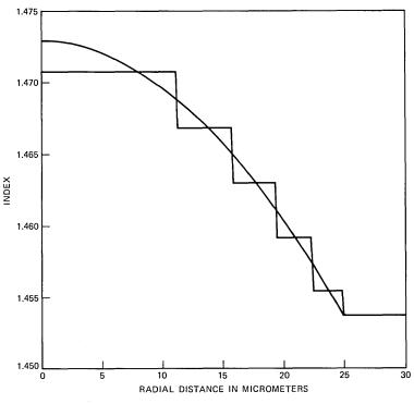
Fig. 11—A plot of a multilayered fit to an  $\alpha$  profile (NS = 5,  $\alpha$  = 1.90).
