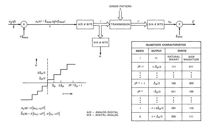
Fig. 7—Model for analyzing quantizing noise and the effects of transmission errors. The graph and table define the quantizer and two binary number representations.
