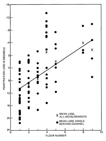
Fig. 3—Penetration loss measurements.
