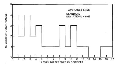
Fig. 2—Differences in level between the strongest and weakest serving channels on the same floor.
