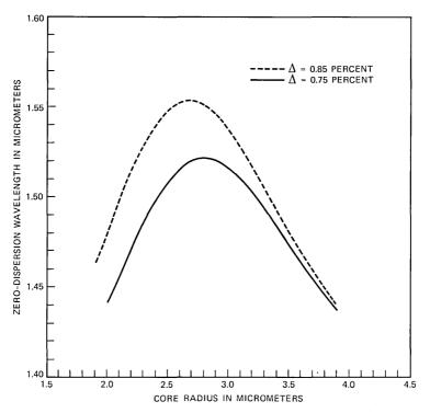
Fig. 17—Plots of computed zero-dispersion wavelength  $(\lambda_o)$  versus core radius (R) for two values of  $\Delta$ , for triangular profiles.
