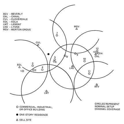
Fig. 1—AMPS Developmental Cellular System locations of 15 buildings and seven serving cell sites.
