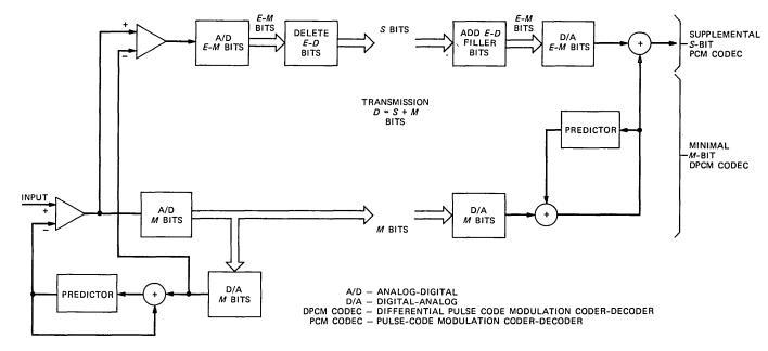
Fig. 2—Embedded DPCM encoder and decoder. *E*-bit analog-to-digital conversion is shown as a two-stage, successive-approximation process. All M minimal bits are transmitted. *S*, the number of supplemental bits transmitted, can range from 0 to E-M.
