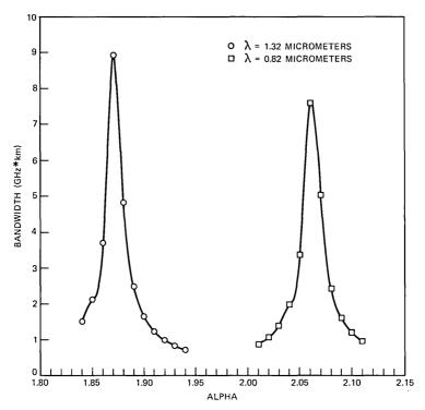
Fig. 10—Plots of bandwidth versus  $\alpha$  for  $\lambda = .82 \ \mu m$  and  $\lambda = 1.32 \ \mu m$  assuming equal excitation of modes having less than 0.1 percent power in cladding.
