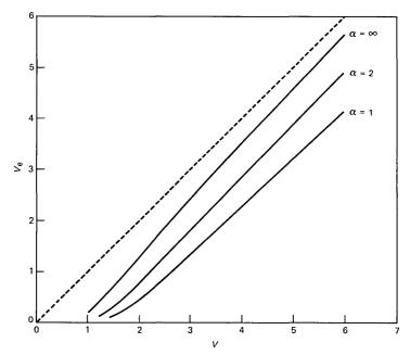
Fig. 16—Plots of  $V_e$  versus V for the  $HE_{11}$  mode of three power-law profiles. 2690 THE BELL SYSTEM TECHNICAL JOURNAL, NOVEMBER 1983
