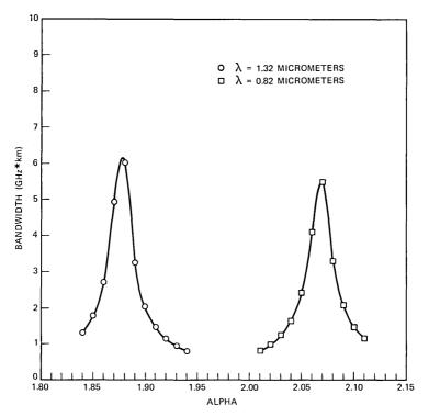
Fig. 9—Plots of bandwidth (in power-law fibers) versus  $\alpha$  for  $\lambda = .82 \ \mu m$  and  $\lambda = 1.32 \ \mu m$ , using tapered modal-power distribution.
