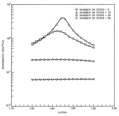
Fig. 12—Plots of bandwidth versus  $\alpha$  at  $\lambda = 1.32 \ \mu m$  for four values of NS.
