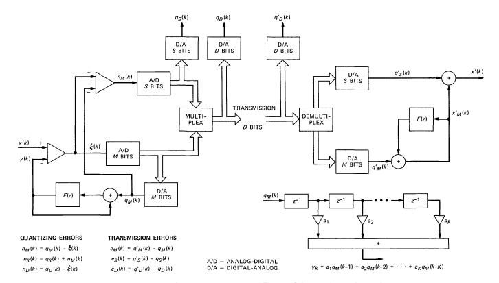
Fig. 6—The signal-processing operations of Fig. 2 and the notation used to analyze them. Three new digital-to-analog converters define signals that appear in the analysis.
