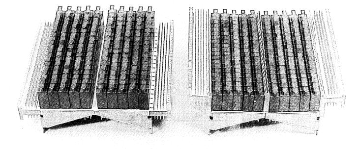
Fig. 1—Originally proposed (left) and modified (right) 309-type protected connector.
