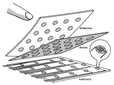
Fig. 1-Membrane switch technology.
