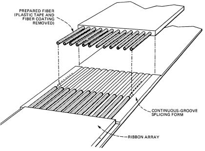
Fig. 1-Basics of a fiber-optic ribbon, continuous-groove splice.
