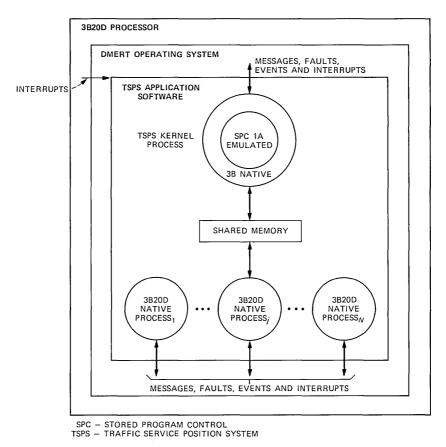
Fig. 5-TSPS No. 1B process structure.
