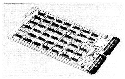
Fig. 11-Typical circuit pack for the Peripheral System Interface frame.
