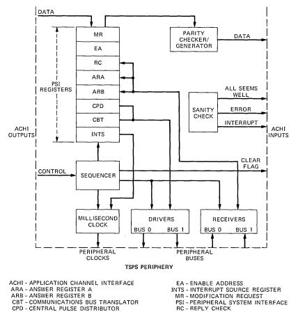
Fig. 5—Block diagram of the Peripheral System Interface circuit.
