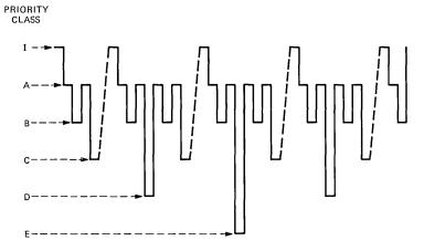
Fig. 12-TSPS No. 1B base-level, priority-class frequency.
