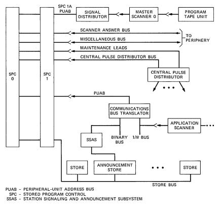
Fig. 3-Connectorized TSPS buses.
