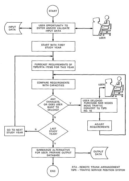
Fig. 3-Flowchart of Node Exhaust program.
