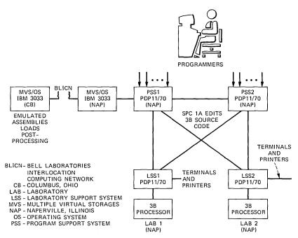
Fig. 1-Software Development System for TSPS No. 1B.
