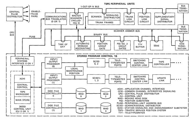
Fig. 3—The SPC 1B Processor and peripheral architecture.
