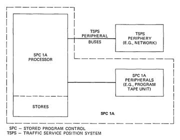
Fig. 1-Existing TSPS system structure.
