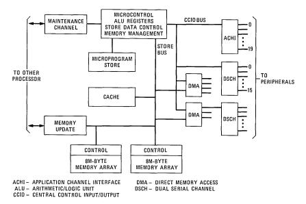
Fig. 3-3B Processor block diagram.
