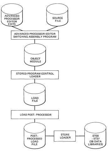
Fig. 2-Basic steps in emulated, assembly-language software generation.
