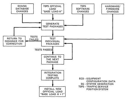
Fig. 4—TSPS integration testing.
