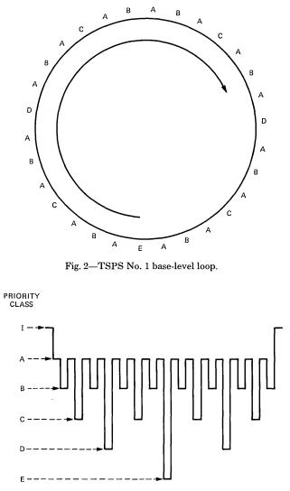
Fig. 3—TSPS No. 1 base-level, priority-class frequency.
