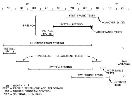
Fig. 1—Test schedule for system integration.
