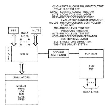
Fig. 3-Laboratory configuration for TSPS No. 1B.
