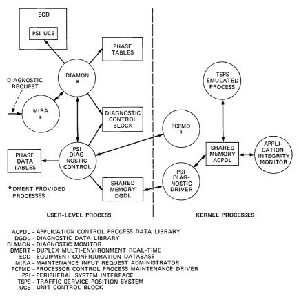
Fig. 13-Maintenance software structure for the Peripheral System Interface.
