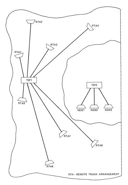
Fig. 5(b)-TSPS/RTA configuration after user move.
