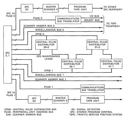
Fig. 2—TSPS No. 1 peripheral buses.
