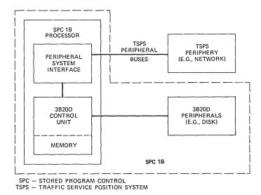
Fig. 2—TSPS No. 1B system structure.
