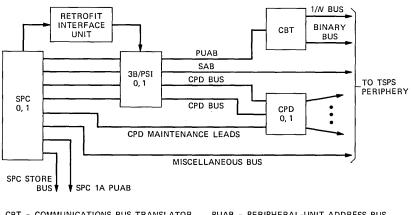
CBT - COMMUNICATIONS BUS TRANSLATOR CPD - CENTRAL PULSE DISTRIBUTOR PSI - PERIPHERAL SYSTEM INTERFACE PUAB - PERIPHERAL-UNIT ADDRESS BUS SAB - SCANNER ANSWER BUS SPC - STORED PROGRAM CONTROL
