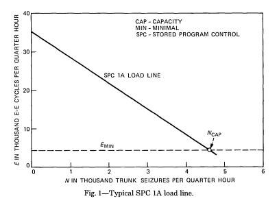
versus N load line. This information is used by the operating telephone companies in growth planning to determine how close a TSPS No. 1 site is to its capacity limit.
