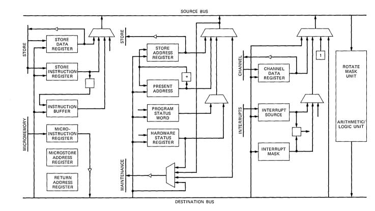
Fig. 5—Processor control architecture.
