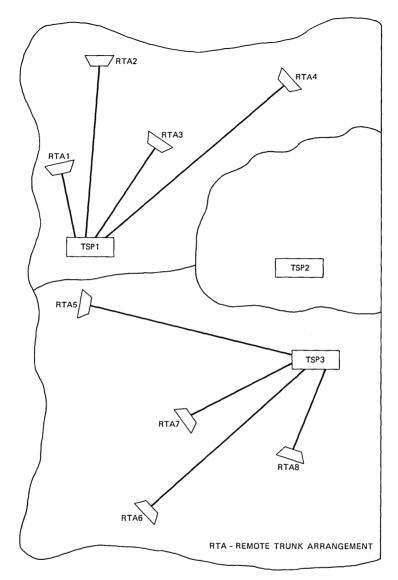
Fig. 5(a)—TSPS/RTA configuration before user move.
