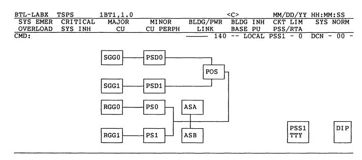
Fig. 14-Maintenance center craft interface for TSPS No. 1B.
