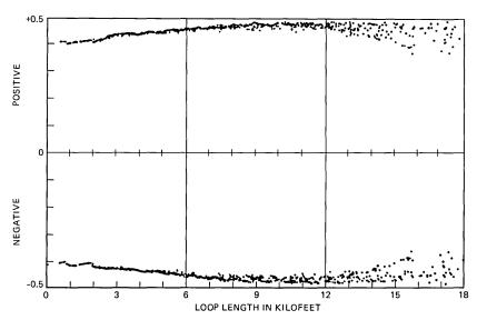
Fig. 45—Eye opening scatter plot for the 1973 survey loops at 126 kb/s  $_{\mbox{\scriptsize TCM}}$  mode. (Effective rate is 56 kb/s.)
