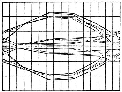
Fig. 12—Eye diagram obtained by transmission of data at 324 kb/s (for an effective bidirectional rate of 144 kb/s) in the  $\tau$ CM mode. The loop configuration is the same as that for the simulations in Fig. 11.
