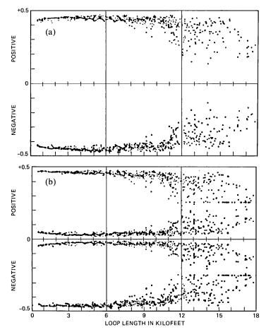
Fig. 24—Eye data scatter plots for 144-kb/s hybrid transmission with 30-dB echo cancellation. Bridged taps are stripped from the loops. Subscriber side data are given. (a) Eye opening. (b) Eye thickness.
