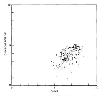
Fig. 4—Scatter plot of loop resistance plotted against its impedance (Central Office side). Temperature =  $60^{\circ}$ F, Frequency = 32 kHz, X- and Y-scales = 20 ohms/division.
