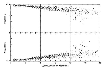
Fig. 36—Eye opening scatter plot at 324 kb/s with 20,000-ft, four-section equalizer in the  $\tau$ cm mode of transmission. Subscriber side data are given.
