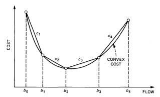
Fig. 9—Piecewise-linear approximation of a convex cost function.
