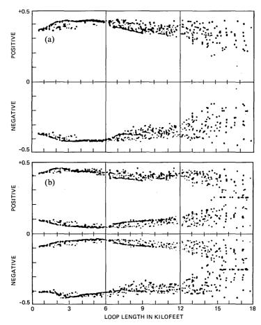
Fig. 22—Eye data scatter plots for 64-kb/s hybrid transmission with 30-dB echo cancellation. Bridged taps are stripped from the loops. Subscriber side data are given. (a) Eye opening. (b) Eye thickness.
