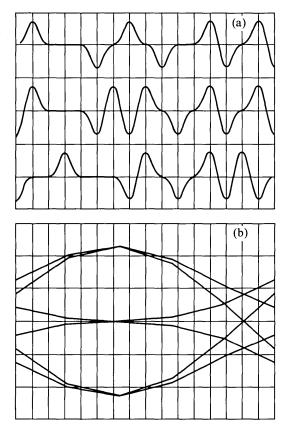
Fig. 8—System characteristics with zero loop length. (a) Pulse pattern and shape at the receiver. (b) Eye diagram at the receiver.
