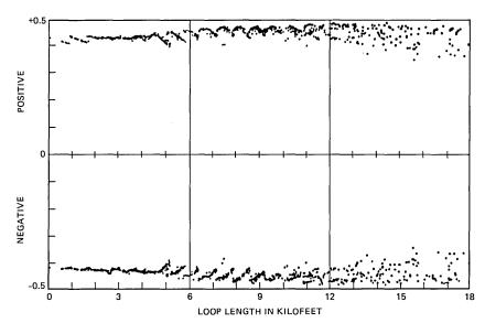
Fig. 46—Eye opening scatter plot for the 1973 survey loops at 162 kb/s  $_{\mbox{\scriptsize TCM}}$  mode. (Effective rate is 72 kb/s.)
