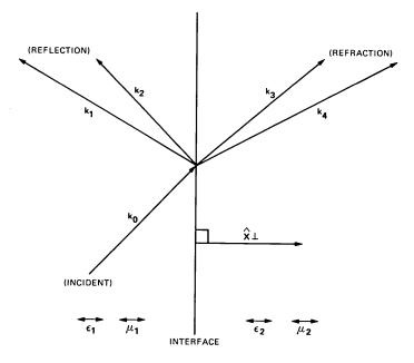
Fig. 1—Scattering at an interface between two anisotropic media.
