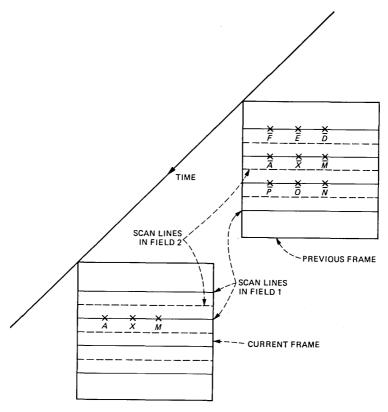
Fig. 2—Pel configuration for interframe processing.
