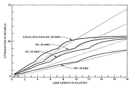
Fig. 38—Cable losses (dotted lines) and equalizer gains of a limited range, single-pole equalizer plotted for a 324-kb/s TCM design. Loop length (1 kft/division) is plotted on the X-axis and loop loss (7 dB/division) is plotted on the Y-axis.
