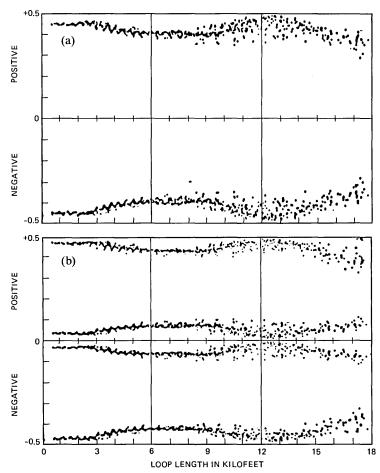
Fig. 28—Eye data scatter plots for 144-kb/s TCM-mode transmission (actual line rate is 324 kb/s). Bridged taps are stripped from the loops. Subscriber side data are given. (a) Eye opening. (b) Eye thickness.
