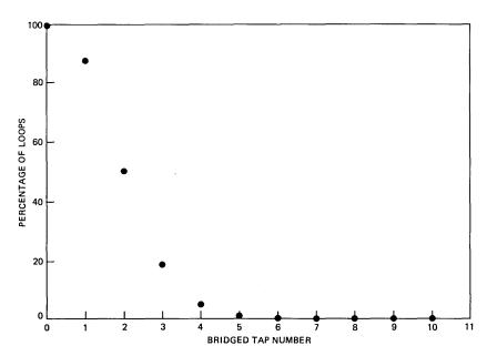
Fig. 6—Percentage of loops (Y-axis) having bridged taps equal to or greater than the bridged-tap number (X-axis) plotted.
