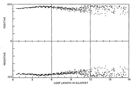
Fig. 47—Eye opening scatter plot for the 1973 survey loops at 216 kb/s  $\tau$ CM mode. (Effective rate is 96 kb/s.)
