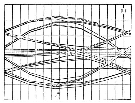
Fig. 17—Experimentally (a) and computationally (b) generated eye diagrams over a four-section (3.46 kft, 19 awg; 8.7 kft, 24 awg; 9.8 kft, 22 awg; 3.46 kft, 19 awg) loop at 324 kb/s in the  $\tau$ cm mode. The loop attenuation at half-bit rate is approximately 48 dB.
