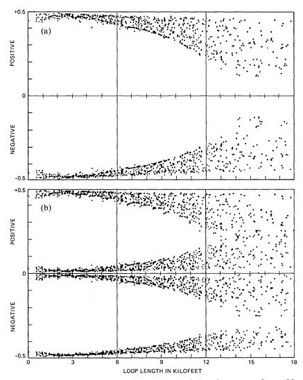
Fig. 32—Eye data scatter plot obtained by the simulation of 1973 survey loops with the three-section, 18,000-ft equalizer at  $144~\rm kb/s$ . (a) Eye opening. (b) Eye thickness.
