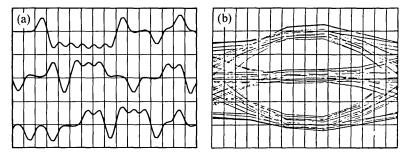
Fig. 13—Pulse pattern and eye diagram obtained by ternary code at 144 kb/s. The loop is 18 kft of No. 22 Awg cable. (a) Subscriber-side pulse pattern. (b) Subscriber-side eye diagram.
