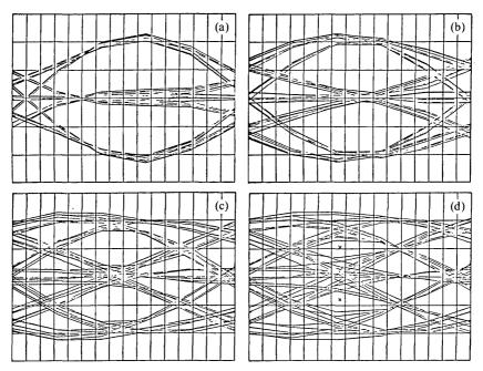
Fig. 18—Degradation of the eye diagram with an increasing number of bridged taps. (a) Subscriber-side eye diagram, no bridged taps. (b) Subscriber-side eye diagram, two bridged taps. (c) Subscriber-side eye diagram, two bridged taps. (d) Subscriber-side eye diagram, three bridged taps.
