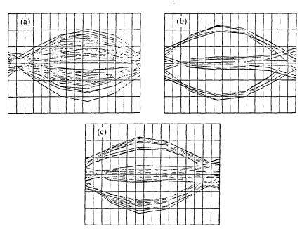
Fig. 11—Eye diagrams obtained by transmission of 144 kb/s bidirectional data over a typical loop. In (a) there is no echo cancellation, in (b) there is perfect echocancellation, and in (c) there is 30-dB echo cancellation.
