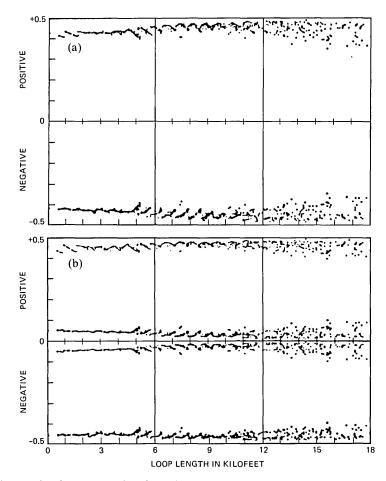
Fig. 26—Eye data scatter plots for 64-kb/s TCM-mode transmission (actual line rate is 144 kb/s). Bridged taps are stripped from the loops. Subscriber side data are given. (a) Eye opening. (b) Eye thickness.
