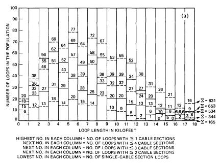
Fig. 1a—Histogram of loop population distribution by number of cable sections in each kft.
