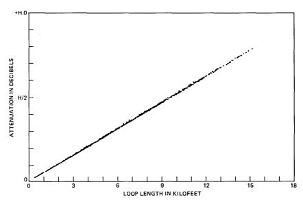
Fig. 3—Scatter plot of loop attenuations plotted against the equivalent loop length of No. 22 AWG cable. The frequency is 32 kHz and the temperature is  $60^{\circ}$ F. The X-scale is 2 kft/division and Y-scale is 5.0 dB/division.
