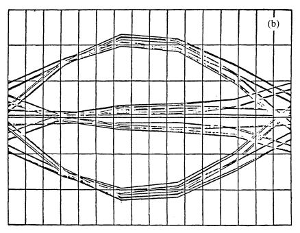
Fig. 16—Experimentally (a) and computationally (b) generated eye diagrams over 14 kft of No. 24 aws cable. The bit rate is  $324~\rm kb/s$ , and the half-bit rate loop attenuation is approximately  $39~\rm dB$ .
