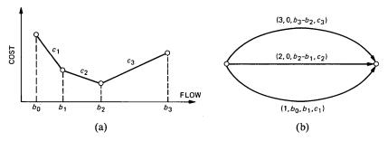
Fig. 8—Piecewise-linear, convex arc cost and equivalent parallel arc formulation.
