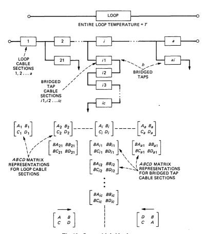
Fig. 50-Loop with bridged taps.
