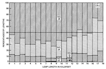
Fig. 1b—Distribution of gauge numbers with loop length.
