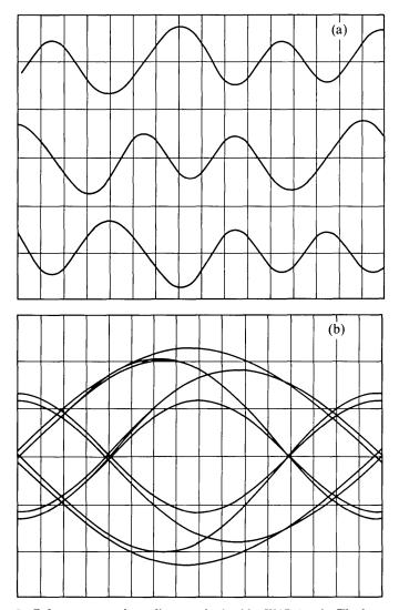
Fig. 15—Pulse pattern and eye diagram obtained by WAL-2 code. The loop configuration has nine cable sections and three bridged taps, and the bit rate is 144 kb/s. (a) Subscriber-side received data. (b) Subscriber-side eye diagram.
