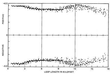
Fig. 48—Eye opening scatter plot for the 1973 survey loops at 324 kb/s. (Effective rate is 144 kb/s.)
