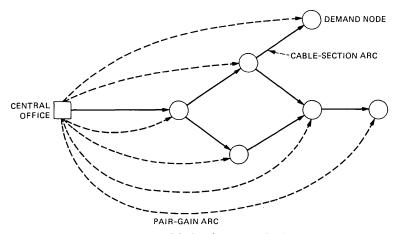
Fig. 12-Network-flow models for placement of pair-gain devices.
