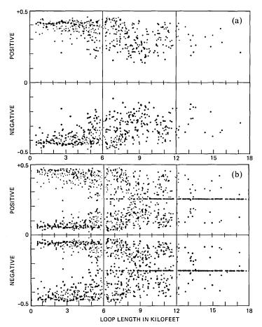
Fig. 25—Eye data scatter plots for 144-kb/s hybrid transmission with 30-dB echo cancellation. Bridged taps are left intact. Subscriber side data are depicted. (a) Eye opening. (b) Eye thickness.
