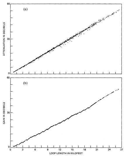
Fig. 34—Comparison of loop attenuations and equalizer gains for various loops at 144 kHz. The Y-axis scale is 6 dB/division. (a) Loop attenuation. (b) Equalizer gain.
