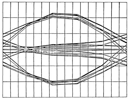
Fig. 42—Seven-section (3450 ft, No. 26 awg; 261 ft, No. 24 awg; 50 ft, No. 26 awg; 313 ft, No. 22 awg; 2477 ft, No. 24 awg; 5329 ft, No. 22 awg; and 200 ft, No. 24 awg) loop response at 324-kb/s  $\tau$ cm excitation.
