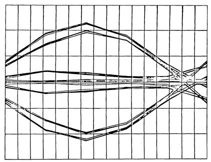
Fig. 41—Seven-section loop (88 ft, No. 19 awg; 3571 ft, No. 22 awg; 17 ft, No. 26 awg; 310 ft, No. 22 awg; 19 ft, No. 24 awg, 1299 ft, No. 26 awg; and 789 ft, No. 24 awg) response at 324-kb/s tcm excitation.
