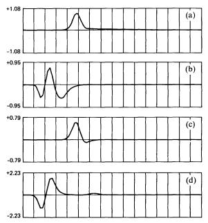
Fig. 9—Transmission and reflection of a single pulse on a typical loop consisting of three cable sections. Pulse rate is 144 kb/s, and each box width corresponds to 1-pulse duration. (a) Received pulse at s end of loop. (b) Reflected pulse at s end of loop. (c) Received pulse at co end of loop. (d) Reflected pulse at co end of loop.
