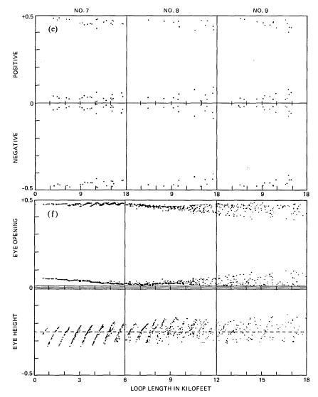
Fig. 21—(e) Eye thickness for loops with 7-, 8-, or  $\geq$ 9-cable sections versus loop length in kft (numbers indicate number of sections). (f) Eye thickness and eye height for all loops versus loop length in kft.
