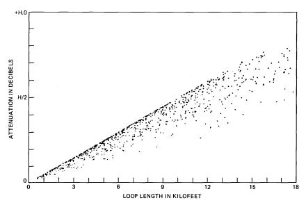
Fig. 2—Scatter plot of loop attenuations plotted against the loop length at 32 kHz and  $60^{\circ}$ F. The X-scale is 1 kft per division and Y-scale is 5.0 dB/division.
