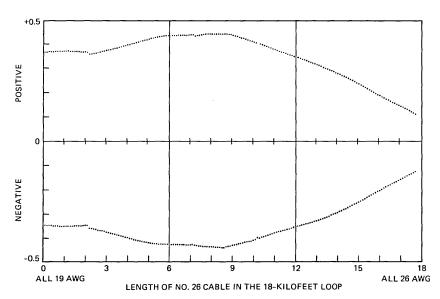
Fig. 31—Eye openings with Nos. 19 and 26  $_{\hbox{AWG}}$  composite cable loops having a total length of 18 kft (144 kb/s).
