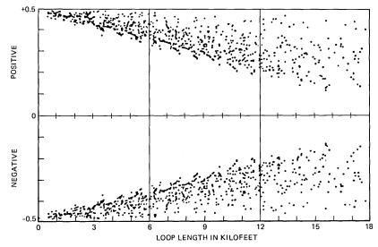
Fig. 37—Eye opening scatter plot at 126 kb/s with 20,000-ft, four-section equalizer in the  $\tau$ cm mode of transmission. Subscriber side data are given.
