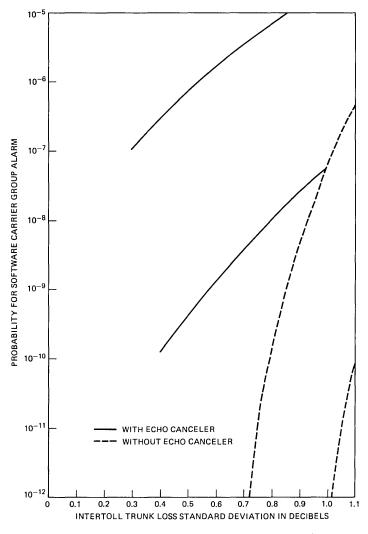
Fig. 7-Probability bounds for software carrier group alarm.
