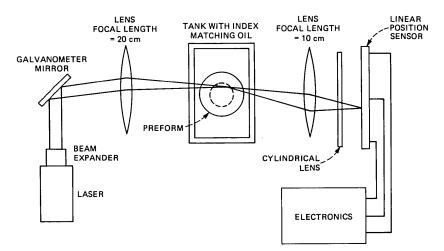
Fig. 28—Arrangement for profiling of preforms by the ray tracing method.
