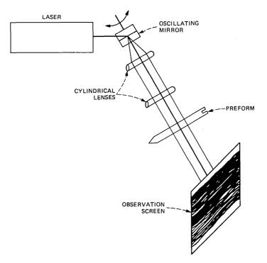
Fig. 21-Arrangement to produce preform diagnostigrams.
