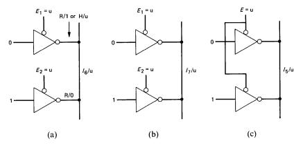
Fig. 13—Generation of indeterminate impedances.
