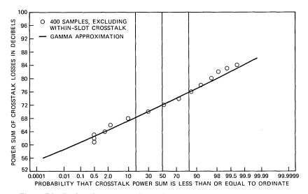
Fig. 6—Distribution of power sum of 48, pair-to-pair, non-within-slot, crosstalk losses of 466-type T1 apparatus case. Data measured from eight apparatus cases in Bell Laboratories, Atlanta. Data represents between-slot crosstalk component of data in Fig. 5.
