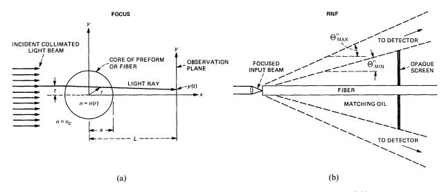
Fig. 3—Principle of operation of (a) focusing method, and (b) refracted near-field (RNF) technique.
