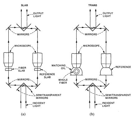
Fig. 2—Schematic diagram of (a) slab interferometric method, and (b) transverse interferometric method. The interference microscope used in both cases is identical.
