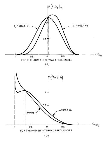
Fig. 6—Density functions required for detection when frequency shift is considered but the additive noise is ignored  $(A \rightarrow \infty)$ .
