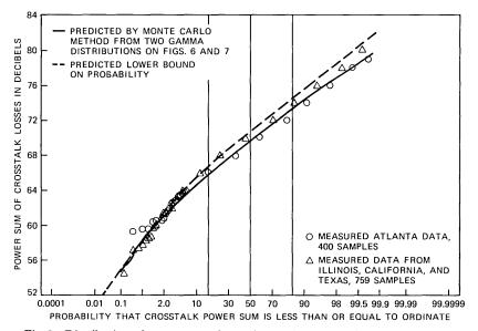
Fig. 3—Distribution of power sum of 50 pair-to-pair crosstalk losses of 466-type T1 apparatus case from laboratory measurements in Atlanta and field measurements in Illinois, California, and Texas.
