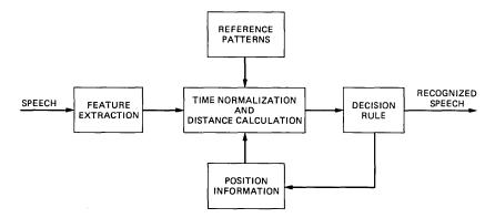
Fig. 1-Block diagram of a generic connected word recognition system.
