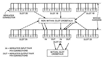
Fig. 2—Wiring diagram on the backplane of 466-type T1 apparatus case showing within-slot crosstalk and non-within-slot crosstalk for slot 24.
