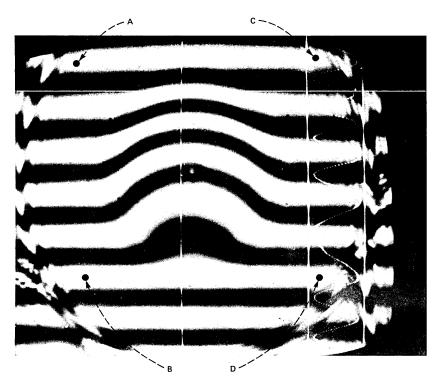
Fig. 23—Fringes observed in a graded-index SLAB sample.
