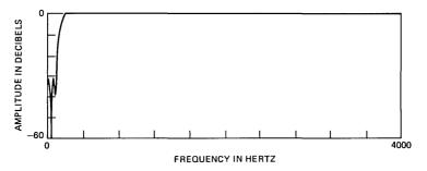
Fig. 4—Frequency response of high-pass filter for 4B-SBC.
