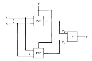
Fig. 9—General model for tristate devices.
