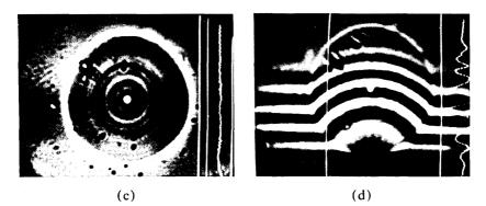
Fig. 4—Two fiber-SLAB samples observed by (a,c) ordinary microscopy, and by (b,d) interference microscopy.
