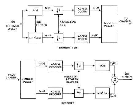
Fig. 2-Two-band sub-band coder used in simulation.
