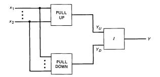
Fig. 7-General model for CMOS and TTL totem pole devices.
