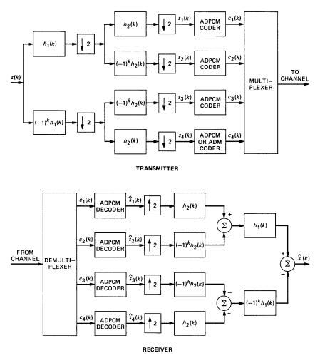
Fig. 3—Four-band sub-band coder used in simulation.
