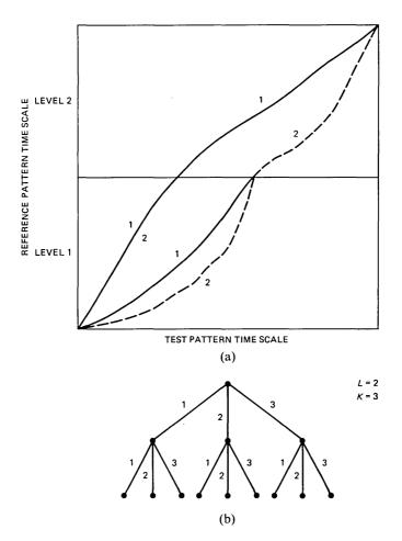
Fig. 6—Generation of multiple candidate strings for the LB algorithm.
