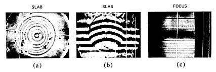
Fig. 10—Fiber no. 3 as observed by (a) ordinary microscopy, (b) slab interference microscopy, and (c) the focusing method.
