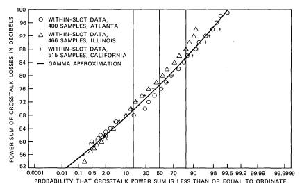
Fig. 7—Distributions of power sum of two, pair-to-pair, within-slot, crosstalk losses of 466-type T1 apparatus case from laboratory measurements in Atlanta and field measurements in Illinois and California. Data represents within-slot crosstalk component of data in Figs. 3 and 5.
