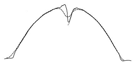
Fig. 18—Profiles of fiber no. 5 as measured by RNF (solid), FOCUS (dotted), and TRANS (broken) techniques.
