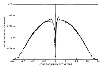
Fig. 19—Profiles of the preform stub from which fiber no. 5 was pulled as measured by the ray-tracing technique (solid curve) and the focusing method (broken). The two halves of each profile were obtained from measurements at two orientations.
