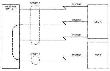
Fig. 3-Line group and alternate delivery.
