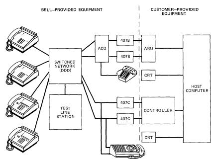
Fig. 2-Switched Network Transaction Telephone System, second phase.
