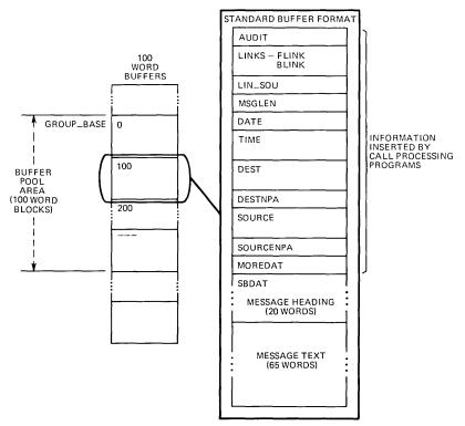
Fig. 2—Standard buffer format structure.
