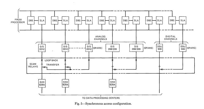
Similarly, the SLA is programmed to interrupt after a given number of characters has been received. An interrupt is also generated when the associated data set detects loss of carrier. In addition, up to 256 special characters may be programmed into the SLA such that an interrupt will be generated whenever any of those special characters is received. The receive interrupts may also be disabled.
