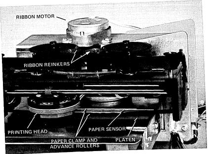
Fig. 4—Printing mechanism.
