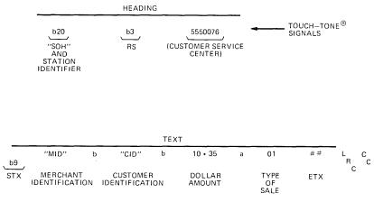
Fig. 7—Dial-in telephone message format.
