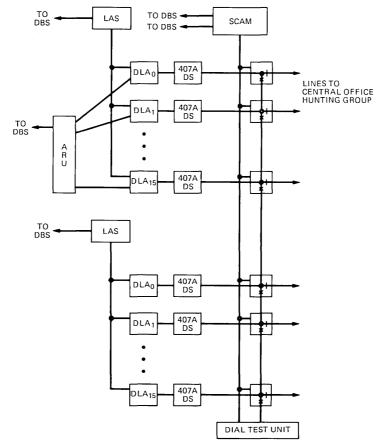
Fig. 7-Dial-in network configuration.
