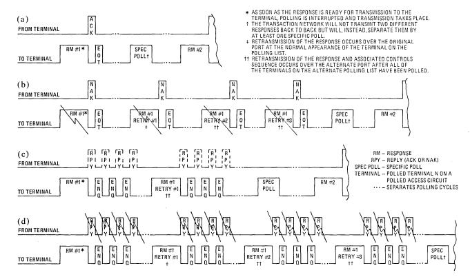
Fig. 7—(a) Normal response transfer. (b) Garbled response from the Transaction Network. (c) Lost reply from the terminal. (d) Garbled reply from the terminal.
