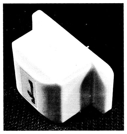
Fig. 9-Transaction III read head.
