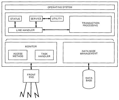
Fig. 2-Sample software configuration.
