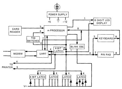
Fig. 6-Transaction III block diagram.
