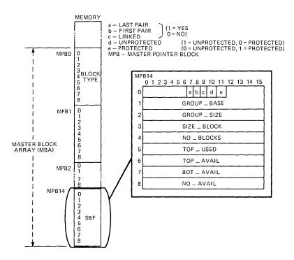
Fig. 3-Master block array.
