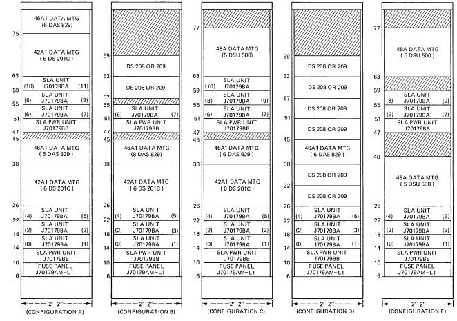
Fig. 7—Synchronous line adapter frame.
