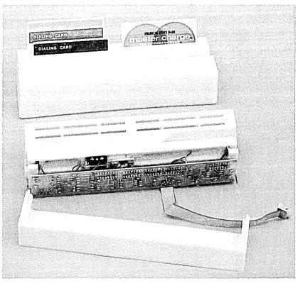
Fig. 8—Transaction III card reader.
