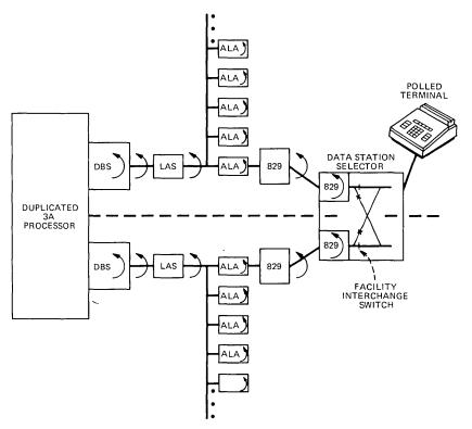
Fig. 11—Asynchronous polled access line loopbacks ()).
