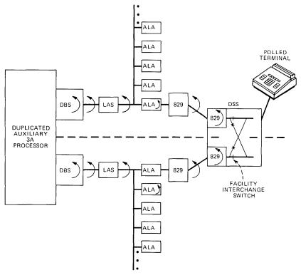
Fig. 2-Asynchronous polled access line configuration.
