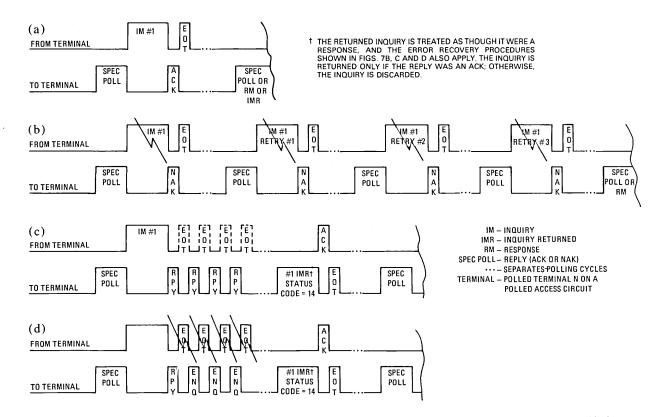
Fig. 6—(a) Normal inquiry transfer. (b) Garbled inquiry from the terminal. (c) Lost termination from the terminal. (d) Garbled termination from the terminal.
