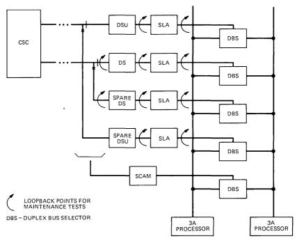
Fig. 9-Synchronous access line configurations.
