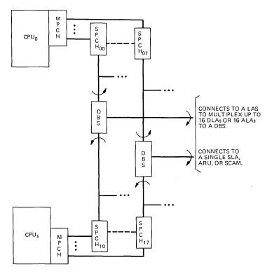
Fig. 1—Switch configuration.
