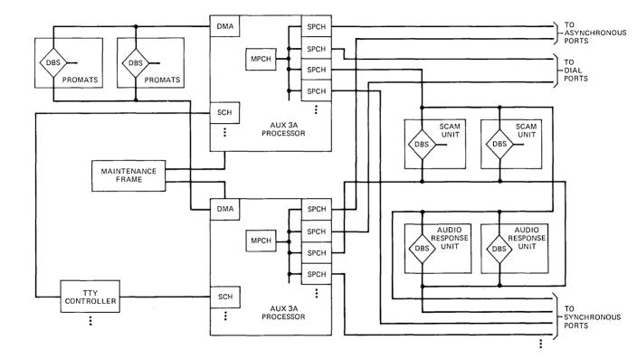
Fig. 1-Message switch common equipment.
