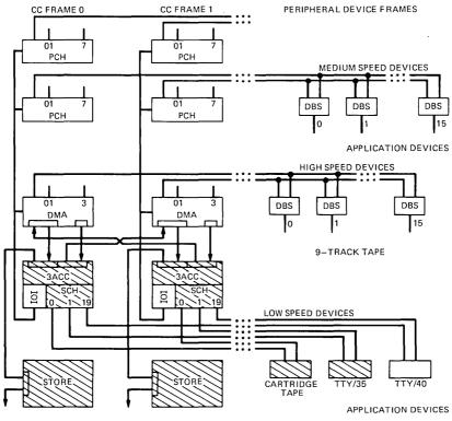
Fig. 1—3A Processor configuration.
