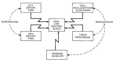
Fig. 8—Dial call processing—task communications.
