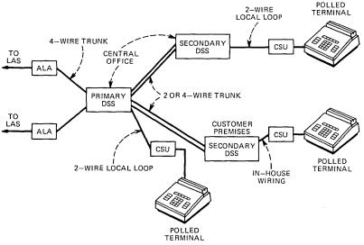
Fig. 5—Possible polled access circuit configuration.
