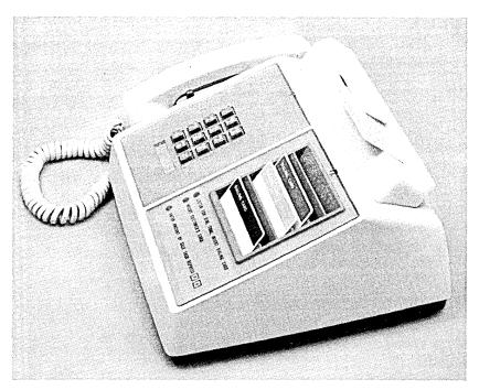
Fig. 6—Transaction set with first slot reader.
