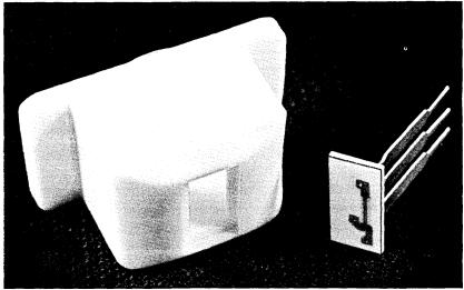
Fig. 10-Components of read head.
