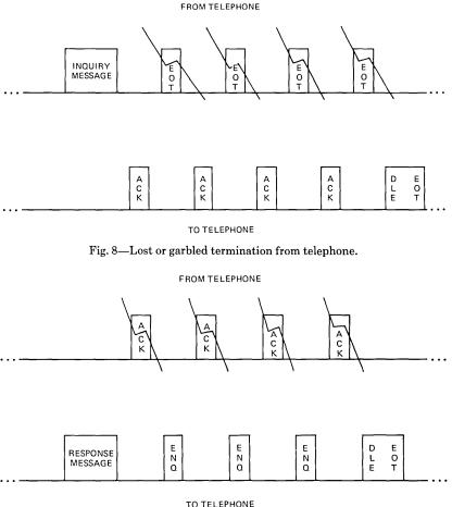
Fig. 9—Lost or garbled replies from telephone.
