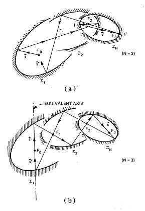
Fig. 4—(a) 2N successive reflections. (b) The central path. The equivalent axis through  $F_0$  is obtained by varying in (a) the initial direction  $\vec{s}$  until  $\vec{s} = \vec{s}''$  as shown in (b).
