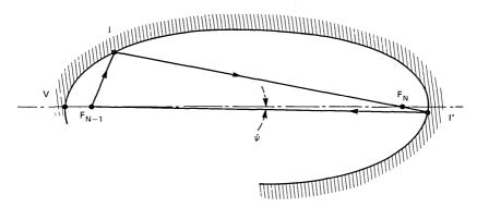
Fig. 5—As the distance of  $F_N$  from the other focus  $F_{N-1}$  is increased, keeping V and  $F_{N-1}$  fixed, the ellipsoid approaches a paraboloid with vertex V and focus  $F_{N-1}$ ; for the ray reflected at I' one has  $\psi \to 0$ .
