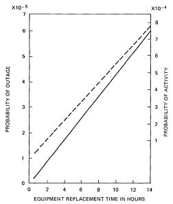
Fig. 8—Probabilities of outage and activity as functions of equipment replacement time.
