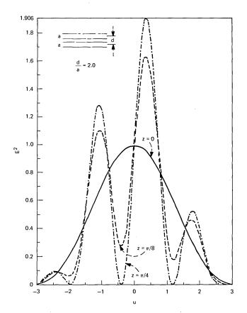
Fig. 3—Computer plots of energy distribution as a function of normalized radiation angle u for the case d/a = 2, with  $Z = \kappa z$  as the parameter.
