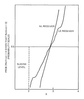
Fig. 4—Comparison of distribution functions of the receiver output Y(n) for the linear and nonlinear receivers (data from channel 14).
