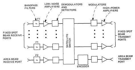
Fig. 3—Regenerative transponder for a hybrid spot-area coverage satellite employing channel coding. The allocated band is split between the spot and area beams on the uplink. The band is totally reused for all the downlinks.
