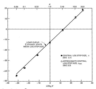
Fig. 7—Load curve  $(\vec{d})$ , central log step size (c), and approximate log step size ( $c_{app}$ ) for uniform 16-level quantizer and Gaussian, zero-mean, input signal variables of variance  $\sigma^2$ . The log multipliers are given in (39) and Q = 1.1. Interleaving interval, I = 16 and leakage,  $\gamma = 0.777$ .
