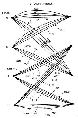
Fig. 4—State diagram for maximum-likelihood detection of interfering coded and uncoded signals. A K = 3,  $r = \frac{1}{2}$  convolutional code is assumed. For each transition, the first two channel digits correspond to the coded symbols, and the second two correspond to the uncoded symbols.
