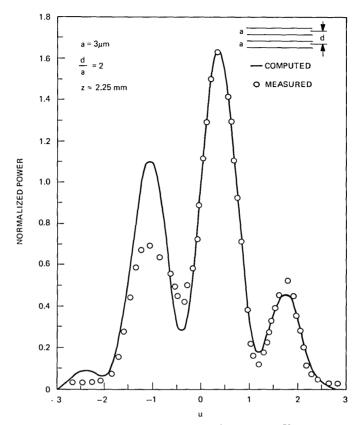
Fig. 8—Radiation pattern of the same coupler shown in Fig. 7, but at a different  $z \simeq 5\pi/8$ , past the location of complete energy transfer.
