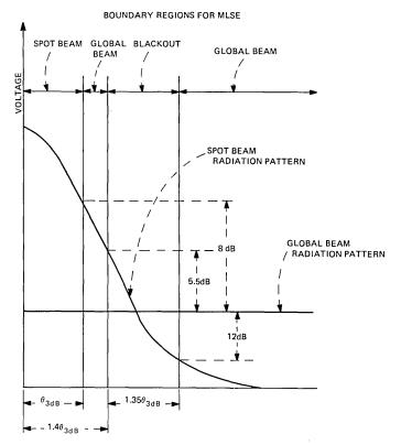
Fig. 11—One-dimensional plot showing the usable regions attainable via MSLE for a hybrid spot-area beam satellite system employing a K = 7, r = 1/2 code for the area beam transmission. The spot beam antenna pattern is Gaussian shaped.
