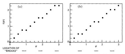
Fig. 3—Machine arithmetics incorporating contraction properties and fidelity criterion for (a) truncating and (b) rounding external arithmetics.  $\gamma = \frac{3}{4}$  and L = 2 (see Section 2.2).
