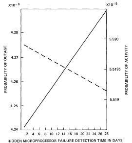
Fig. 9—Probabilities of outage and activity as functions of hidden microprocessor failure detection time.
