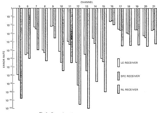
Fig. 5—Comparison of error rates for the three receivers.
