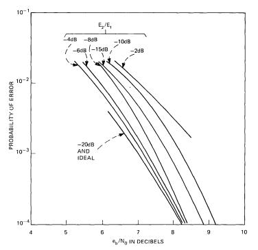
Fig. 7—Uncoded bit error rate performance of maximum-likelihood detector vs  $e_b/N_o$  obtained via simulation for select values of interference.
