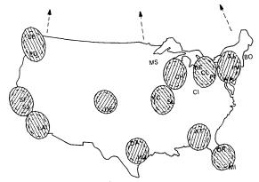
Fig. 2—Footprints of a hypothetical 11-beam system showing -1, -2, and -3 dB contours. Both polarizations are employed.
