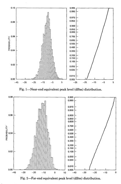
distance between end offices the more the signals are attenuated. This source of variation explains the greater variability among the far-end signal powers. These near-end, far-end differences exist for both EPL and average power; however, a comparison of the near- and far-end EPL results gives a difference of 2.1 dB, while a similar comparison for the average power measures gives a difference of 2.9 dB. In the following
