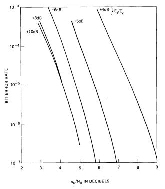
Fig. 8—Bound on coded bit error rate performance of maximum-likelihood detector vs  $e_b/N_o$  for select values of interference.
