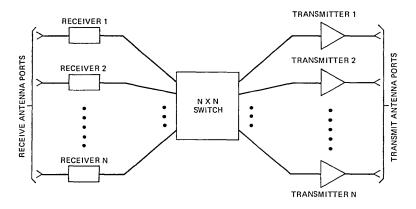
Fig. 1-Satellite transponder.
