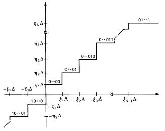
Fig. 1—The quantizer. A natural coding scheme is displayed. The step size is timevarying and the parameters  $(\xi_n)$  and  $(\eta_n)$  are prespecified and fixed.
