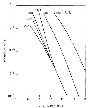
Fig. 6—Bound on uncoded bit error rate performance of maximum-likelihood detector vs  $e_b/N_o$  for select values of interference.
