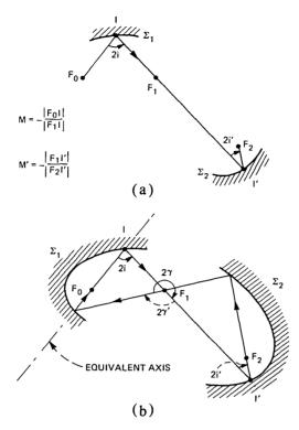
Fig. 10-Central path and equivalent axis of a combination of two ellipsoids.
