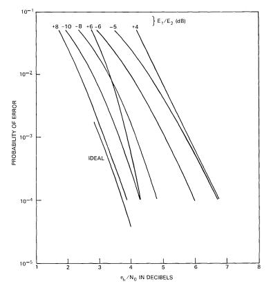
Fig. 9—Coded bit error rate performance of maximum likelihood detector vs  $e_b/N_o$  obtained via simulation for select values of interference.
