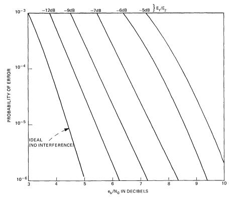
Fig. 10—Measured bit error rate performance of a K = 7,  $r = \frac{1}{2}$  convolutional code vs  $e_b/N_o$  for select values of interference. The interference is bit-synchronous with the encoded channel bits, and the ordinary Viterbi algorithm with soft (3-bit) quantization is employed.
