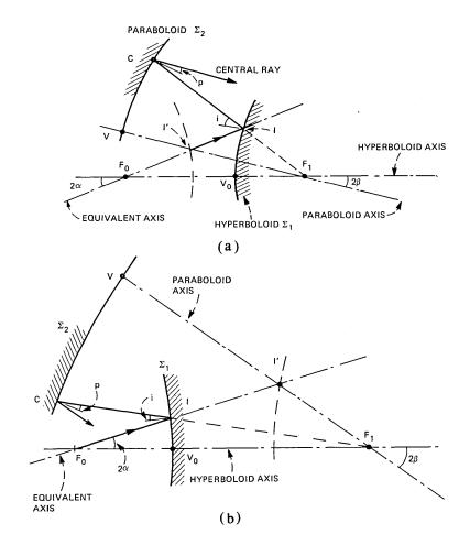
Fig. 7—How to determine the central path and the equivalent axis of a paraboloid combined in (a) with a convex hyperboloid and in (b) with a concave hyperboloid.
