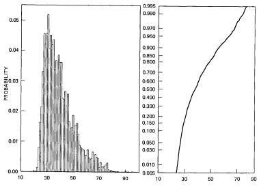
Fig. 14-Near-end loop current (mA) distribution for residential.
