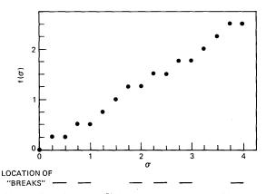
Fig. 4—Machine arithmetic for  $\gamma = \frac{5}{8} (L = 2)$  for two fractional bits in machine word and truncating external arithmetic. The contraction requirements and fidelity criterion are satisfied.
