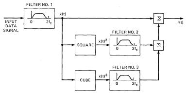
Fig. 2—Model of a nonlinear channel.
