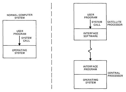
Fig. 2—Satellite processor concept.
