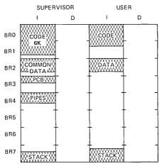
Fig. 3—UNIX<sup>TM</sup> process virtual address space.
