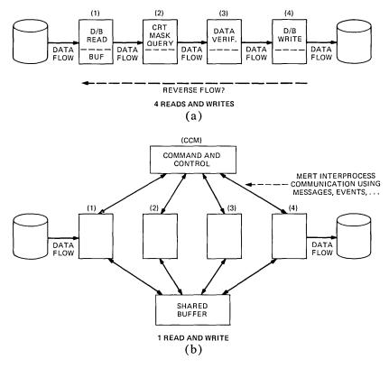
Fig. 3—(a) UNIX<sup>TM</sup> shell architecture. (b) MERT shell architecture.
