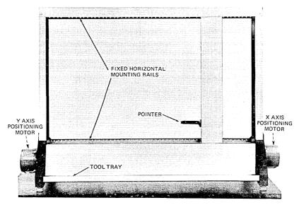
Fig. 4—Standard Logic semi-automatic wire-wrap machine.
