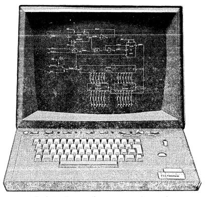
Fig. 2—The Tektronix 4014 terminal displaying a circuit.
