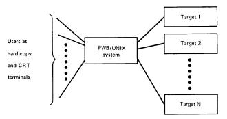
Fig. 1—PWB/UNIX<sup>TM</sup> interface with its users.
