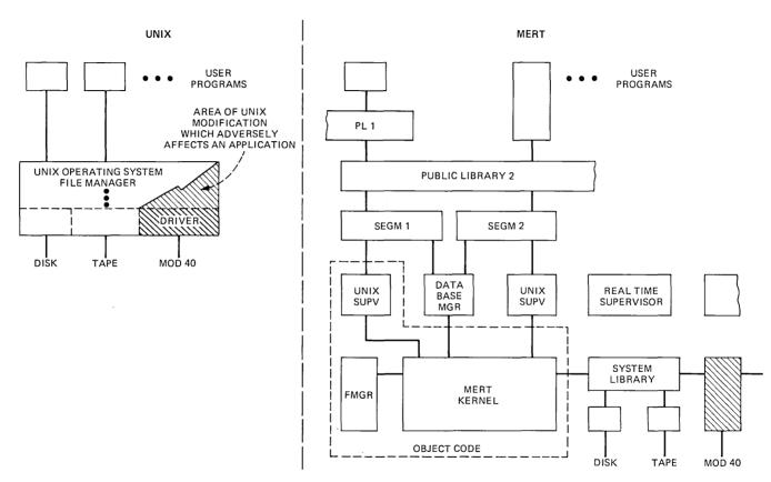
Fig. 2—UNIX<sup>TM</sup> and MERT executive architectures with possible application interfaces.
