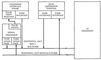
Fig. 1—Communication path between 1A Processor and VIF and EST.
