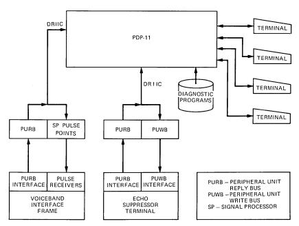
Fig. 2—No. 4 ESS diagnostic support environment.
