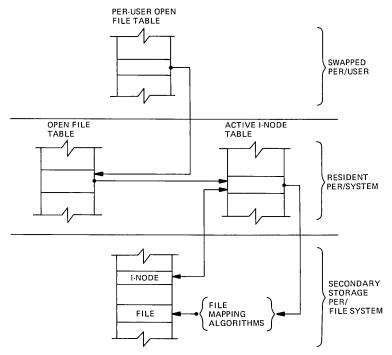
Fig. 2—File system data structure.
