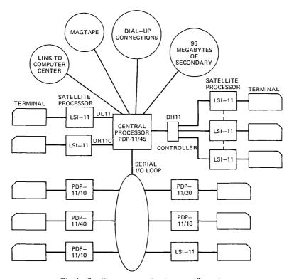
Fig. 1—Satellite processor hardware configuration.
