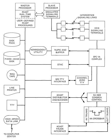
Fig. 6—4CAST system in switching office configuration.
