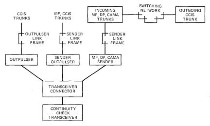
Fig. 2—Connecting continuity check transceiver.
