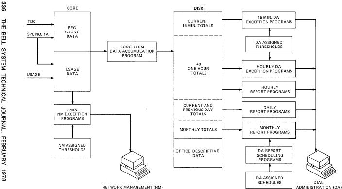
Fig. 6—PBC data accumulation.
