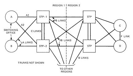
Fig. 1—CCIS signaling network.
