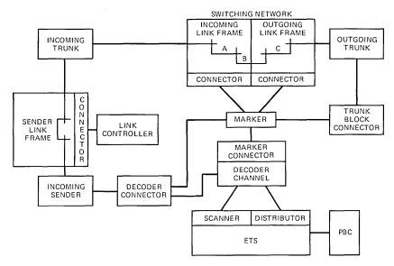
Fig. 1-Block diagram of 4A/ETS.
