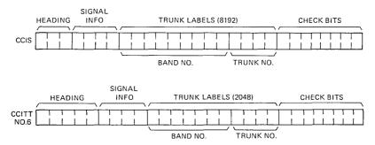
Fig. 7—Lone Signal Unit (LSU) format.
