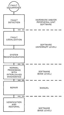
Fig. 6—Fault reaction sequence.
