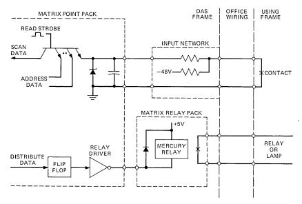
Fig. 22—Distribute and scan circuits.
