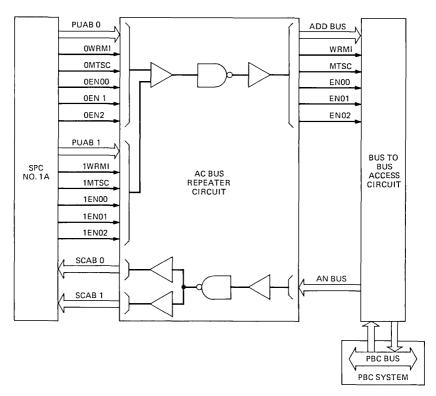
Fig. 3—SPC to PBC interface block diagram.
