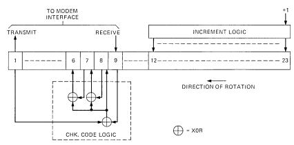
Fig. 13—Logic register layout and check code generation.
