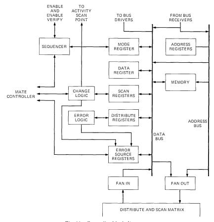
Fig. 23—Controller block diagram.
