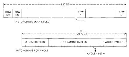
Fig. 24—Autonomous cycle timing.
