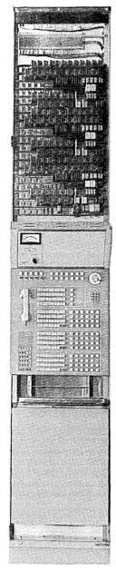
Fig. 33—CCIS intra-office trunk test frame.
