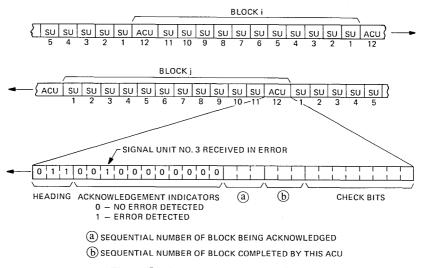
Fig. 5—Block structure, CCIS SUs and ACU.
