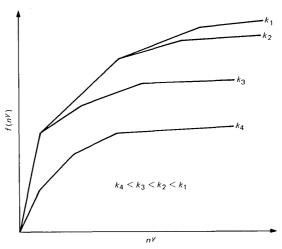
Fig. 1—Linear programming optimal value  $[f(n^y)]$  as a function of the number of CCIS office conversions  $n^y$  and trunk group conversions k.
