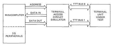
Fig. 8—Terminal unit test system configuration.
