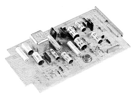
Fig. 6—Discrete component circuit pack.
