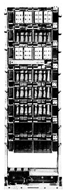
Fig. 35—Voice frequency link access frame.
