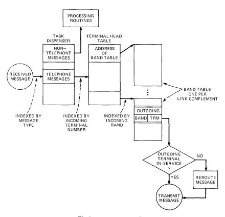
Fig. 5—STP message routing.
