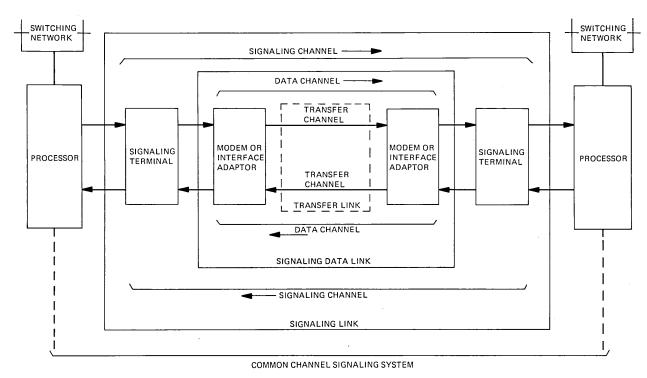
Fig. 4—Basic block diagram of the Common Channel Interoffice Signaling System.
