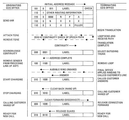
Fig. 13—CCIS signaling for a 10-digit call.
