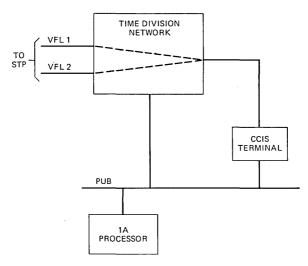
Fig. 2—CCIS data link configuration.
