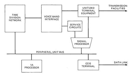
Fig. 1-No. 4 ESS system architecture.
