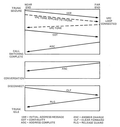
Fig. 4—Typical signal unit exchange.
