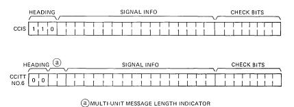
Fig. 9—Subsequent Signal Unit (SSU) format.
