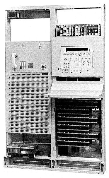
Fig. 34—Voice frequency link test frame.
