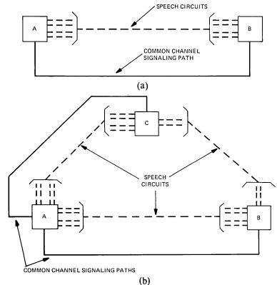
Fig. 2—(a) Associated signaling. (b) Nonassociated signaling.
