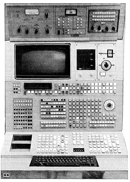
Fig. 36—Close up of integrated manual test frame.
