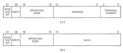
Fig. 10—(a) Terminal operation command format. (b) TAC operation command format.
