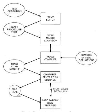
Fig. 4—Generation of 4CAST procedures.
