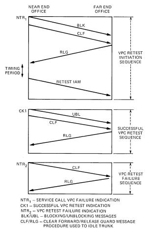
Fig. 8—VPC retest signaling sequence.
