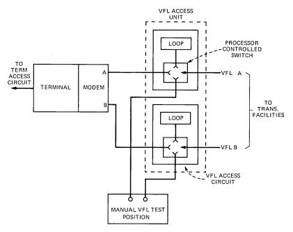
Fig. 7—Switching office VFL test arrangements.
