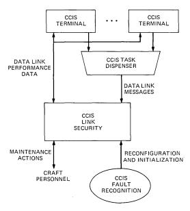
Fig. 7—CCIS link security module.
