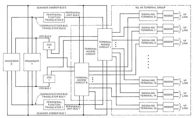
Fig. 7—No. 4A crossbar terminal group block diagram.
