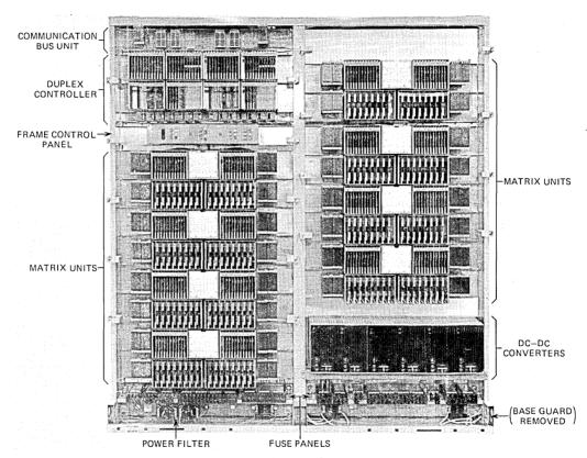
Fig. 21—Distributor and scanner frame.
