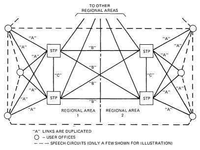
Fig. 3—User offices connected to STP quad.
