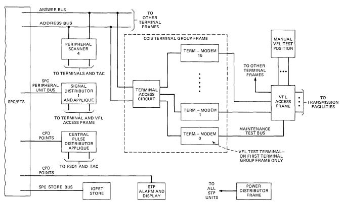
Fig. 3—ETS/STP system block diagram.
