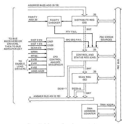
Fig. 4—Block diagram of bus-to-bus access circuit.
