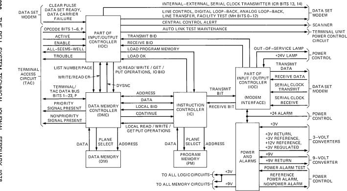
Fig. 11—Terminal unit block diagram.
