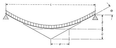
Fig. 9-WT4 sheath on simple supports.
