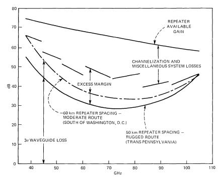
Fig. 2—WT4A system loss composite.
