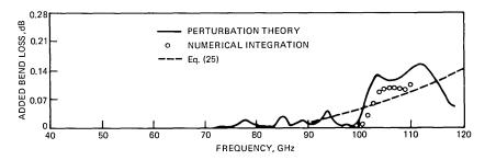
Fig. 13—Added TE<sub>01</sub> loss for plan bend in WT4 field evaluation test.
