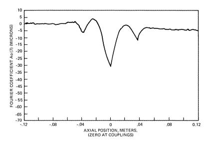
Fig. 6-Radius distortions in a welded coupling.
