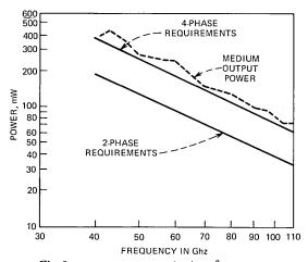
Fig. 3—IMPATT power output vs. frequency.
