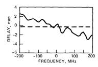
Fig. 1—Unequalized loss and delay characteristics.
