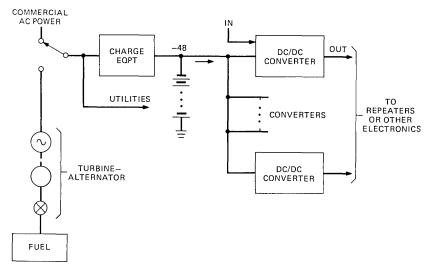
Fig. 8—Local powering arrangement for WT4 repeaters.
