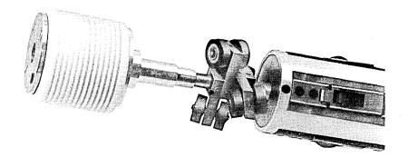
Fig. 9—Detail of propeller and pneumatic piston.
