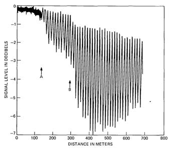
Fig. 10—Moving piston measurement of relative  ${\rm TE}_{01}$  level for 720-m-long section at 113 GHz.
