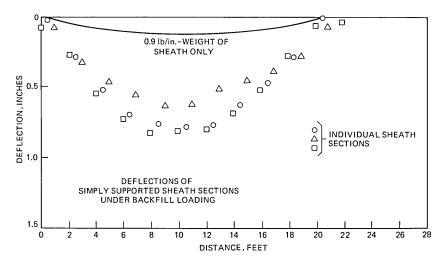
Fig. 6—Experimental determination of effective sheath loading.
