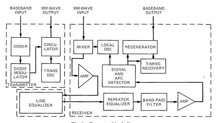
Fig. 9—Repeater block diagram.
