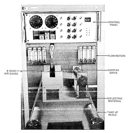
Fig. 12—Dielectric thickness gauge.
