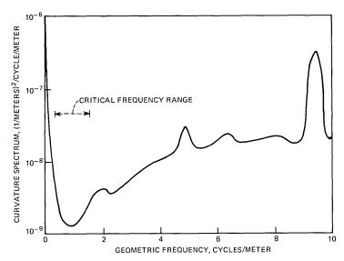
Fig. 1—Curvature spectrum of installed 60-mm waveguide.
