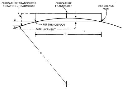
Fig. 1—Principle of measurement with three-point gauge.
