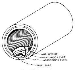
Fig. 5-Helix waveguide.
