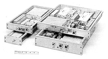
Fig. 15—Field evaluation test repeater.
