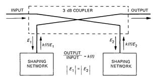
Fig. 3—Basic equalizer configuration.
