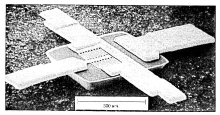
Fig. 7—Large area microwave transistor.
