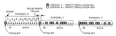
Fig. 11—Data burst timing diagram.
