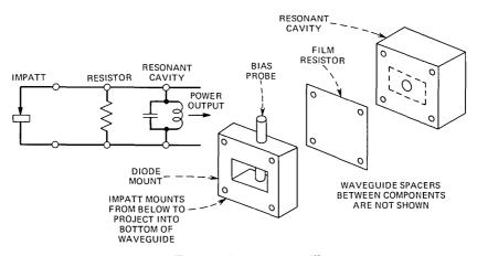
Fig. 3—Transmitting IMPATT oscillator.
