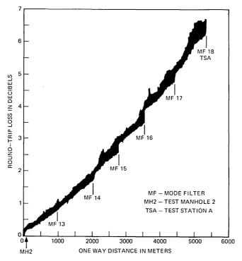
Fig. 5—Moving piston measurements, 95.8 GHz.
