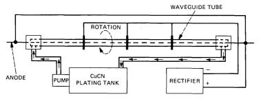
Fig. 10--Horizontal plating system.
