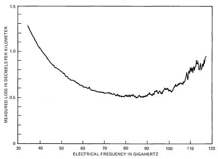
Fig. 11—WT4 field evaluation test measured loss.
