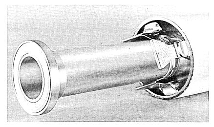
Fig. 1—Components of WT4 sheathed waveguide medium.
