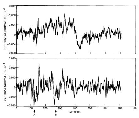
Fig. 8-Measured curvature for 720-m-long section in WT4 field evaluation test.
