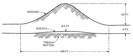
Fig. 3—Cross section through a hypothetical ridge.
