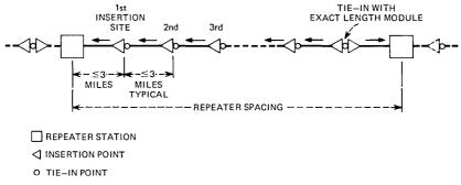
Fig. 1—Insertion segments within a waveguide repeater span.
