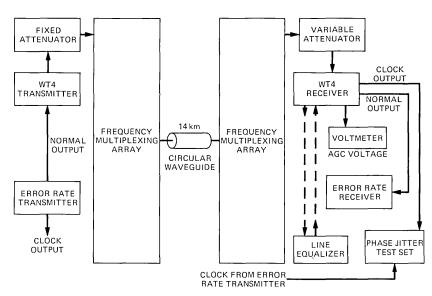
Fig. 3—Equipment arrangement for field measurements.
