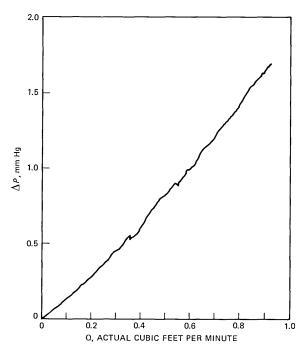
Fig. 3—Flow characteristics of WT4 sheath.
