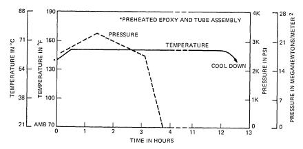
Fig. 17-Iron-loaded epoxy cure cycle.
