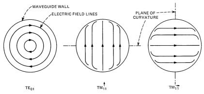
Fig. 1—Normal mode electric fields in dielectric-lined waveguide.
