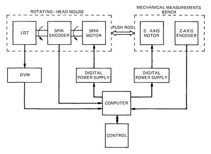
Fig. 4—Rotating-head mouse system block diagram.
