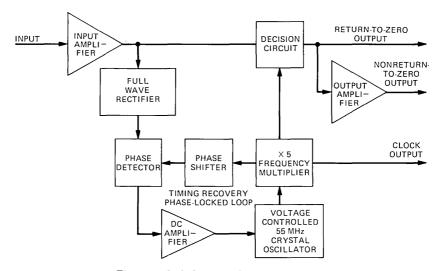
Fig. 13—Block diagram of WT4 regenerator.
