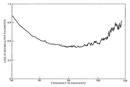
Fig. 5—Field evaluation test waveguide measured loss.
