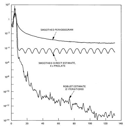
Fig. 18—Comparison of three estimates of spectrum for the data shown in Fig. 12. The systematic oscillations in the center curve are a result of interactions between the two outliers.
