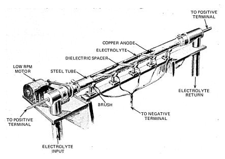
Fig. 9—Copper plating system.
