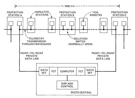
Fig. 6—Double access configuration.
