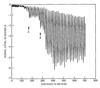
Fig. 11—Calculated TE<sub>01</sub> level for 720-m-long section at 113 GHz.
