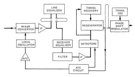
Fig. 1-WT4 repeater block diagram.
