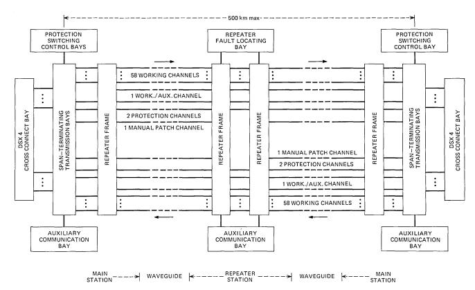
Fig. 1-Layout of protection span.
