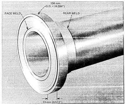
Fig. 13-Flanged end of waveguide.
