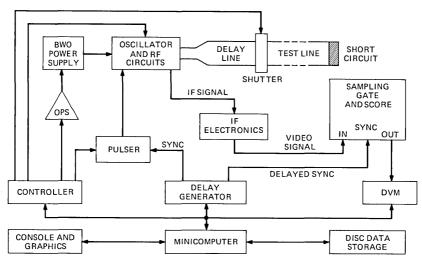
Fig. 2-Millimeter waveguide transmission measurement system.
