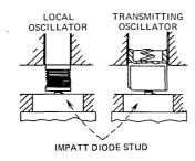
Fig. 18—Bias rods for WT4 oscillators.
