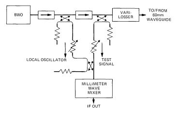
Fig. 3—RF millimeter-wave circuit arrangement.
