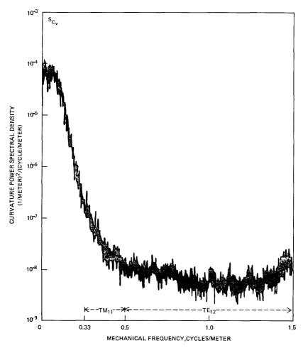
Fig. 4—Average field test vertical curvature spectrum.
