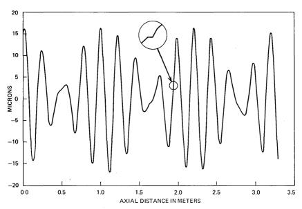
Fig. 12—Plot of the horizontal curvature gauge output for an experimental dielectriclined waveguide. The insert shows one of two outliers in this data set.
