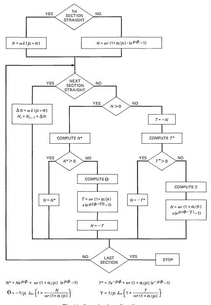
Fig. 14—Insertion force flow diagram.
