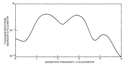
Fig. 11-PSD of dielectric tubing thickness.
