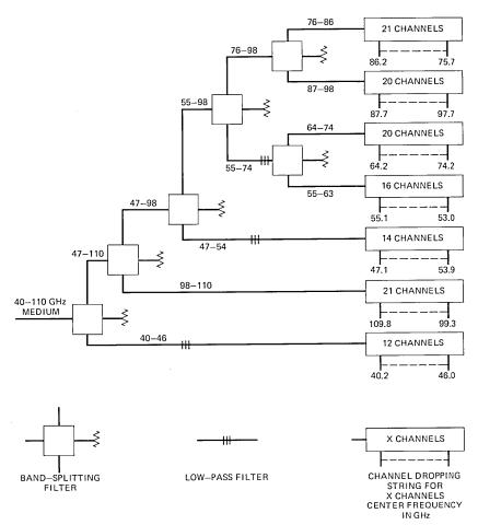
Fig. 2—Channelizing array.
