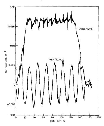
Fig. 6—Measured curvature data for experimental route bend.
