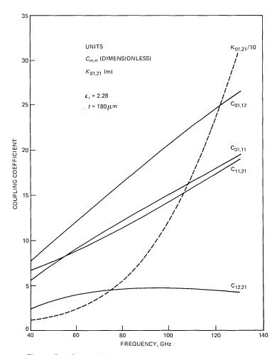
Fig. 4—Coupling coefficients for 60-mm-diameter lined waveguide.
