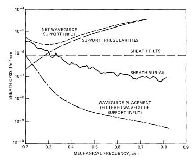
Fig. 14—Components of waveguide placement spectrum.
