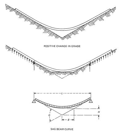
Fig. 4—WT4 sheath at positive change in grade.
