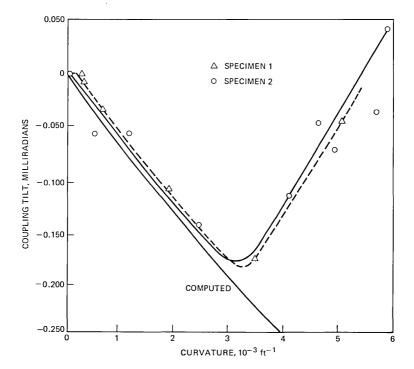
Fig. 13—Apparent tilt due to excess stiffness.
