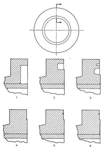
Fig. 12—Flange design stages.
