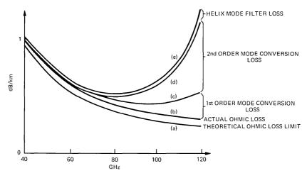
Fig. 6—Addition of the various loss components.
