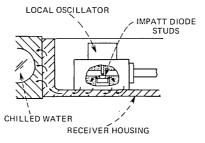
Fig. 17—Thermal path for receiving oscillator.
