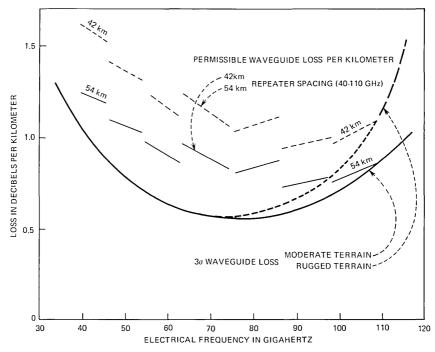
Fig. 12—Waveguide loss and repeater spacing.
