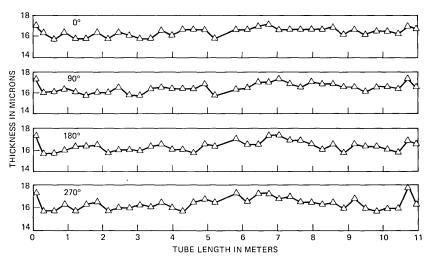
Fig. 11—Plating thickness results.
