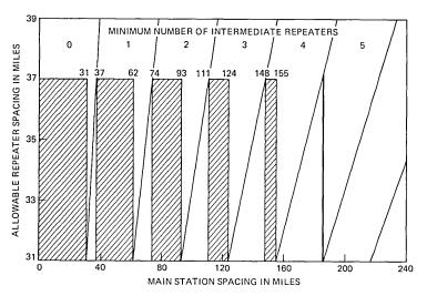
Fig. 1—Minimum number of intermediate repeaters.
