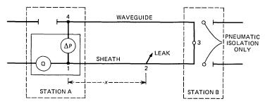
Fig. 2-Locating a leak.
