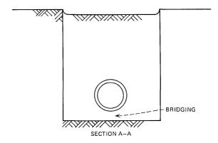
Fig. 4—Sheath-soil interaction model.
