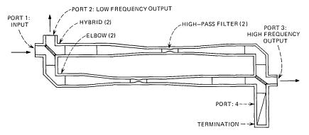
Fig. 3—Band-splitting filter.
