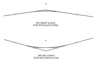
Fig. 6—Sample beam-curve overlays.
