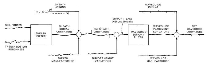
Fig. 2—Waveguide curvature inputs and filtering.
