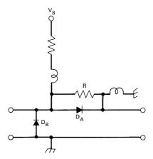
Fig. 10—Schematic of variable attenuator.
