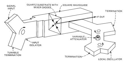
Fig. 2—Down-converter assembly.
