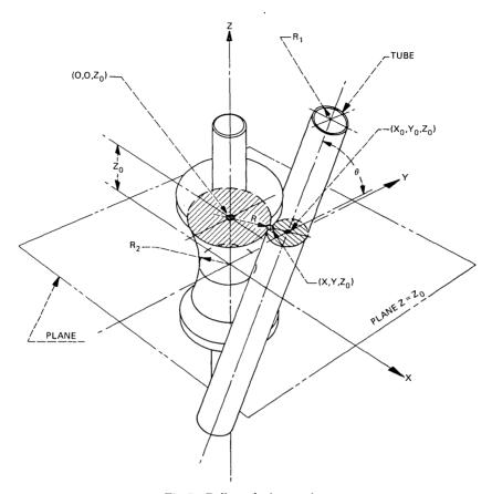
Fig. 5—Roller-tube interaction.
