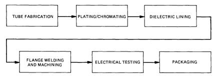
Fig. 2—Dielectric-lined waveguide processing.
