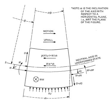
Fig. 11—Equilibrium of an element of waveguide.
