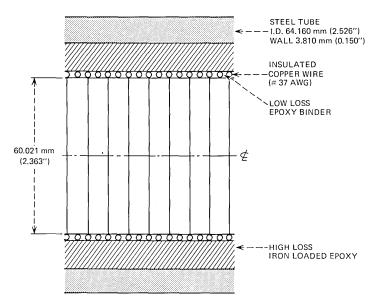
Fig. 15—Helix cross-sectional geometry.
