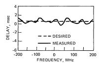
Fig. 9—Loss and delay in equalized line.
