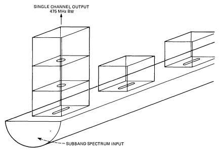
Fig. 4—Channel-dropping filter.
