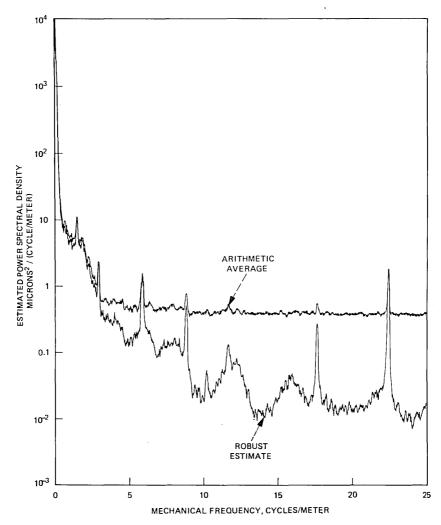
Fig. 8—Comparison of pilot spectrum estimates formed by robust and arithmetic average combinations of the subset spectrum estimates (shown in Fig. 7) for mode filter section 3 horizontal curvature. For plotting purposes both estimates have been smoothed with an adaptive filter having a span of  $\pm 10$  points.
