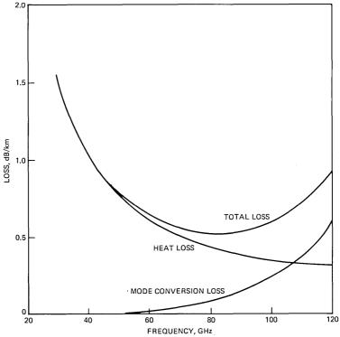
Fig. 3—Waveguide loss components.
