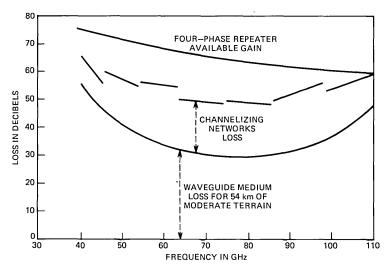
Fig. 1—Moderate-terrain transmission medium loss and projection of available gain.
