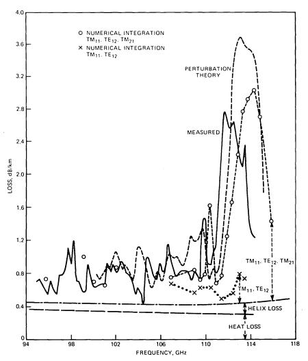
Fig. 9—Loss comparison for 720-m section.
