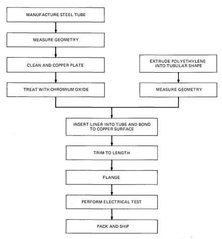
Fig. 4—Manufacturing process for dielectric-lined waveguide.
