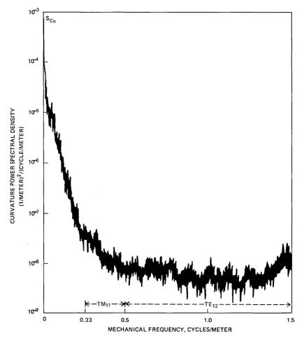
Fig. 5—Average field test horizontal curvature spectrum.
