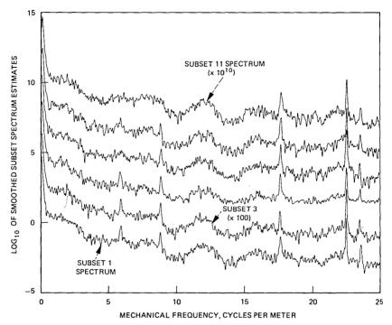
Fig. 6—Smoothed spectrum estimates from alternate subsets of mode filter section 6 vertical curvature. For plotting purposes the estimates have been offset by factors of 100.
