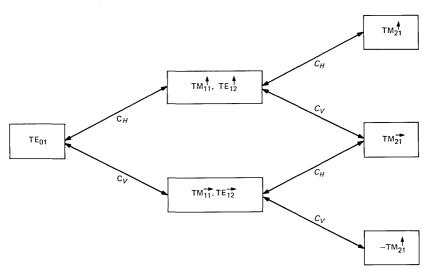
Fig. 2—Curvature coupling mechanisms.
