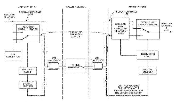
Fig. 4—Switching section—simplified block diagram.
