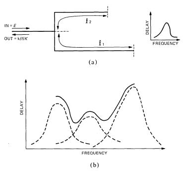
Fig. 4—(a) Delay reflection network. (b) Typical delay shape.
