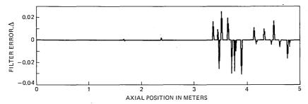
Fig. 14—The error,  $\Delta$ , between the original uncontaminated data (The contaminated data is shown in Fig. 13) and the sequence obtained by robust filtering using an extreme value influence function with  $u_0=4.5$ . Note the difference in scale between Figs. 13 and 14.
