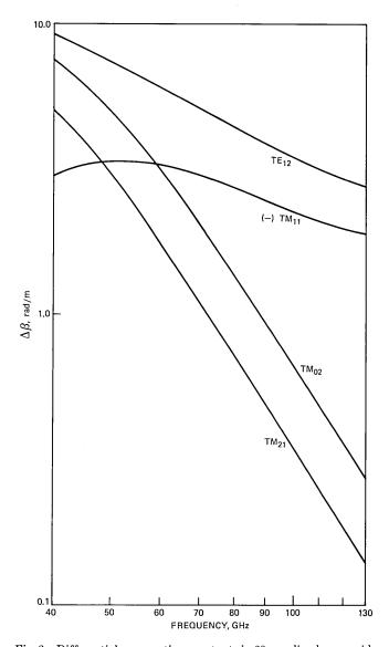
Fig. 3—Differential propagation constants in 60-mm lined waveguide.
