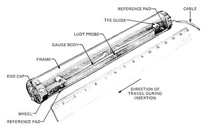
Fig. 7—Curvature gauge.
