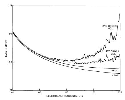
Fig. 10—WT4 field evaluation test estimated loss.
