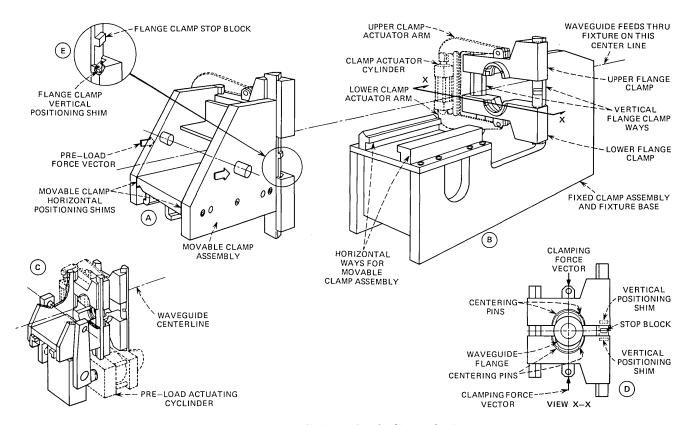
Fig. 5—The WSV aligning and preloading mechanisms.
