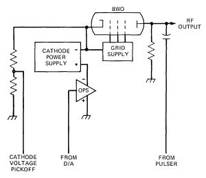
Fig. 4—BWO frequency-control circuit arrangement.
