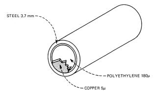
Fig. 4—Dielectric-lined waveguide.
