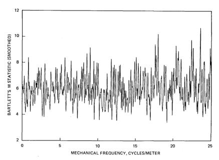
Fig. 9—Comparison of the subset spectrum estimates shown in Fig. 6 for homogeneity using Bartlett's *M* statistic as a function of frequency. For plotting and interpretative purposes the values shown here have been lightly smoothed.
