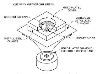
Fig. 2—IMPATT diode structure and package.
