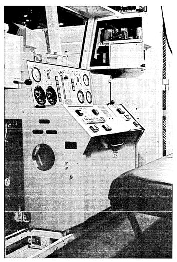
Fig. 4—The WSV aligning and splicing fixture.
