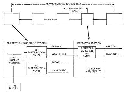
Fig. 1-WT4 nitrogen system maintenance area.
