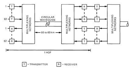
Fig. 1—Block diagram of a repeater hop.
