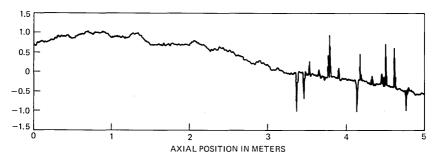
Fig. 13—Simulated waveguide curvature data with outliers. These data were generated using a 54th-order auto regression with a normal innovations sequence.
