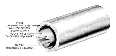
Fig. 2—Dielectric-lined waveguide configurations.
