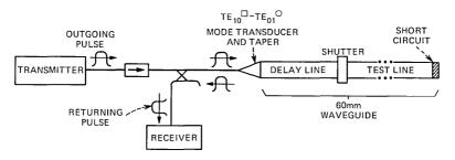
Fig. 1—Pulse reflection loss measurement arrangement.
