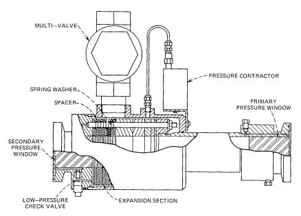
Fig. 6—Multifunction waveguide.
