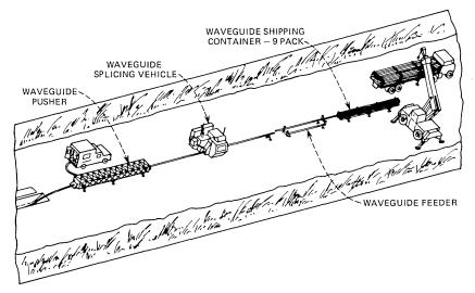
Fig. 2—Arrangement of field evaluation test equipment.
