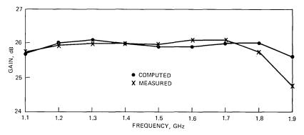
Fig. 8-Insertion gain vs. frequency.
