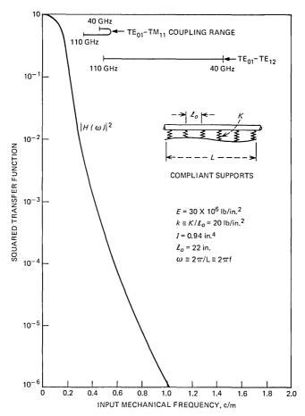
Fig. 7—Response of waveguide-support system.
