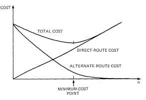
Fig. 2-Single-hour trunk-group sizing.
