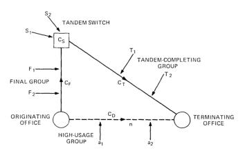
Fig. 6—Typical alternate-route configuration.
