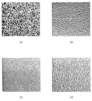
Fig. 12—Pictures of noise patterns for coefficients. (a) Picture of noise added to  $H_1$  on a flat background. (b) Picture of noise added to  $H_2$  on a flat background. (c) Picture of noise added to  $H_3$  on a flat background. (d) Picture of noise added to  $H_4$  on a flat background.
