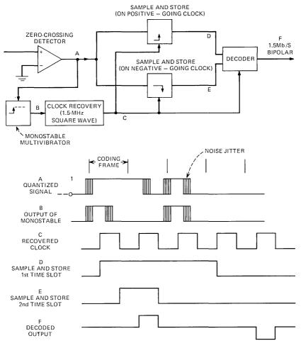
Fig. 3—Decoding process.
