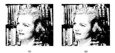
Fig. 5—Filtered test picture and *H*-noise added pictures. (a) Filtered test picture (1-MHz  $Picturephone^{\circ}$  filter). (b) Picture with noise added to  $H_1$ . (c) Picture with noise added to  $H_2$ . (d) Picture with noise added to  $H_4$ .
