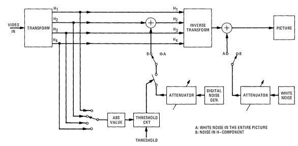
Fig. 7—Experimental setup. Noise is added to  ${\cal H}_2$  coefficient as a function of its magnitude.
