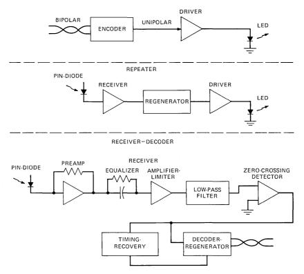
Fig. 2-Electronics of the optical-fiber link.
