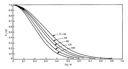
Fig. 5—First-order asymptotic approximation  $S_1(\eta)$  for the bore, with k = 0.5, plotted as a function of  $\eta$  for various values of the frequency parameter  $\chi$  and Poisson ratio  $\sigma = 0.16974$ .
