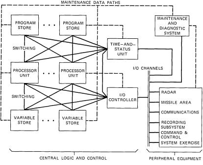
Fig. 1-Central Logic and Control unit.
