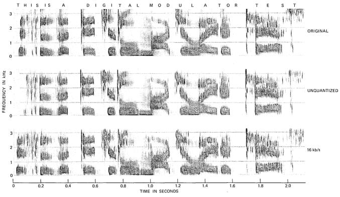
Fig. 9—Sound spectrograms comparing original, unquantized speech output and the 9.6-kb/s output from the sub-band coder.
