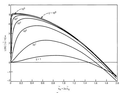
Fig. 16—Amplification factor vs  $\tilde{k}_0$  for  $\alpha=0.001$ , g=0.1, and  $1\leq\xi\leq10^6$  (modification of Tomotika's analysis for quenched base state).
