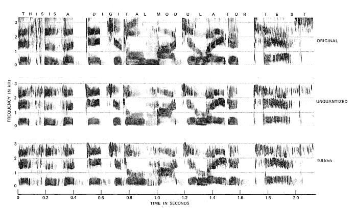
Fig. 8—Sound spectrograms comparing original, unquantized speech output and the 16-kb/s output from the sub-band coder.
