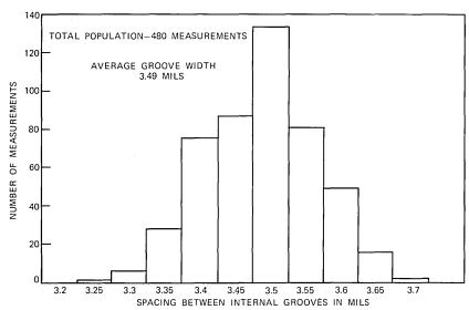
Fig. 3—Histogram of spacing between the internal grooves of molded polycarbonate substrate.
