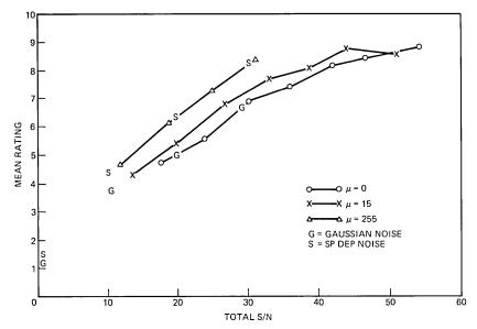
Fig. 8—Mean ratings of unclipped speech for each companding law and the added noise conditions as a function of the total s/n.
