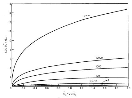
Fig. 15—Amplification factor vs  $\tilde{k}_0$  for  $\xi \to \infty$  (Tomotika's model with constant viscosity and surface tension).
