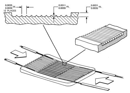
Fig. 1—Precision-molded substrate for  $12 \times 12$  optical-fiber splice connector.
