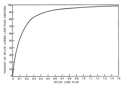
Fig. 7—Derived cumulative distribution of total splice loss data.
