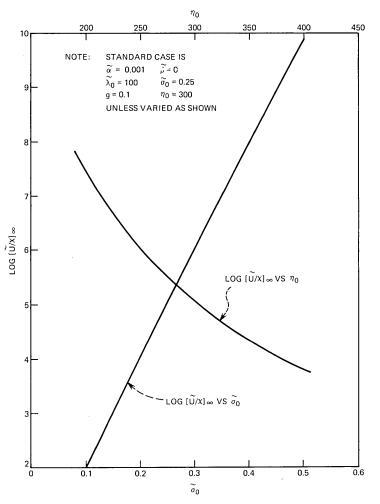
Fig. 14—Amplification factor vs  $\eta_0$  and  $\tilde{\sigma}_0$ .
