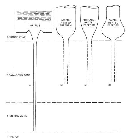
Fig. 1—Fiber-drawing methods.
