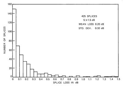
Fig. 6—Histogram of total splice loss data.
