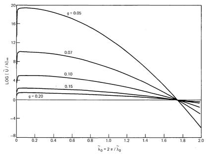
Fig. 17—Amplification factor vs  $\tilde{k}_0$  for  $\tilde{\alpha}=0.001$ ,  $\xi=10^6$ , and  $0.005 \le g \le 0.20$  (modification of Tomotika's analysis for quenched base state).
