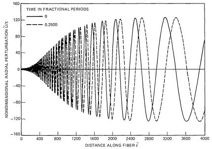
Fig. 11—Plot of deflected surface shapes for  $\tilde{\lambda}_0 = 15.7$ .
