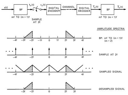
Fig. 7—Integer-band sampling technique for digital encoding of speech sub-bands.
