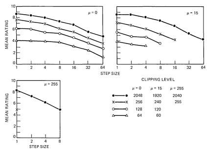
Fig. 6—Mean rating across listeners, talkers, and bandwidth at each clipping level as a function of step size for each companding law.
