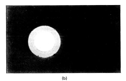
Fig. 10(a)—Optical ribbon with prepared fiber ends. (b) Typical fiber end.
