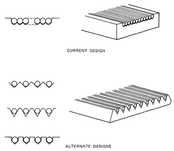
Fig. 8-Alternate groove depths.
