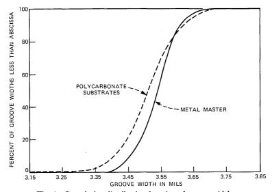
Fig. 4—Cumulative distribution function of groove widths.
