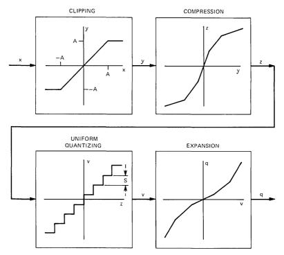
Fig. 3—Four processes included in quantization.
