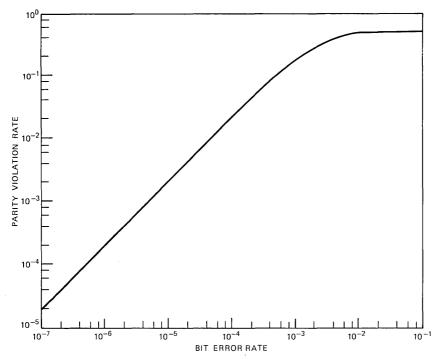
Fig. 1-Parity-violation rate vs bit-error rate.
