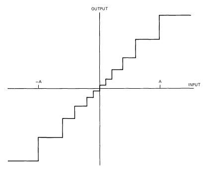
Fig. 2—Input/output diagram of a quantizer.
