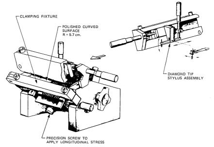
Fig. 9—Fiber ribbon cutting tool.
