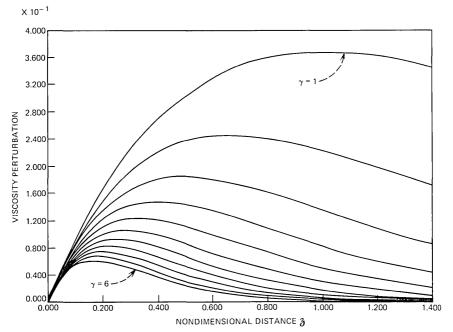
Fig. 4—Profiles of the viscosity perturbation,  $\nu/\nu_0 = \partial e^{-\gamma \delta}$ .
