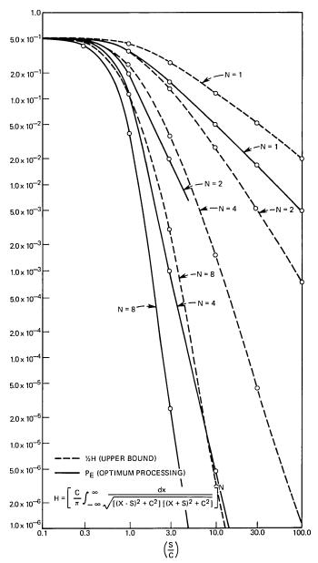
Fig. 12—Log likelihood probability of error and Hellinger integral upper bound for Cauchy ( $\alpha=1,\,\beta=0$ ) samples vs (s/c).
