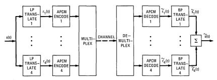
Fig. 3—Four-band encoder using low-pass translation and APCM encoding in each band.
